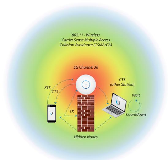
In summary, 802.11 wireless networks are based on listen first, then talk design. "Wi-Fi" radios like UniFi Access Points are half-duplex, meaning they can either transmit or receive, but neither communicate simultaneously. Compared to switches, wireless radios feature a single collision domain shared among stations competing for channel usage.
