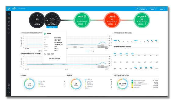
The UniFi dashboard summarizes the most important statistics about traffic collected by UniFi devices and reported back to the UniFi controller. The Deep Packet Inspection engine is a free, powerful function that can be enabled for any UniFi site with a UniFi Security Gateway. To enable the DPI function, visit the Site settings page in your UniFi Controller.
