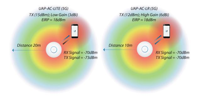
The antenna gain diagrams represent a three-dimensional area over which wireless signals propagate. Indoor as well as outdoor UniFi access points feature 'omnidirectional' antennas that produce a radiation pattern similar to a 'donut' shape.
