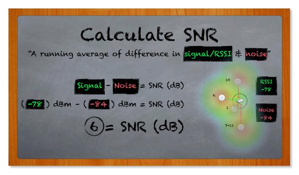
UniFi relates SNR as a percentage value to help new WLAN admins troubleshoot the connected stations in their network. Just like SNR, which is a dynamically changing value, the Signal % of a client device may increase or decrease accordingly and in real-time. To derive the SNR reported by the Signal % value, the following formula may be used:
