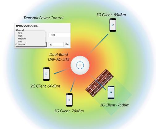
The purpose of any access point is to provide wireless coverage to clients over a given area known as a cell. As a WLAN station moves away from the AP, its receive signal gradually weakens. This also occurs as obstacles prevent direct line-of-sight between AP and station. As signals decrease, wireless performance drops before eventually, the station becomes disconnected from the AP. This is due to the Free Space Path Loss (FSPL) relationship as mentioned previously.
