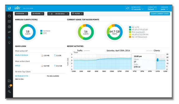
Enterprise networks often require that statistics be gathered to monitor traffic and establish controls on network activity. UniFi provides flexibility in monitoring wireless traffic and presents the data in an intuitive manner during user-defined intervals. The Controller makes setting user controls simple and straightforward. Among the data collected and displayed on the *Statistics* tab, UniFi tracks:
