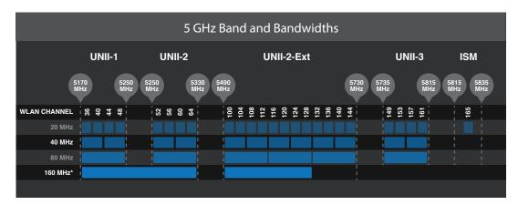
Compared to the 2.4 GHz spectrum, 5 GHz offers much more flexibility for wireless operators due to greater availability of spectrum and relaxed transmission power requirements. Although the 2.4 GHz band only allows for 3 reuse channels without overlap (1, 6 and 11), the 5 GHz band allows for as many as 24, depending on region (36, 40, 149, 153, etc.). Given the abundance of available channels and short-range propagation characteristics, high-density WLANs benefit greatly from the 5 GHz band.
