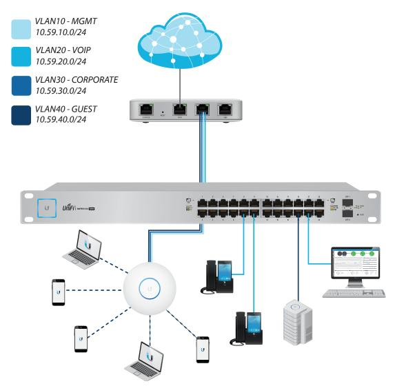
Scalability and security are two important objectives when deploying an enterprise network. Through VLAN (virtual LAN) technology, networks can achieve both without great costs in time or resources. Fortunately, UniFi supports 802.1Q, an industry standard that supports VLAN information in packet (frame) headers.
