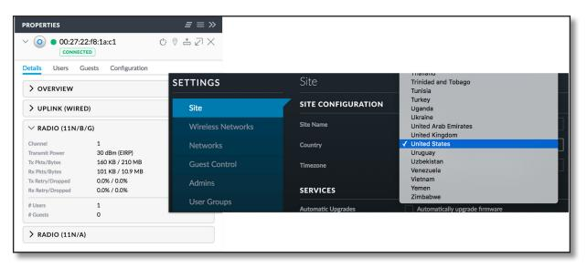
Check the *Properties* settings for your UniFi AP to see its EIRP level (in dBm). To determine its actual Transmit (TX) Power level (in dBm), subtract its Antenna Gain (in dBi) from its EIRP (in dBm). The Transmit Power for the UAP-AC-LITE pictured in the previous image is 27 dBm, since the EIRP = 30 dBm and its Antenna Gain = 3 dBi.
