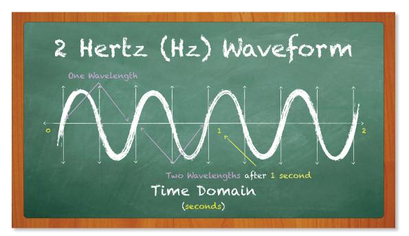
Frequency is measured in Hertz (Hz), which individually represents one period, wavelength, or wave cycle. As a waveform travels from one point to another, it undergoes signal loss due to a phenomenon known as Free Space Path Loss (FSPL). However, lower frequencies (ex. 2.4 GHz) have much longer wavelengths and can propagate further than higher frequencies (ex. 5 GHz).
