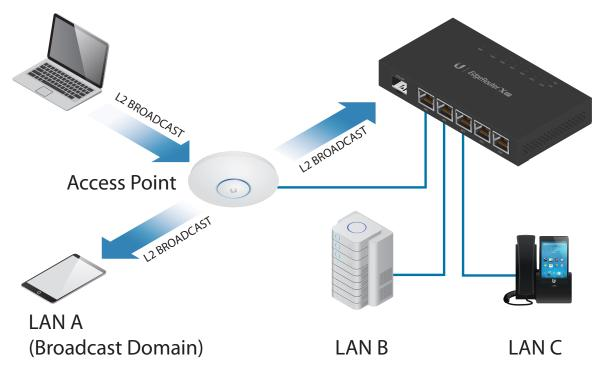
The following image demonstrates how **LAN segmentation** can limit the severity of broadcast storms in the network environment by replacing a switch with a layer-3 router.
