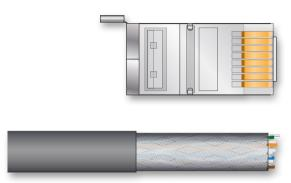
Carefully cut and remove the braided cable shielding covering the drain wire and foil shield.
