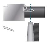
**TC-GND Users** - If you are using TC-GND TOUGHCable Connectors, then secure the end of the ground wire to a grounding point, such as the tower ground system or a metal mounting bracket.
