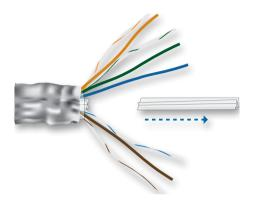
Place the wires in order as shown below (and as detailed in the Cable Wiring Specification T568B on page 8). Ensure the wires are as straight and compact as possible.
