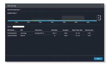
**Scanned Frequencies** Displays the scanned frequencies list. In *Station PTP* or *Station PTMP* mode, you can edit this list; for details, see <u>"Frequency List, MHz" on page 15</u>.
