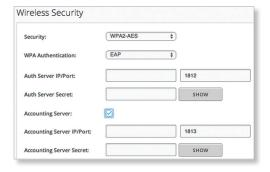
**Auth Server IP/Port** In the first field, enter the IP address of the RADIUS authentication server. RADIUS is a networking protocol providing centralized Authentication, Authorization, and Accounting (AAA) management for computers to connect to and use a network service.
