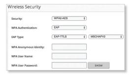
**EAP Type** Select the authentication protocol (**EAP-TTLS** or **EAP-PEAP**) and the inner authentication protocol (**MSCHAPV2**).
