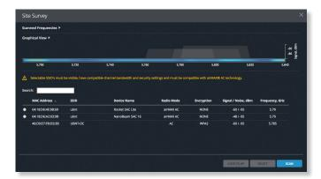
The Site Survey tool will search all supported channels for available wireless networks in range and let you select one for association. The tool has incremental scan functionality for more dynamic results. If the selected network uses encryption, you'll need to configure the Wireless Security settings (refer to "Wireless Security" on page 16).
