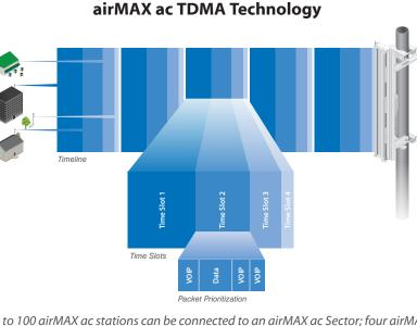
Up to 100 airMAX ac stations can be connected to an airMAX ac Sector; four airMAX ac stations are shown to illustrate the general concept.
