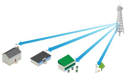
The IsoStation<sup>™</sup> 5AC is used as a CPE device for each client in an airMAX PtMP (Point-to-MultiPoint) network.
