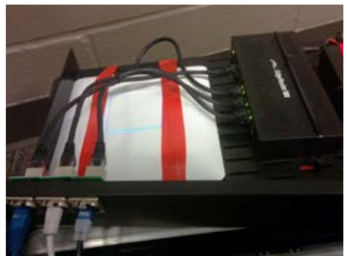
UniFi AP AC connected to an EdgeRouter Lite
