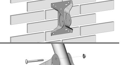
Install the pole to the base using pivot bolt
