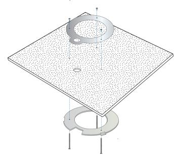
6. Feed the Ethernet cable through the hole and then align the UniFi AP with the notches on the *Wall-Mount Bracket*.
