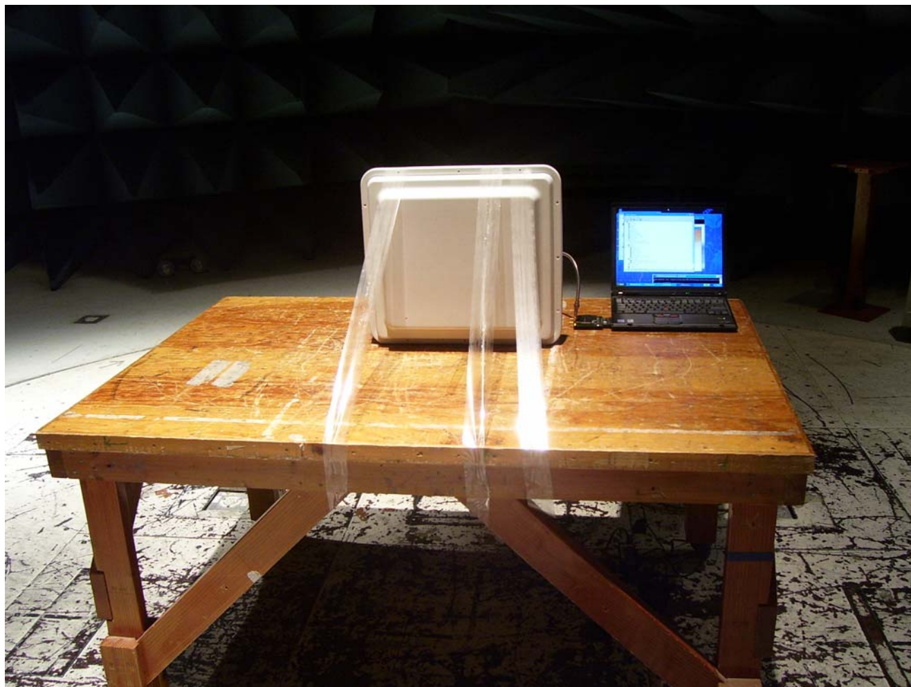
Photograph 5. Test Equipment and setup for various Radiated Measurements
