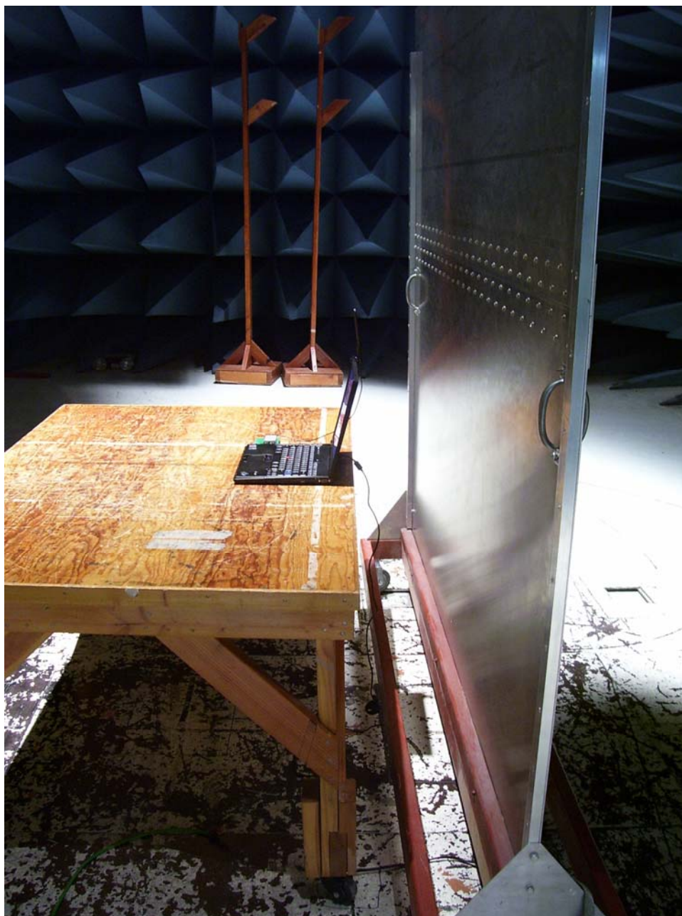
Photograph 2. Conducted Emissions Test Setup
