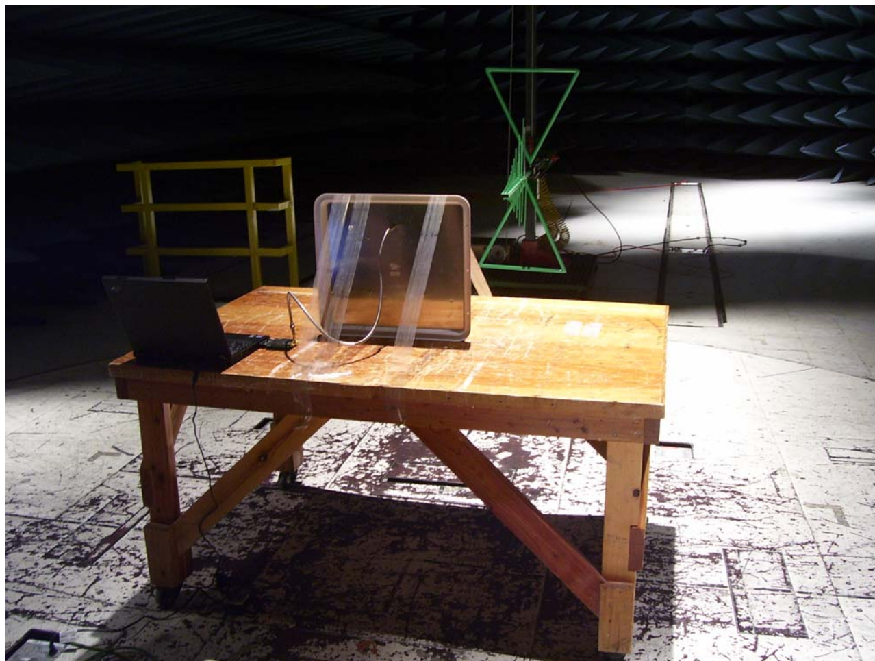
Photograph 4. Radiated Emission Test Setup 30 MHz - 1 GHz
