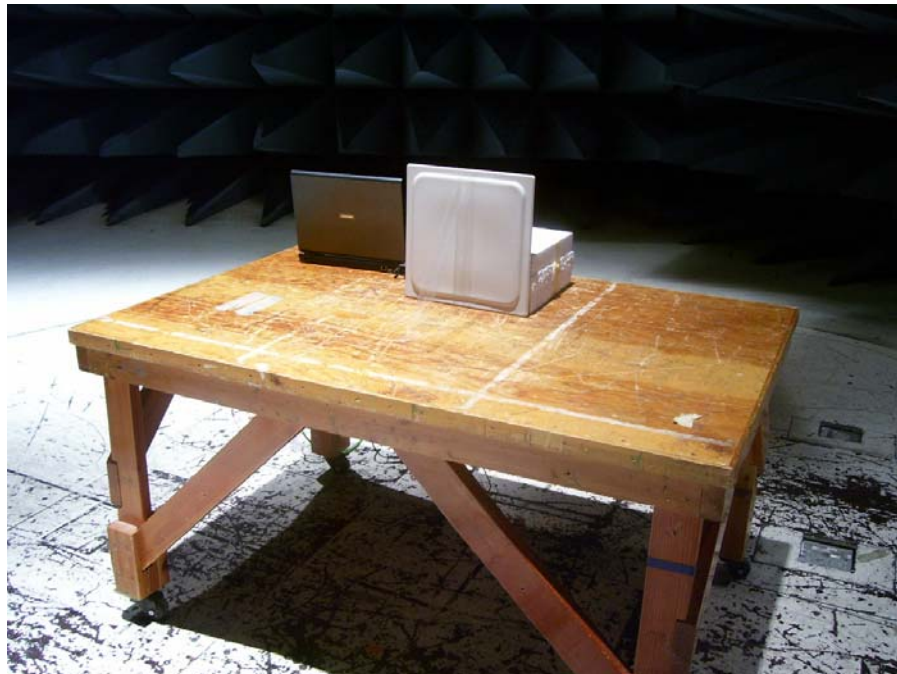
Photograph 5. Test Equipment and setup for various Radiated Measurements Panel Antenna
