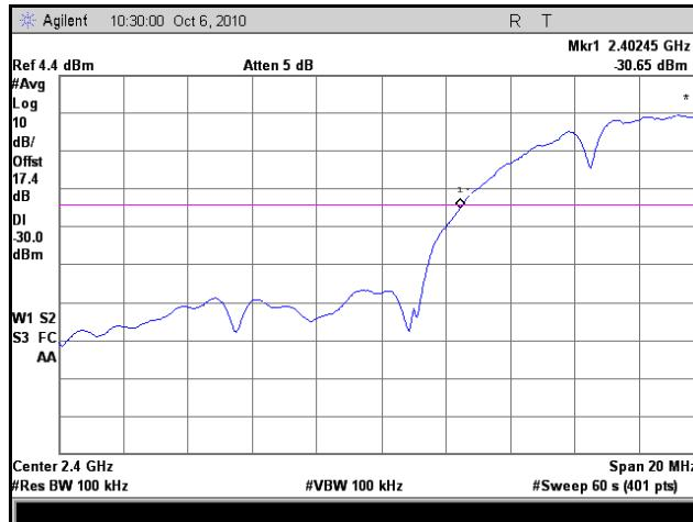
Plot 21. Frequency Range, Low Channel, 802.11b, Normal Temperature, Normal Voltage
