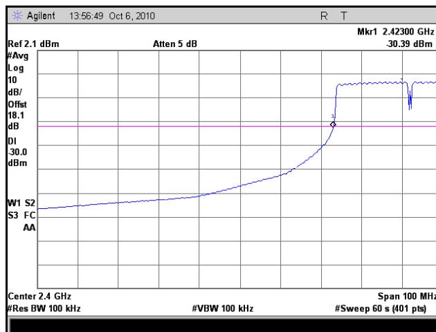
Plot 53. Frequency Range, Low Channel, 802.11n 40 MHz, Maximum Temperature, Minimum Voltage
