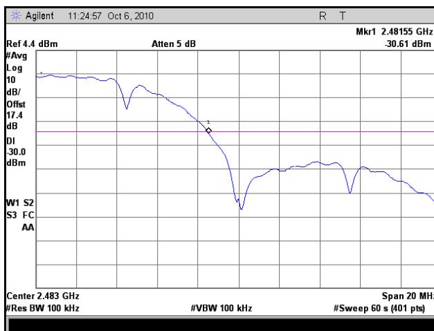
Plot 28. Frequency Range, High Channel, 802.11b, Maximum Temperature, Minimum Voltage
