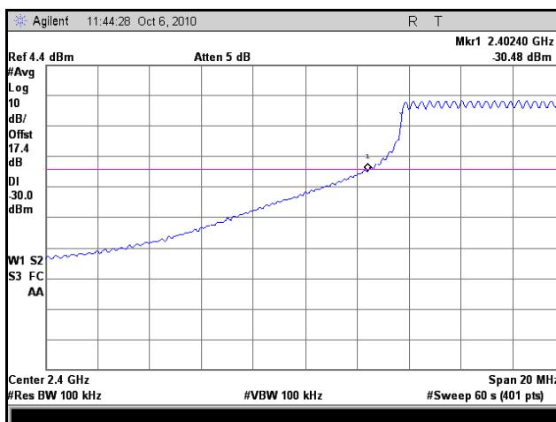
Plot 32. Frequency Range, Low Channel, 802.11g, Maximum Temperature, Maximum Voltage
