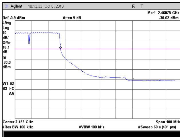
**Plot 56. Frequency Range, High Channel, 802.11n 40 MHz, Normal Temperature, Normal Voltage**
