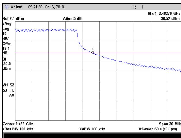
**Plot 49. Frequency Range, High Channel, 802.11n 20 MHz, Minimum Temperature, Maximum Voltage**
