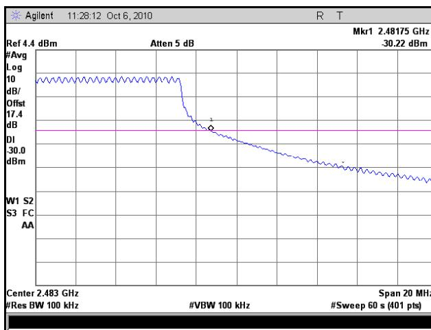
Plot 38. Frequency Range, High Channel, 802.11g, Maximum Temperature, Minimum Voltage
