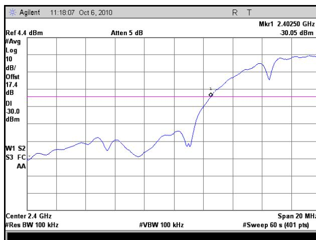
Plot 23. Frequency Range, Low Channel, 802.11b, Maximum Temperature, Minimum Voltage
