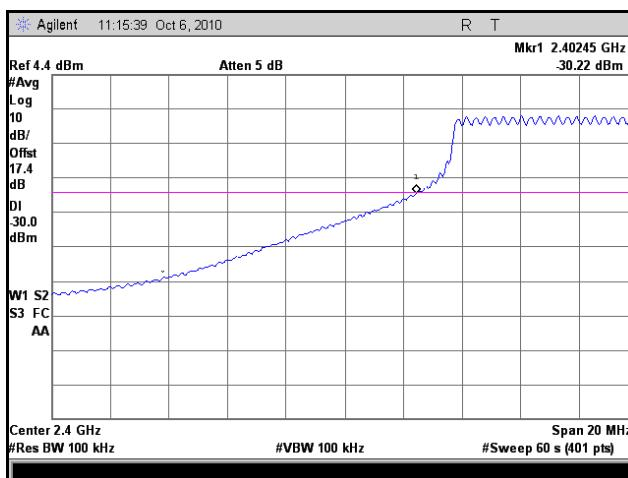
Plot 33. Frequency Range, Low Channel, 802.11g, Maximum Temperature, Minimum Voltage
