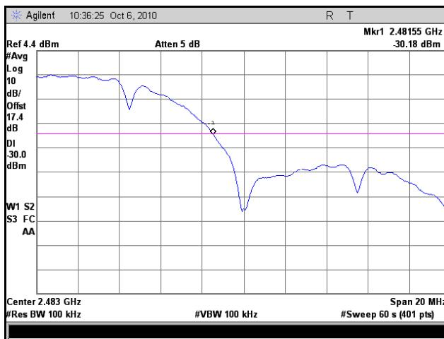
**Plot 26. Frequency Range, High Channel, 802.11b, Normal Temperature, Normal Voltage**
