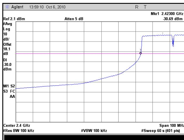
Plot 52. Frequency Range, Low Channel, 802.11n 40 MHz, Maximum Temperature, Maximum Voltage
