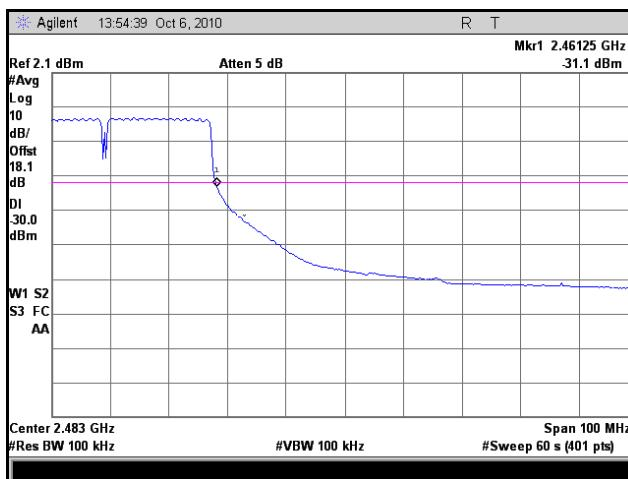
**Plot 58. Frequency Range, High Channel, 802.11n 40 MHz, Maximum Temperature, Minimum Voltage**
