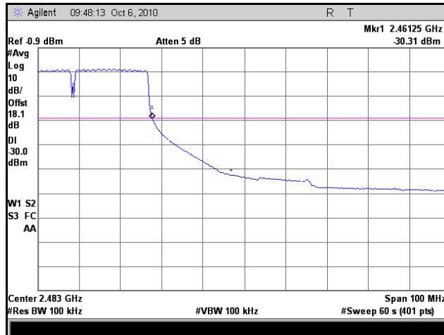
**Plot 60. Frequency Range, High Channel, 802.11n 40 MHz, Minimum Temperature, Minimum Voltage**
