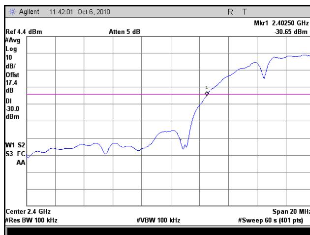
Plot 22. Frequency Range, Low Channel, 802.11b, Maximum Temperature, Maximum Voltage
