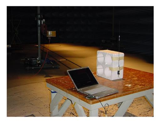
Photograph 4. Test Equipment and setup for Radiated Harmonic Measurements
