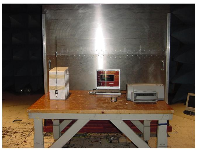
Photograph 1. Conducted Emissions Test Setup
