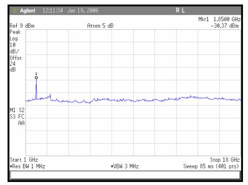
Plot 4. 802.11/b - Low Channel Conducted Emissions 1-18GHz
