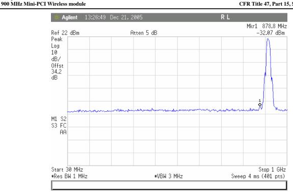
Plot 5. 802.11/b - High Channel Conducted Emissions 30MHz-1GHz
