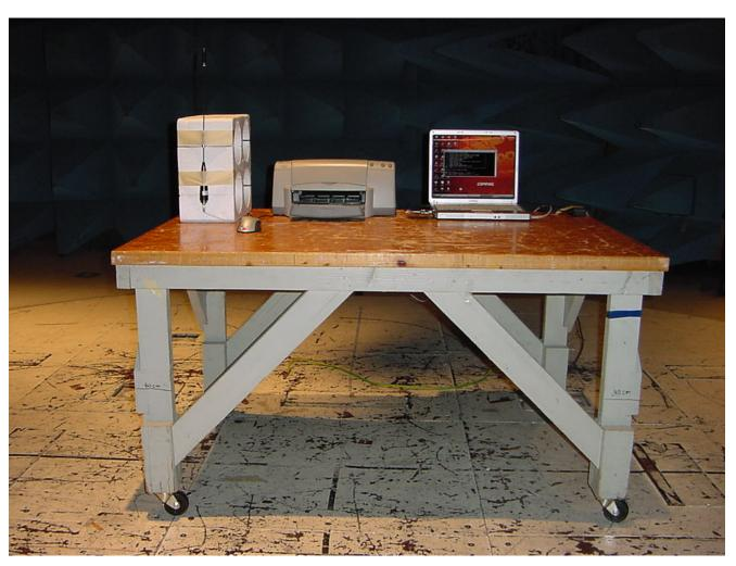
Photograph 2. Radiated Emission Limits Test Setup
