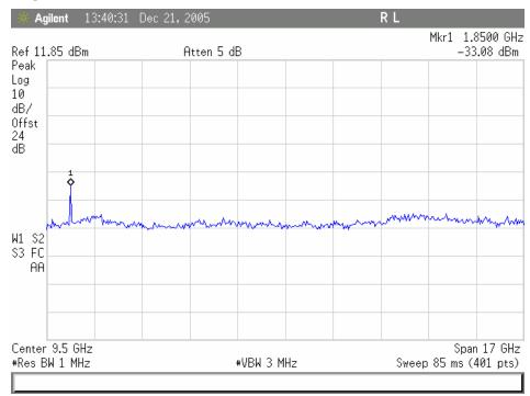
Plot 6. 802.11/b - High Channel Conducted Emissions 1-18GHz
