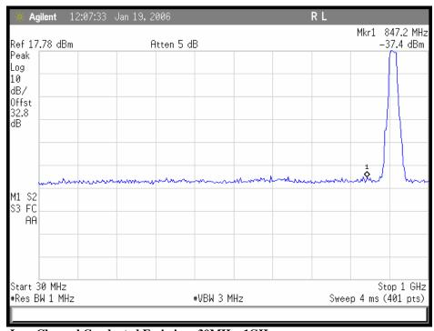
Plot 7. 802.11/g – Low Channel Conducted Emissions 30MHz- 1GHz
