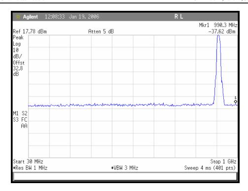
Plot 3. 802.11/b - Low Channel Conducted Emissions 30MHz - 1GHz
