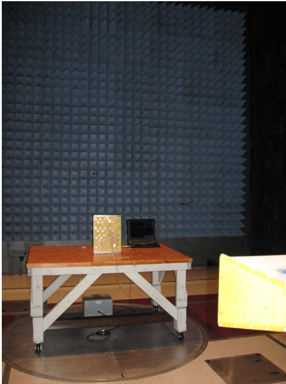
Photograph 6. Test Equipment and setup for various Radiated Measurements – 5.8GHz Panel Antenna
