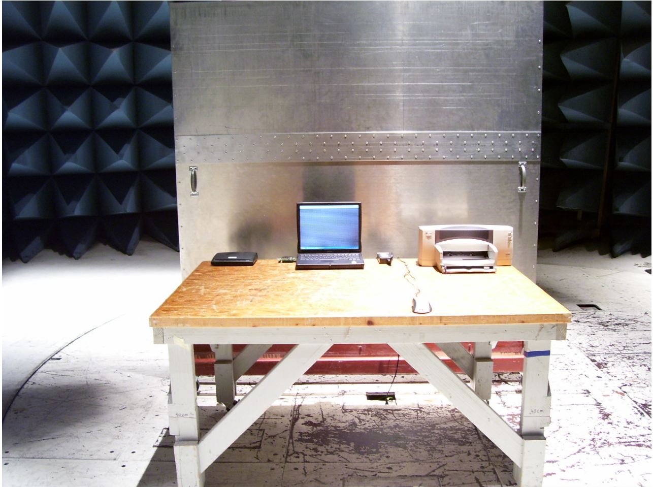
Photograph 2. Conducted Emissions Test Setup
