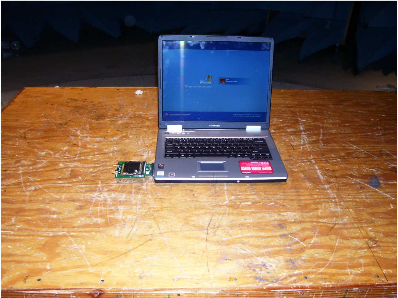
Photograph 4. Radiated Emission Spurious Test Setup
