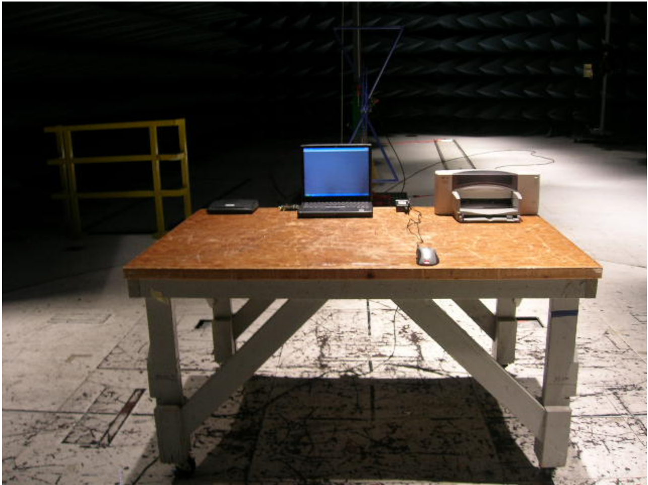
Photograph 3. Radiated Emission Limits Test Setup
