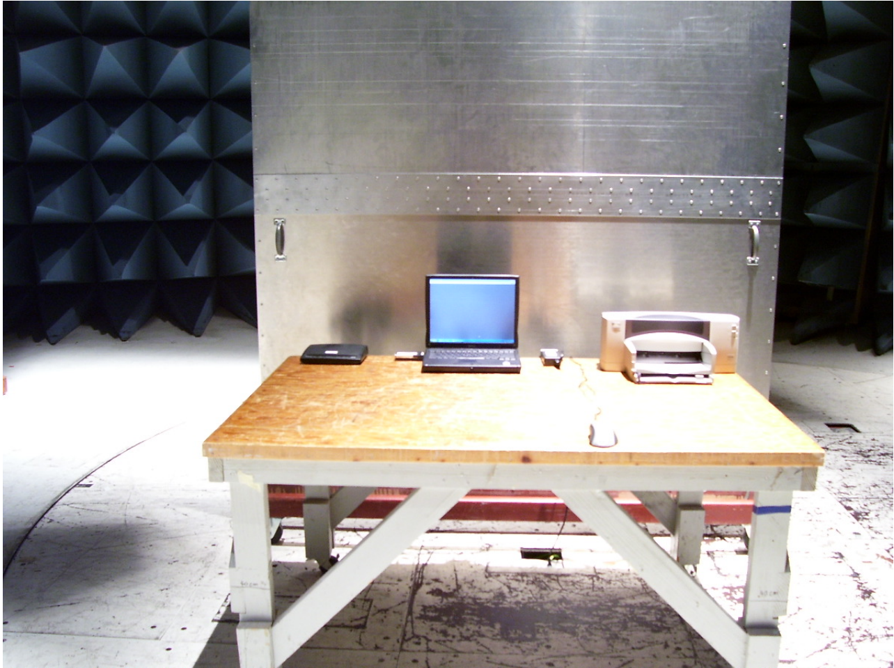
Photograph 2. Conducted Emissions Test Setup
