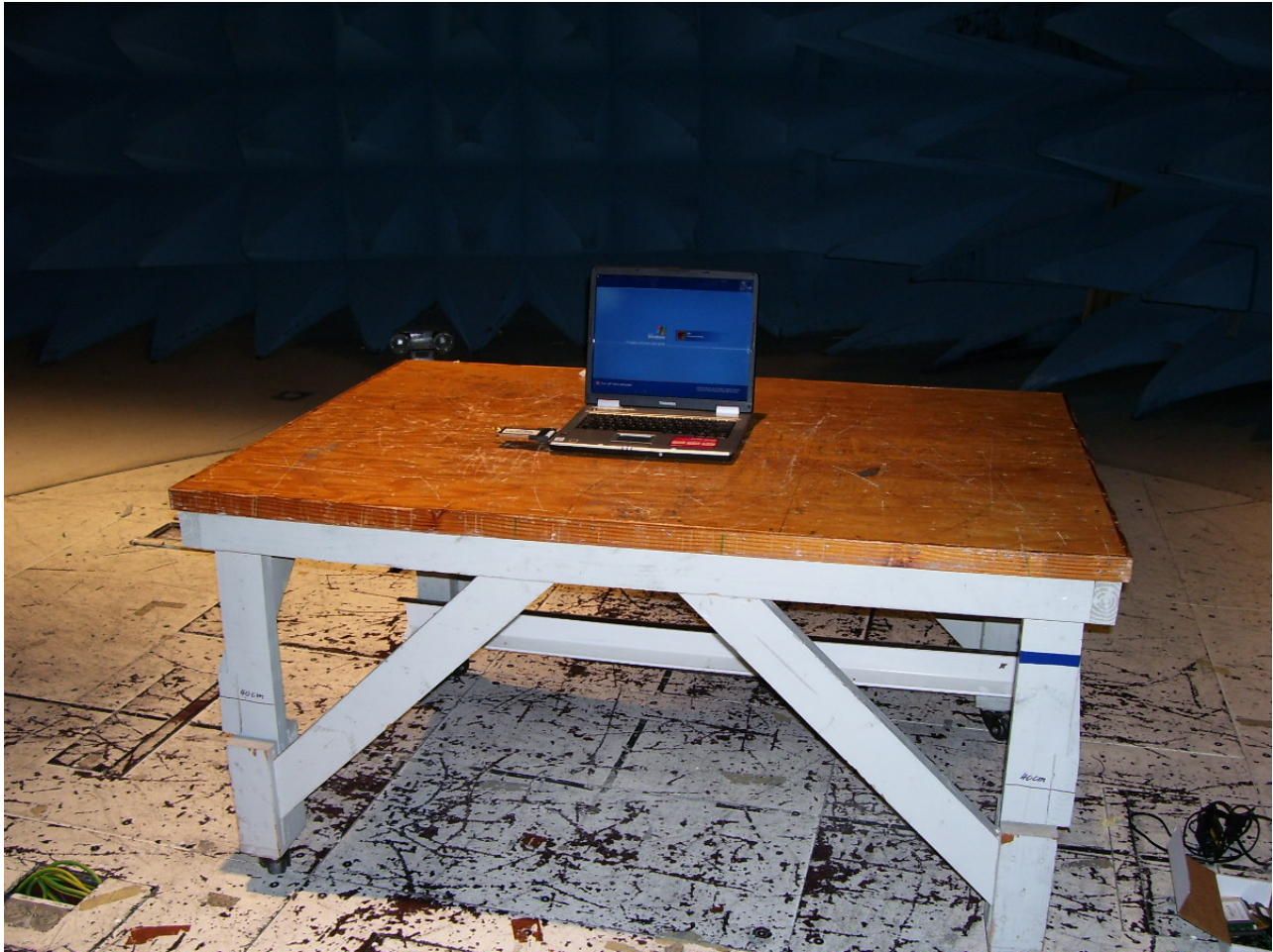
Photograph 4. Radiated Emission Spurious Test Setup
