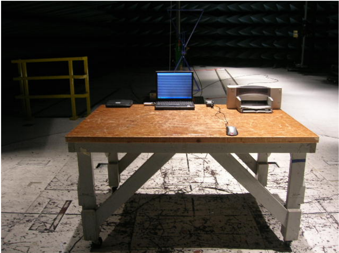
Photograph 3. Radiated Emission Limits Test Setup
