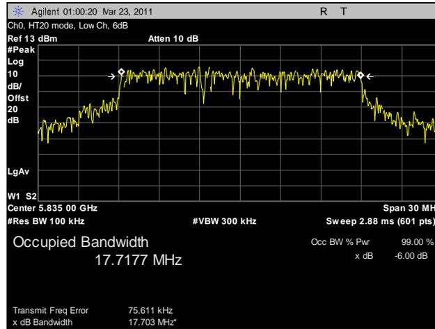
Plot 6. 6 dB Occupied Bandwidth, Low Channel, HT20, CH0
