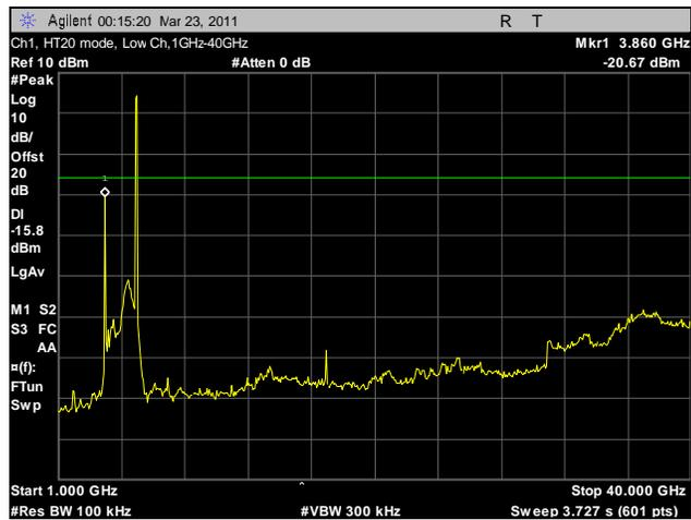
Plot 186. Conducted Spurious Emissions, Low Channel, HT20, 1 GHz – 40 GHz, CH1
