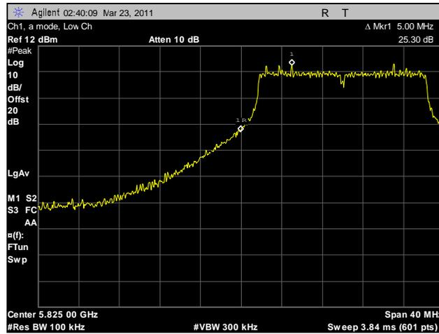
Plot 201. Conducted Spurious Emissions, Low Channel, a Mode, CH1, 20 dBc
