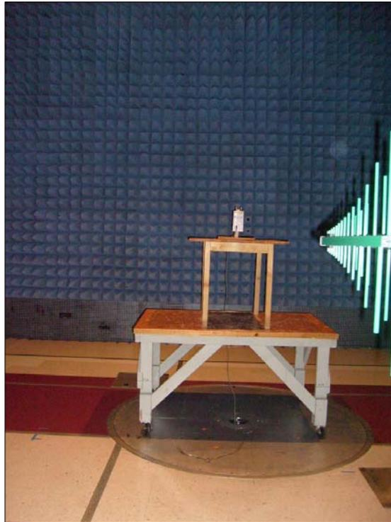
**Photograph 1. Radiated Emissions, Test Setup, 30 MHz – 1 GHz**
