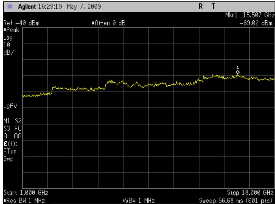
Plot 159. Receiver Mode Spurious Emission, 1 GHz - 18 GHz, , All Ports
