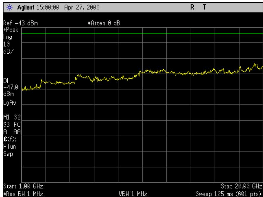
**Plot 155. Receiver Mode Spurious Emission 1 GHz - 26.5 GHz, Port 2, HT20**
