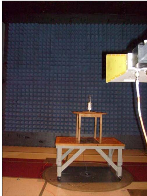
**Photograph 5. Radiated Emissions, Test Setup, 1 GHz – 18 GHz, n**
