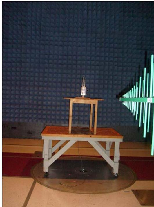
**Photograph 4. Radiated Emissions, Test Setup, 30 MHz – 1 GHz, n**
