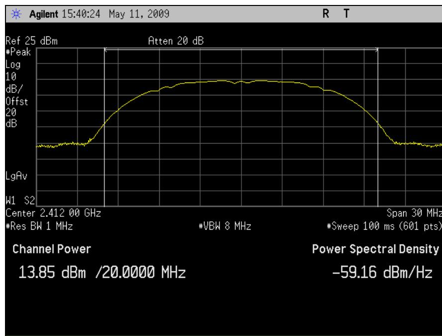
Plot 26. Output Power – Low Channel 802.11b Mode, Port 1 (16dBi Sector Antenna)
