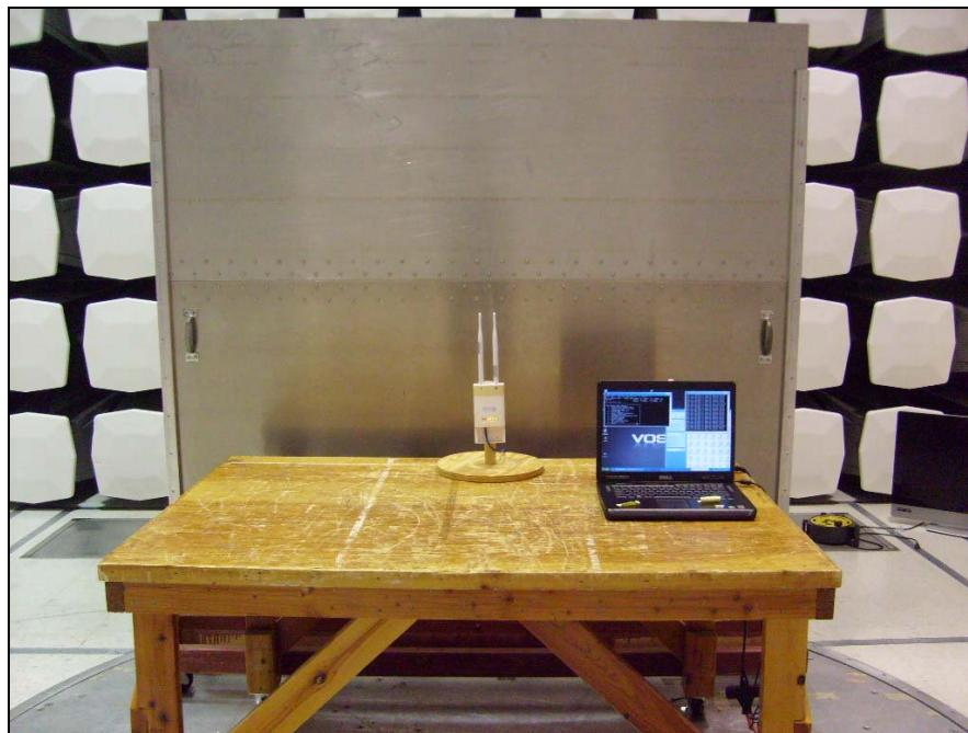
**Photograph 5. Conducted Emissions Test Setup**
