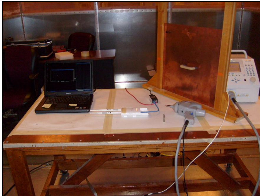
Photograph 6. Electrostatic Discharge, Test Setup
