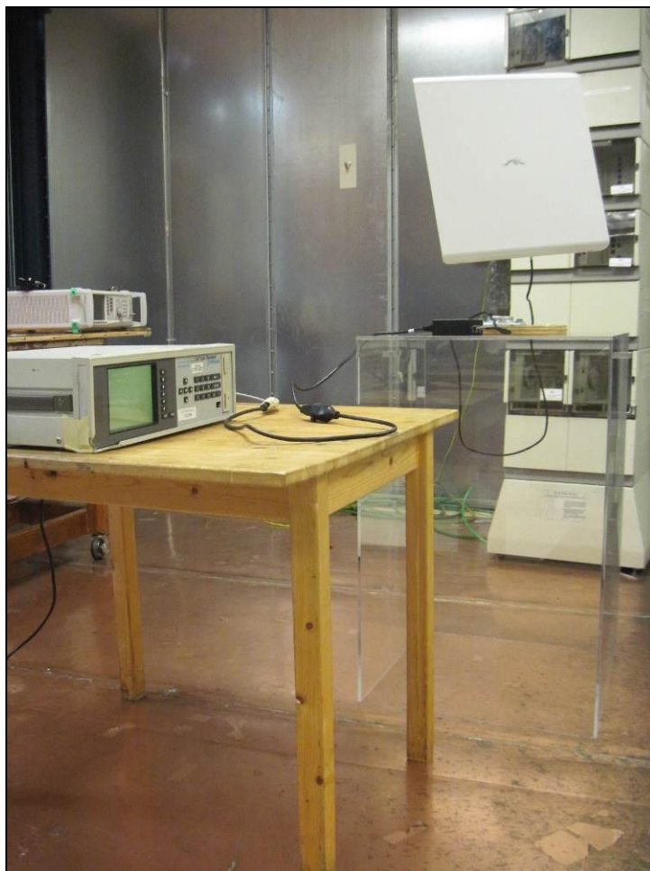
Photograph 4. Voltage Fluctuations (Flicker), Test Setup
