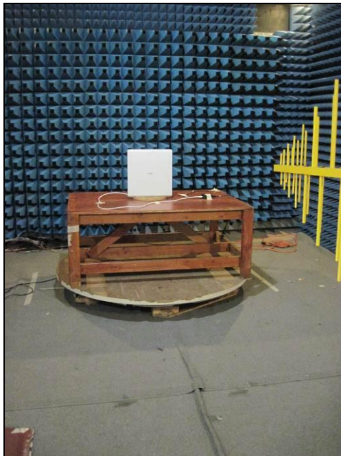
Photograph 6. Radiated Immunity, Test Setup, 80 MHz – 1 GHz
