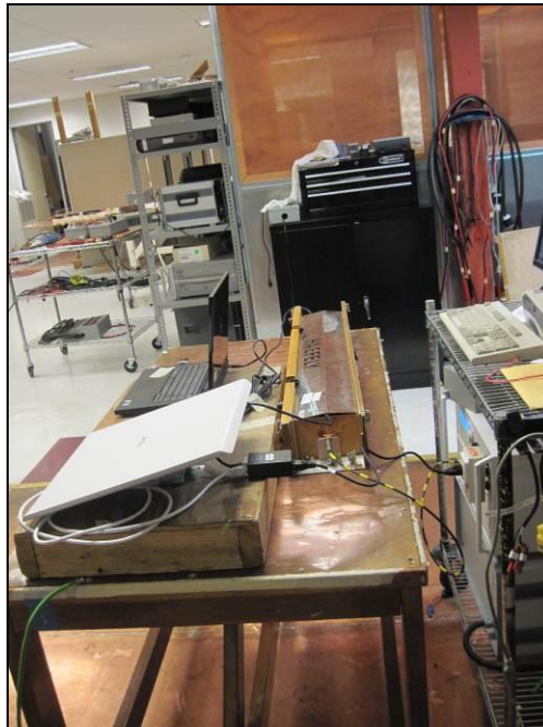
Photograph 12. Fast Transient, Common Mode, Test Setup, I/O Cables
