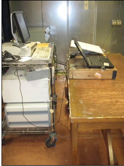
Photograph 11. Fast Transient, Common Mode, Test Setup, AC Mode
