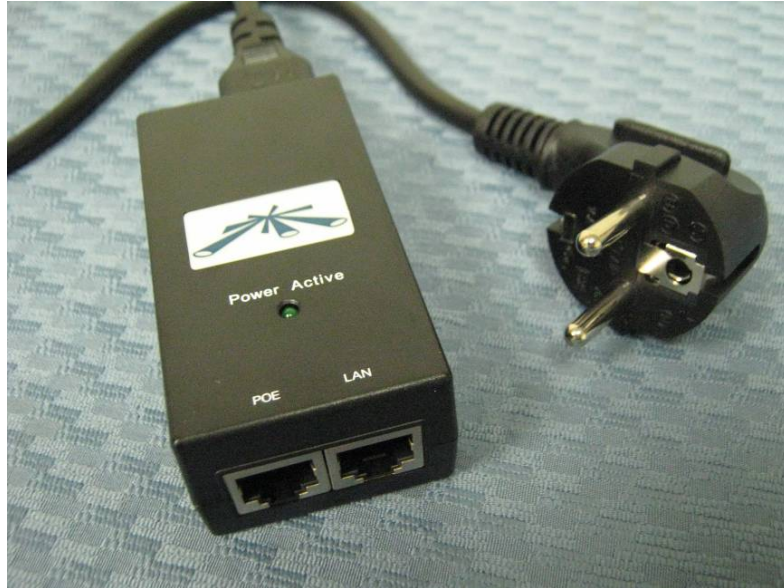
Figure 5: Listed AC/DC LPS Power Supply Adaptor
