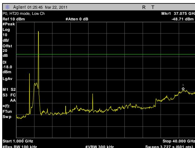
**Plot 117.** Conducted Spurious Emissions, Low Channel, HT20, 1 GHz – 40 GHz, P0
