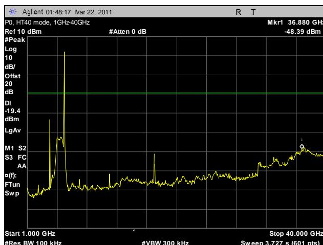
Plot 123. Conducted Spurious Emissions, HT40, 1 GHz – 40 GHz, P0
