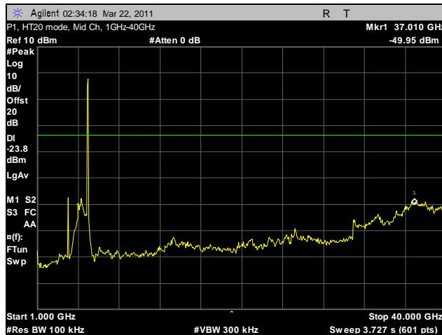
Plot 133. Conducted Spurious Emissions, Mid Channel, HT20, 1 GHz – 40 GHz, P1
