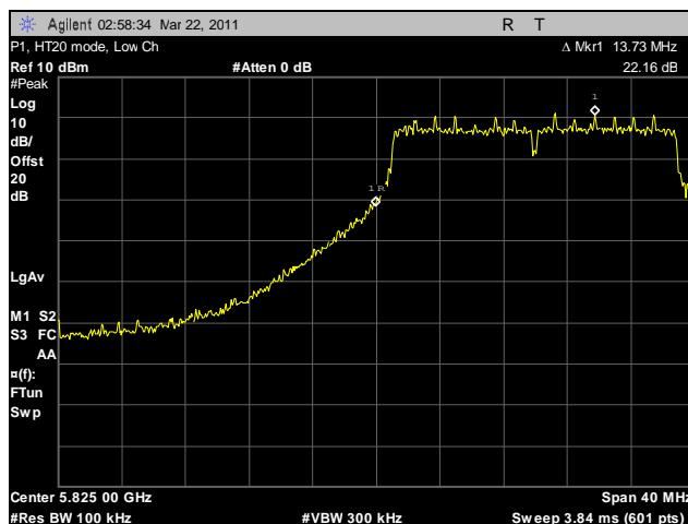
Plot 148. Conducted Spurious Emissions, Low Channel, HT20, P1, 20 dBc
