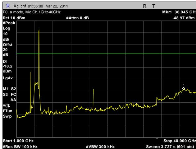
**Plot 107. Conducted Spurious Emissions, Mid Channel, a Mode, 1 GHz – 40 GHz, P0**
