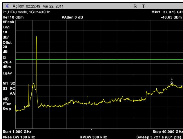
Plot 137. Conducted Spurious Emissions, HT40, 1 GHz – 40 GHz, P1
