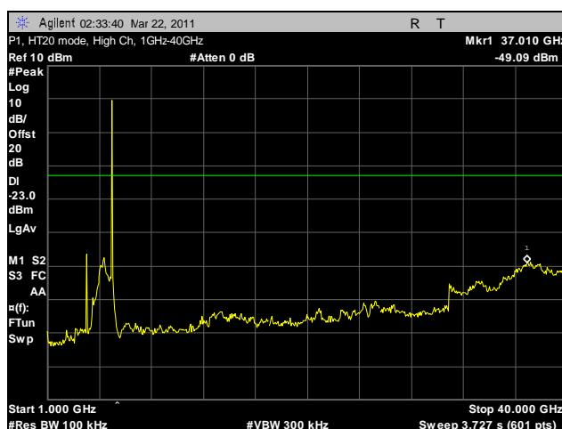
Plot 135. Conducted Spurious Emissions, High Channel, HT20, 1 GHz – 40 GHz, P1
