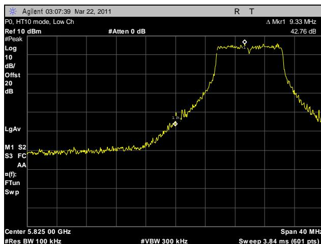
Plot 140. Conducted Spurious Emissions, Low Channel, HT10, P0, 20 dBc
