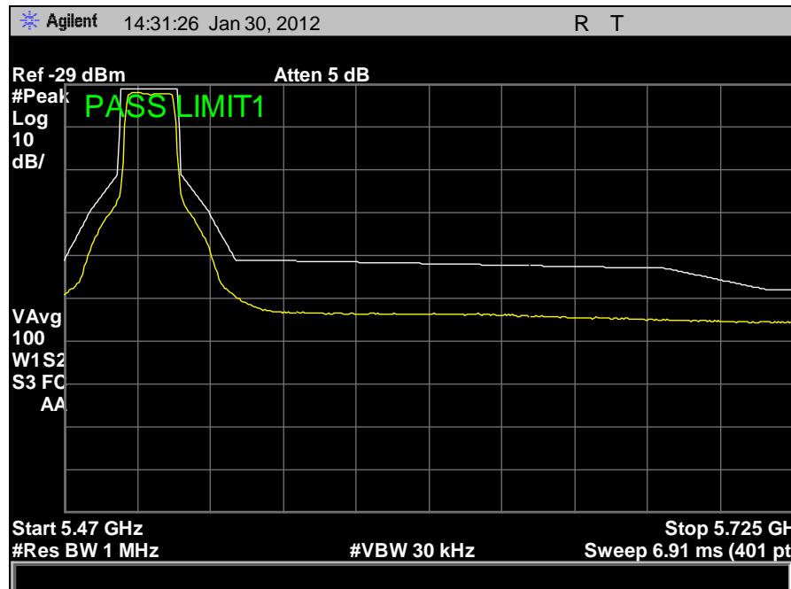
Plot 106. Conducted In Band Spurious Emission, Wide Span, 5500 MHz, 802.11a 20 MHz
