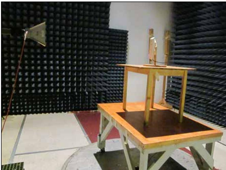
Photograph 4. Radiated Emissions, Test Setup, 1 GHz – 18 GHz
