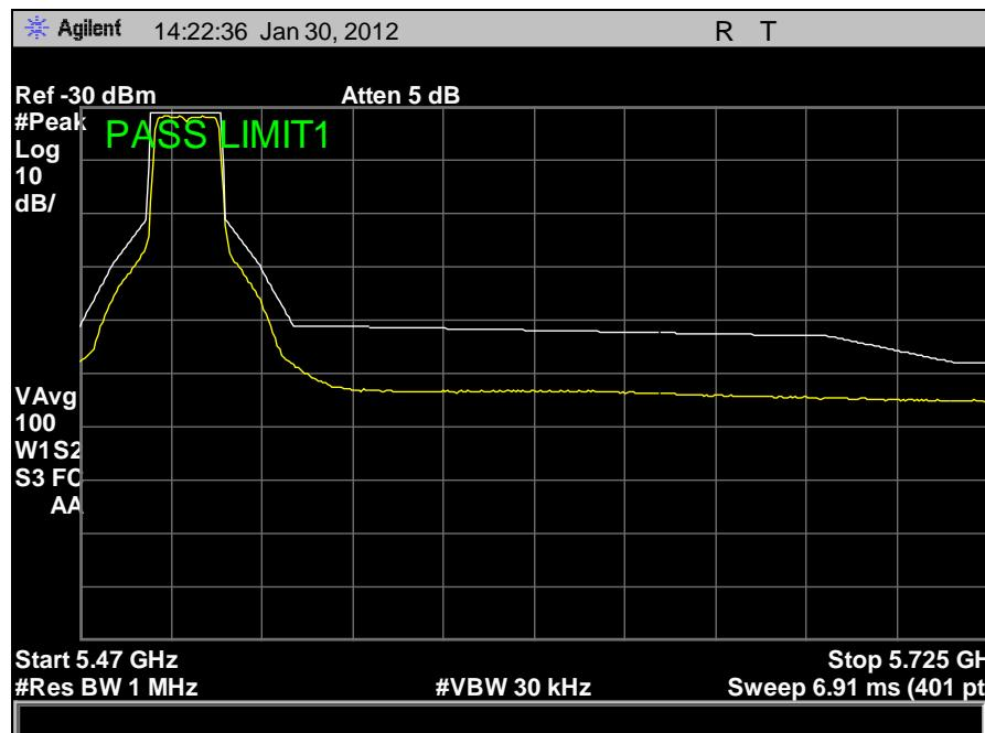
Plot 114. Conducted In Band Spurious Emission, Wide Span, 5500 MHz, 802.11n 20 MHz
