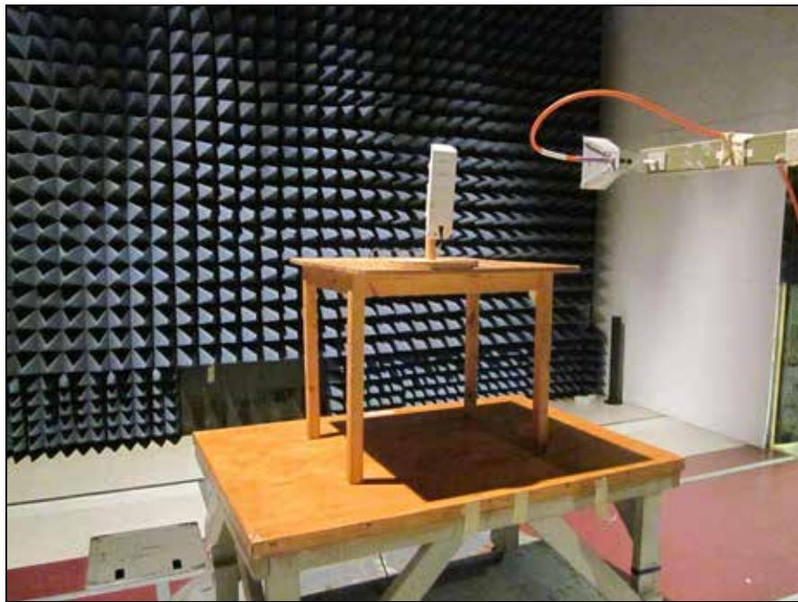
**Photograph 5. Radiated Emissions, Test Setup, 1 GHz – 26.5 GHz**
