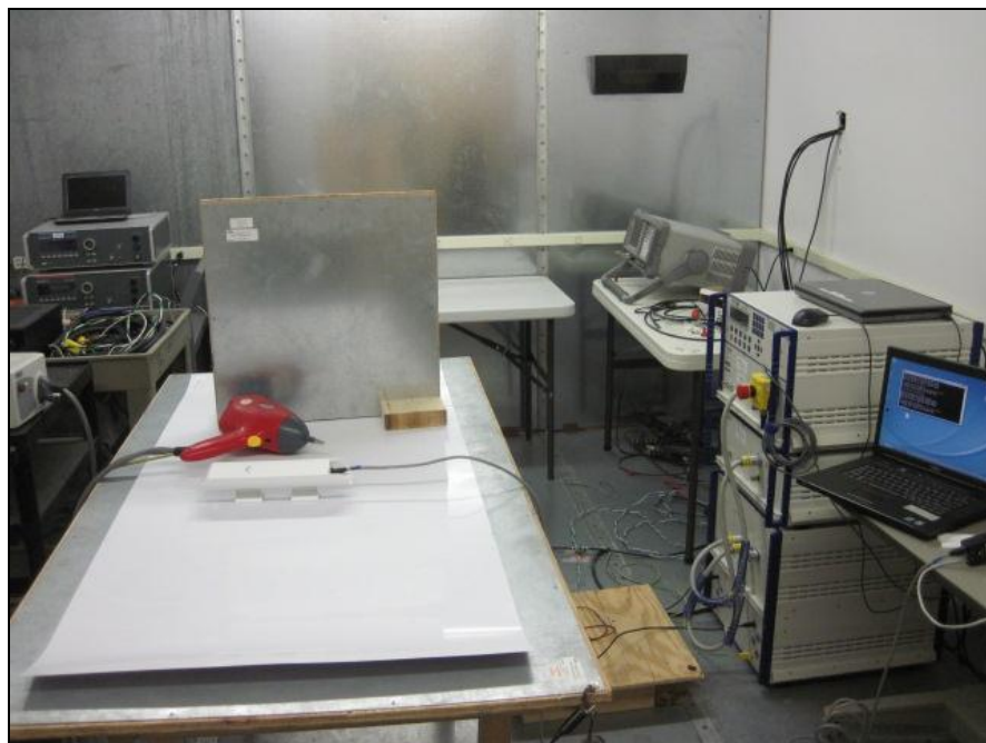
Photograph 18. Electrostatic Discharge, Test Setup, GME Power Supply
