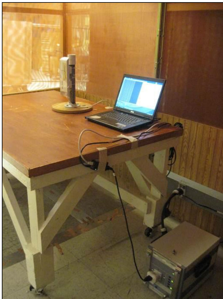
Photograph 2. AC Mains Power Conducted Disturbance, Test Setup
