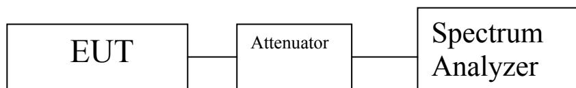
**Figure 4. Frequency Range Test Setup**
