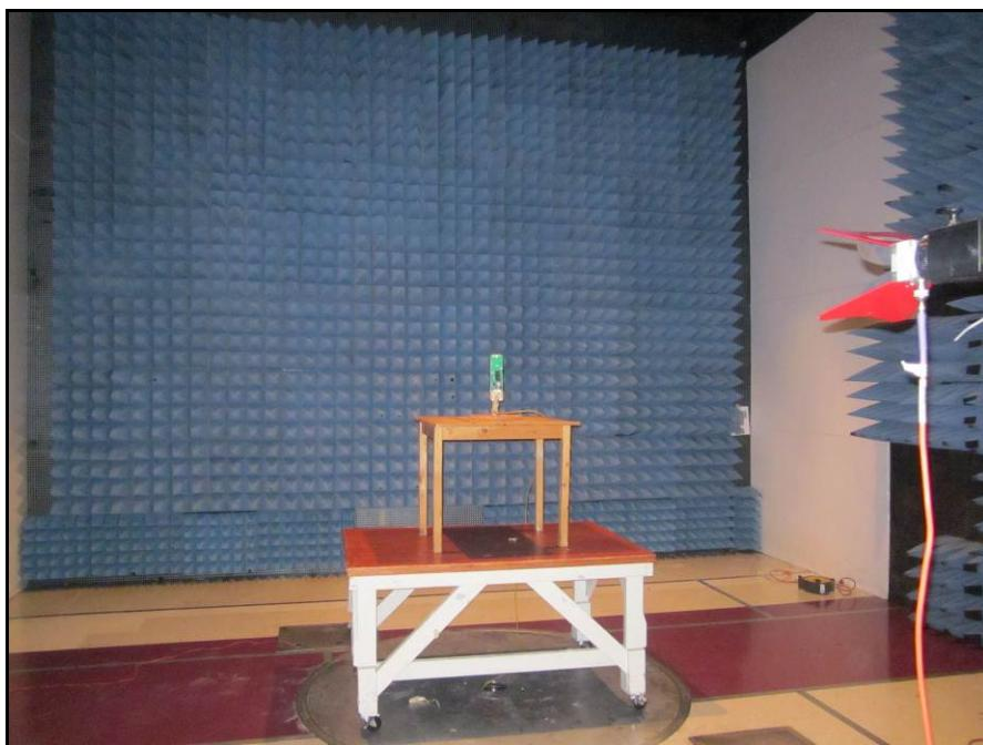
**Photograph 3. Radiated Emissions, Test Setup, 1 GHz – 12.75 GHz**
