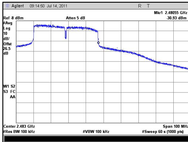
**Plot 104. Frequency Range, High Channel, Nom. Temperature, Nom. Voltage, 802.11n HT40**
