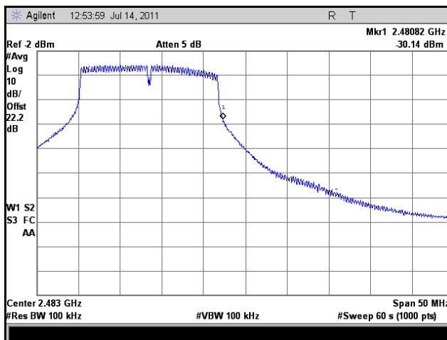
**Plot 70. Frequency Range, High Channel, High Temperature, High Voltage, 802.11g 20 MHz**
