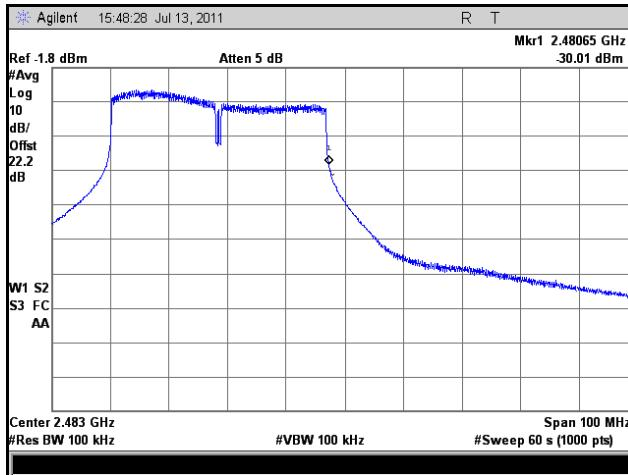
**Plot 84. Frequency Range, High Channel, Nom. Temperature, Nom. Voltage, 802.11g 40 MHz**
