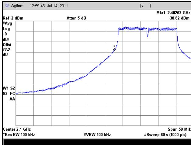
Plot 65. Frequency Range, Low Channel, High Temperature, High Voltage, 802.11g 20 MHz
