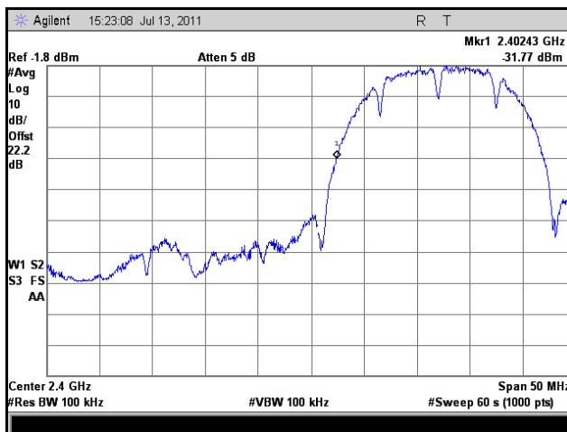
Plot 57. Frequency Range, Low Channel, Low Temperature, High Voltage, 802.11b
