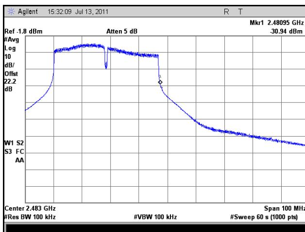
Plot 82. Frequency Range, High Channel, Low Temperature, High Voltage, 802.11g 40 MHz
