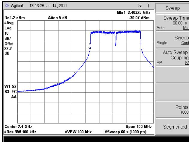
Plot 75. Frequency Range, Low Channel, High Temperature, High Voltage, 802.11g 40 MHz
