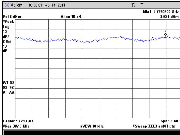
Plot 335. Peak Power Spectral Density, Low Channel, Average, 802.11a 20 MHz
