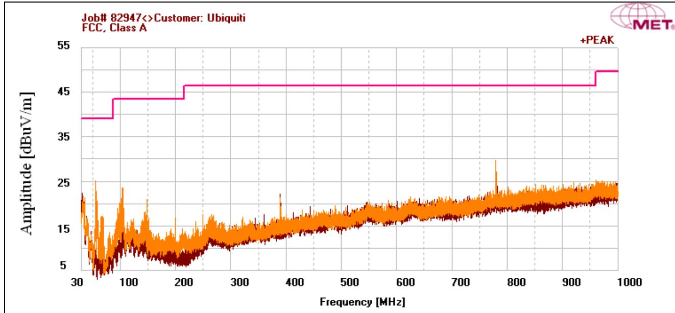
Plot 3. Radiated Emissions, 30 MHz - 1 GHz, FCC Limits
