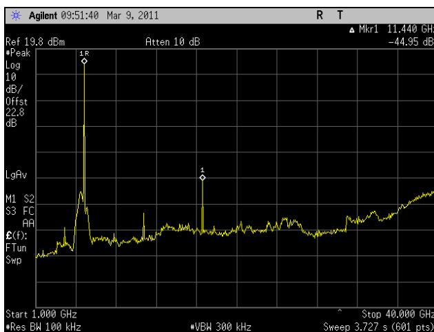
Plot 260. Conducted Spurious Emissions, Low Channel, 1 GHz – 40 GHz, 802.11n HT10, Port 1
