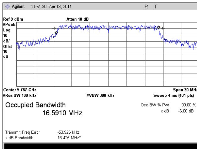
Plot 8. 6 dB Occupied Bandwidth, Mid Channel, 802.11a 20MHz
