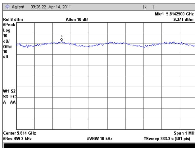
Plot 345. Peak Power Spectral Density, High Channel, Average, 802.11a 40 MHz
