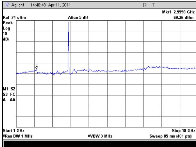
Plot 138. Radiated Spurious Emissions, High Channel, 1 GHz – 18 GHz, 802.11a 20 MHz
