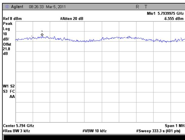
Plot 372. Peak Power Spectral Density, Mid Channel, 802.11n HT30, Port 1
