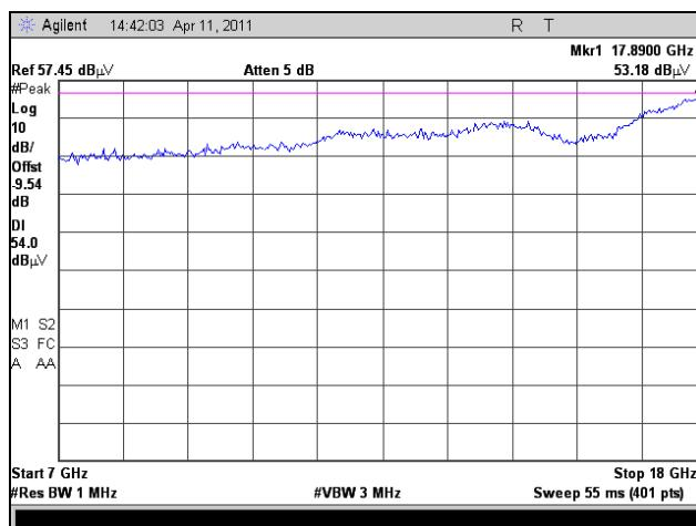
Plot 186. Radiated Harmonics, Mid Channel, 7 GHz – 18 GHz, 802.11a 40 MHz
