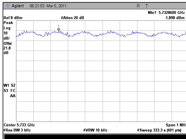
Plot 359. Peak Power Spectral Density, Low Channel, 802.11n HT10, Port 1
