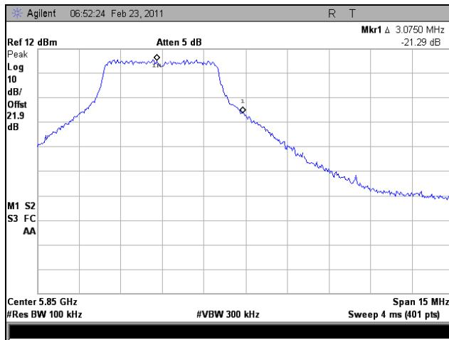
Plot 312. Conducted Band Edge, High Channel, 802.11n HT5, Port 1
