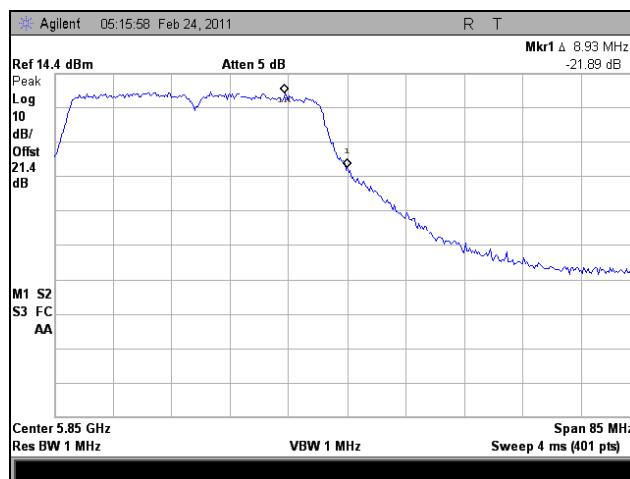
**Plot 334. Conducted Band Edge, High Channel, 802.11n HT40, Port 2**
