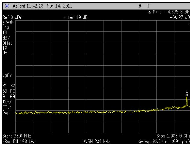
Plot 229. Conducted Spurious Emissions, Low Channel, 30 MHz – 1 GHz, 802.11a 40 MHz
