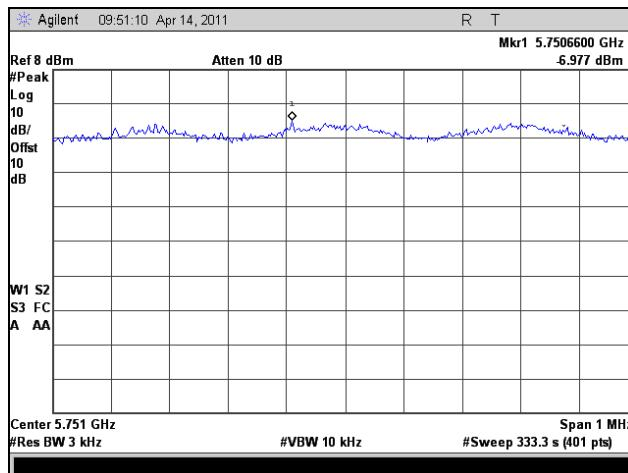
Plot 341. Peak Power Spectral Density, Low Channel, Average, 802.11a 40 MHz
