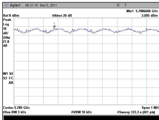
Plot 360. Peak Power Spectral Density, Mid Channel, 802.11n HT10, Port 1
