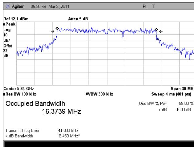
Plot 33. 6 dB Occupied Bandwidth, High Channel, 802.11n HT20, Port 1
