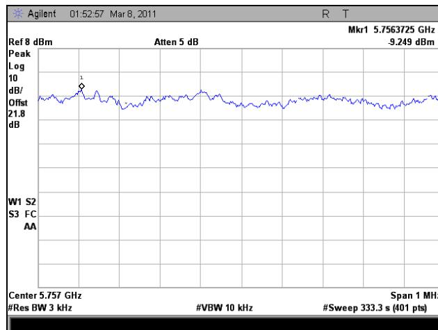
Plot 380. Peak Power Spectral Density, Low Channel, 802.11n HT40, Port 2
