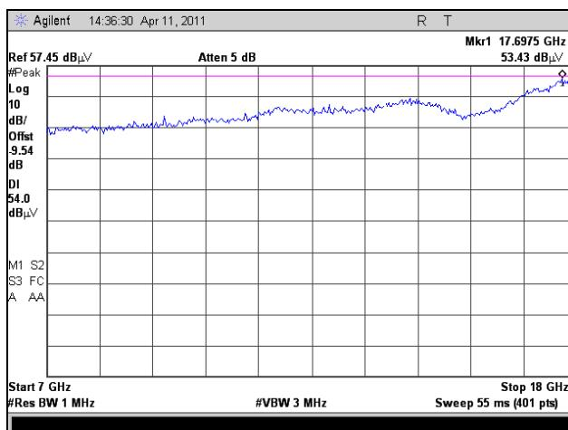
Plot 183. Radiated Harmonics, Mid Channel, 7 GHz – 18 GHz, 802.11a 20 MHz
