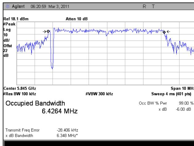
Plot 24. 6 dB Occupied Bandwidth, High Channel, 802.11n HT8, Port 2
