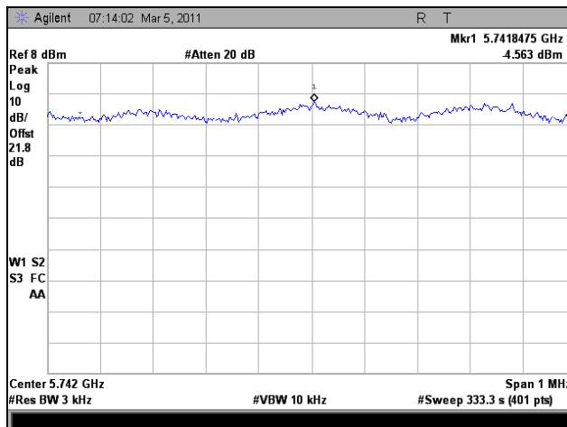
Plot 365. Peak Power Spectral Density, Low Channel, 802.11n HT20, Port 1
