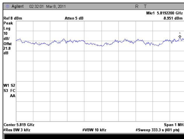
Plot 382. Peak Power Spectral Density, High Channel, 802.11n HT40, Port 2
