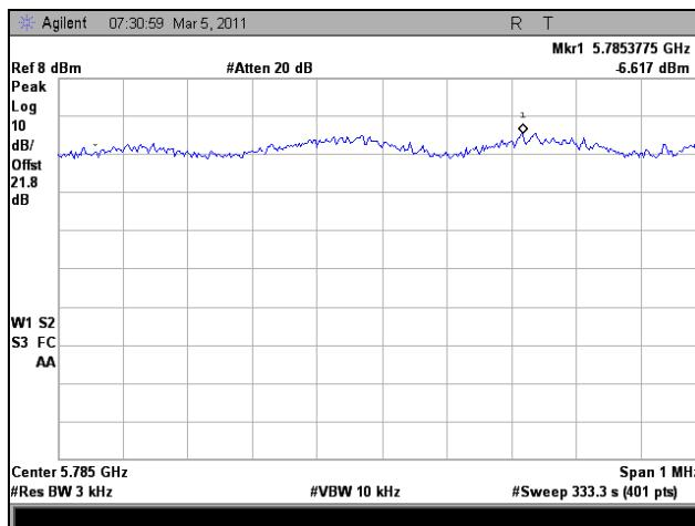
Plot 366. Peak Power Spectral Density, Mid Channel, 802.11n HT20, Port 1
