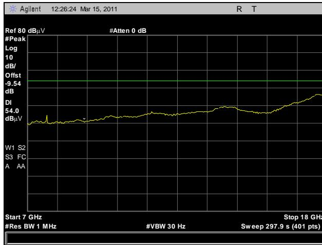
Plot 207. Radiated Harmonics, Mid Channel, 7 GHz – 18 GHz, Average, 802.11n HT20
