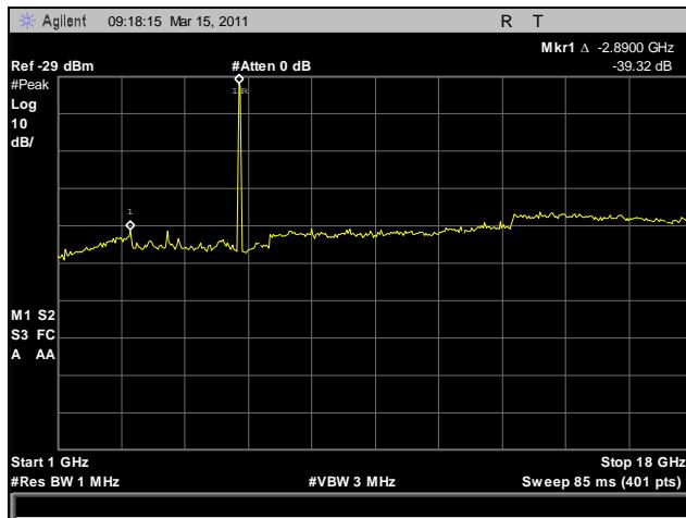
Plot 150. Radiated Spurious Emissions, High Channel, 1 GHz – 18 GHz, 802.11n HT5
