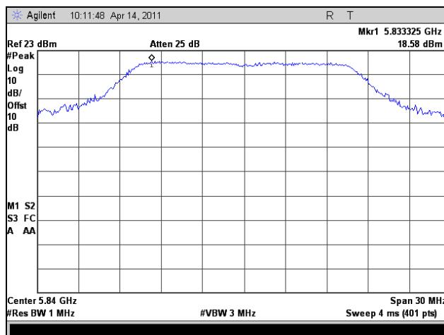
Plot 340. Peak Power Spectral Density, High Channel, Peak, 802.11a 20 MHz
