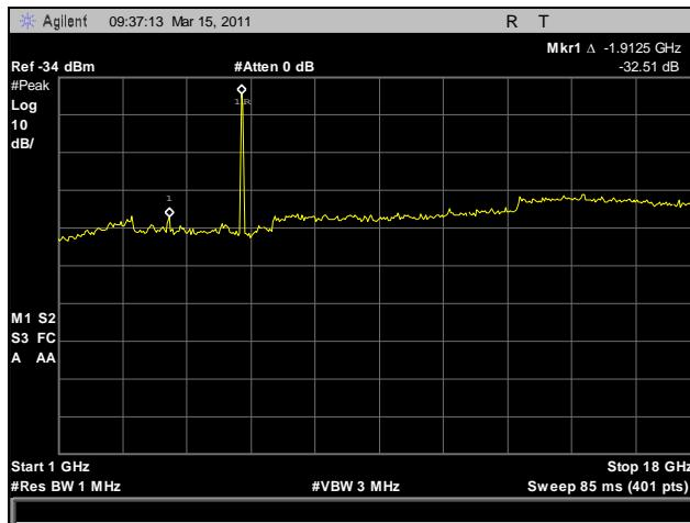
Plot 174. Radiated Spurious Emissions, High Channel, 1 GHz – 18 GHz, 802.11n HT30
