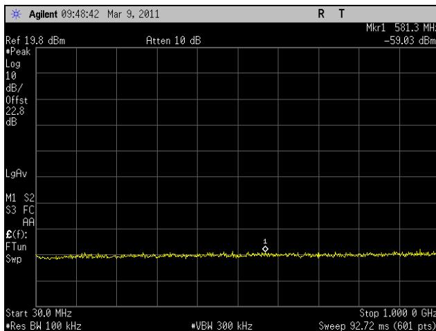
Plot 253. Conducted Spurious Emissions, Low Channel, 30 MHz – 1 GHz, 802.11n HT8, Port 2
