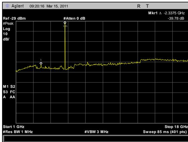
Plot 148. Radiated Spurious Emissions, Mid Channel, 1 GHz – 18 GHz, 802.11n HT5
