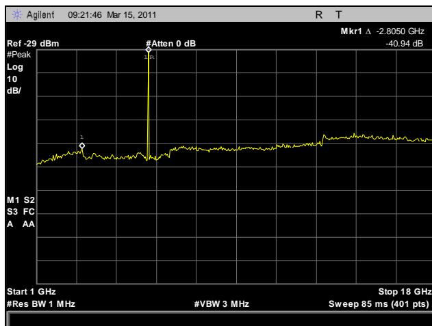
Plot 146. Radiated Spurious Emissions, Low Channel, 1 GHz – 18 GHz, 802.11n HT5
