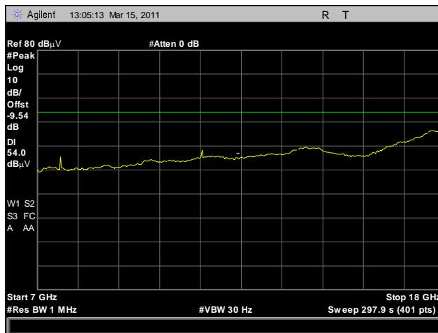
Plot 193. Radiated Harmonics, Low Channel, 7 GHz – 18 GHz, Average, 802.11n HT8
