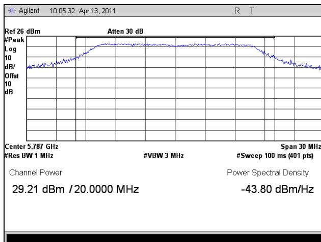
Plot 92. Peak Power Output, Mid Channel, 802.11a 20 MHz
