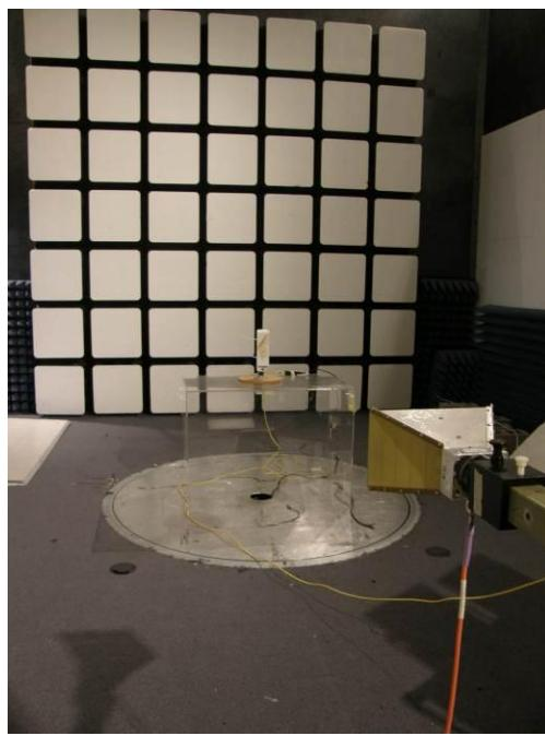
Photograph 7. Radiated Spurious Emissions, Test Setup, 1 GHz – 18 GHz
