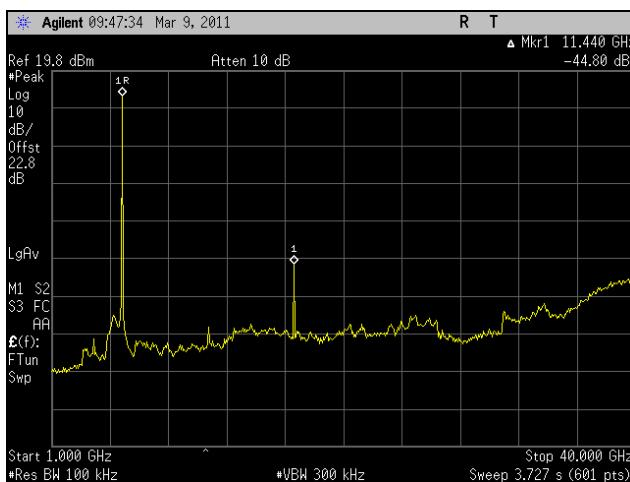
Plot 254. Conducted Spurious Emissions, Low Channel, 1 GHz – 40 GHz, 802.11n HT8, Port 2
