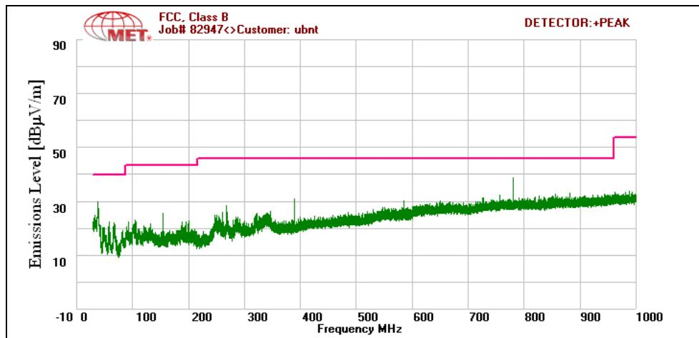
Plot 139. Radiated Spurious Emissions, Low Channel, 30 MHz – 1 GHz, 802.11a 40 MHz
