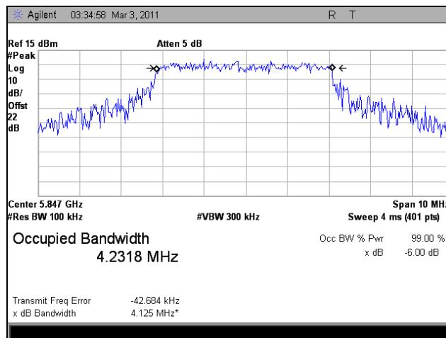
Plot 15. 6 dB Occupied Bandwidth, High Channel, 802.11n HT5, Port 1
