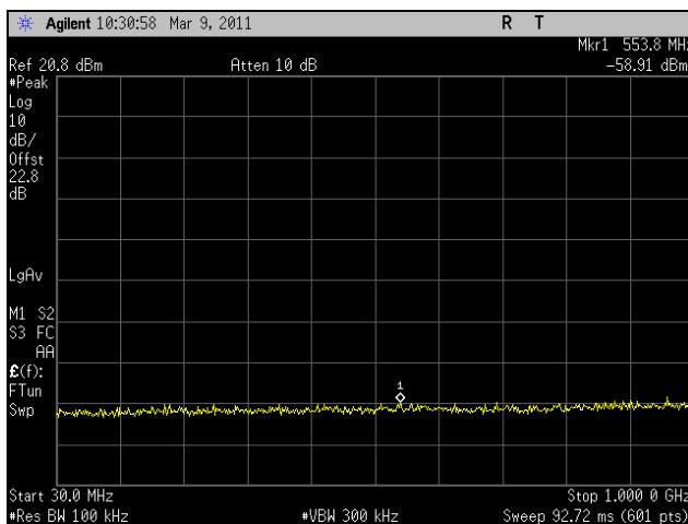
Plot 255. Conducted Spurious Emissions, Mid Channel, 30 MHz – 1 GHz, 802.11n HT8, Port 2
