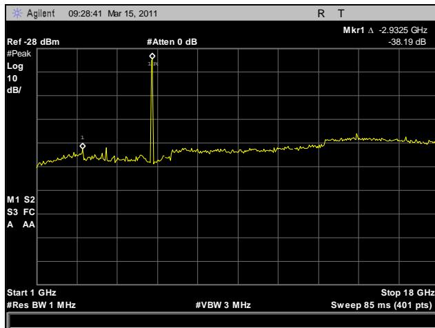
Plot 162. Radiated Spurious Emissions, High Channel, 1 GHz – 18 GHz, 802.11n HT10
