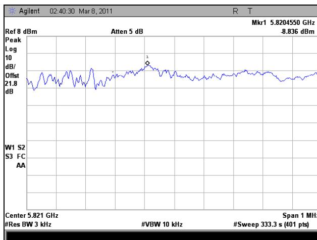
Plot 379. Peak Power Spectral Density, High Channel, 802.11n HT40, Port 1
