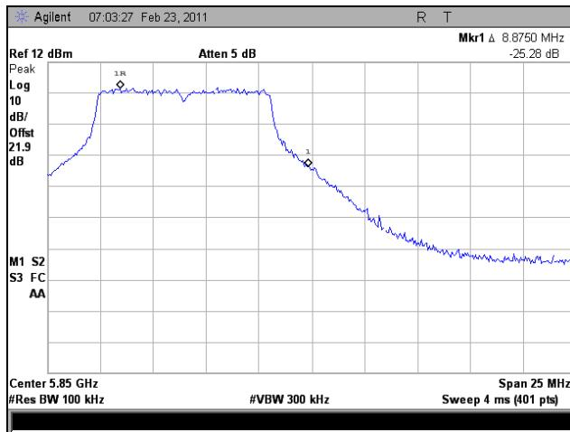
Plot 320. Conducted Band Edge, High Channel, 802.11n HT10, Port 1
