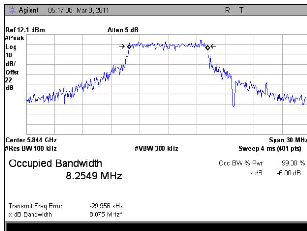
Plot 27. 6 dB Occupied Bandwidth, High Channel, 802.11n HT10, Port 1
