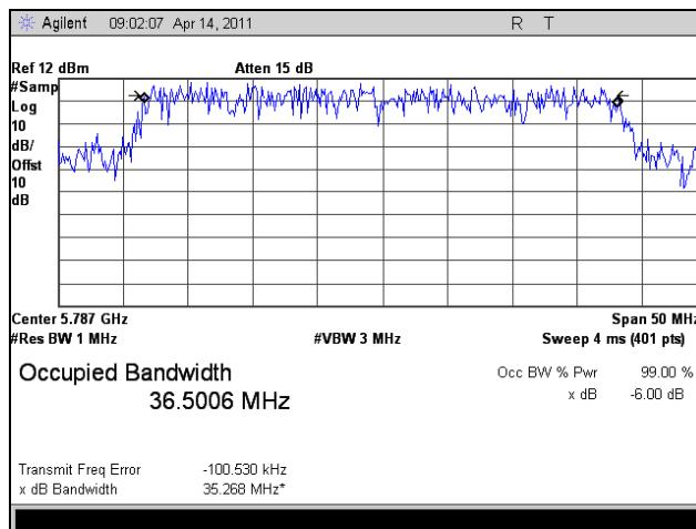
Plot 53. 99% Occupied Bandwidth, Mid Channel, 802.11a 40 MHz
