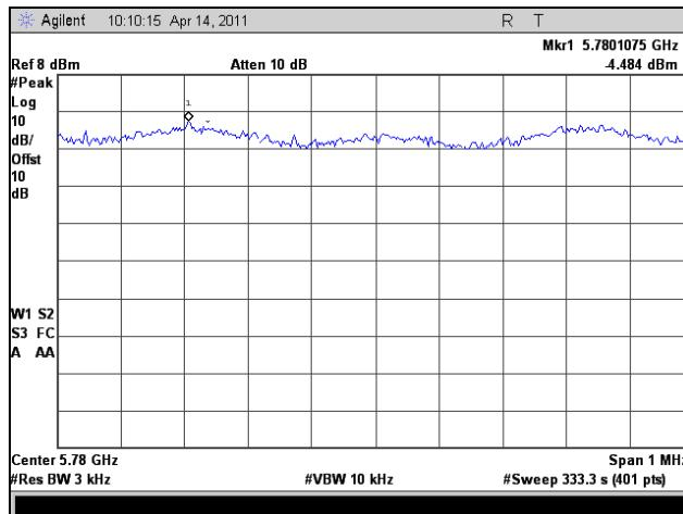
Plot 337. Peak Power Spectral Density, Mid Channel, Average, 802.11a 20 MHz
