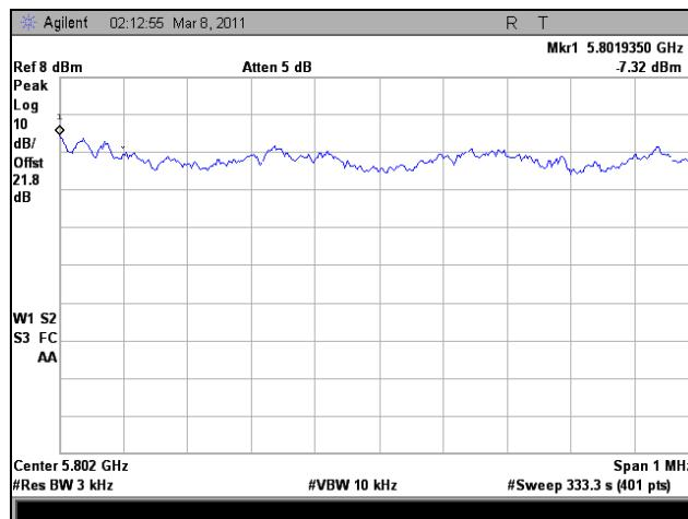
Plot 381. Peak Power Spectral Density, Mid Channel, 802.11n HT40, Port 2
