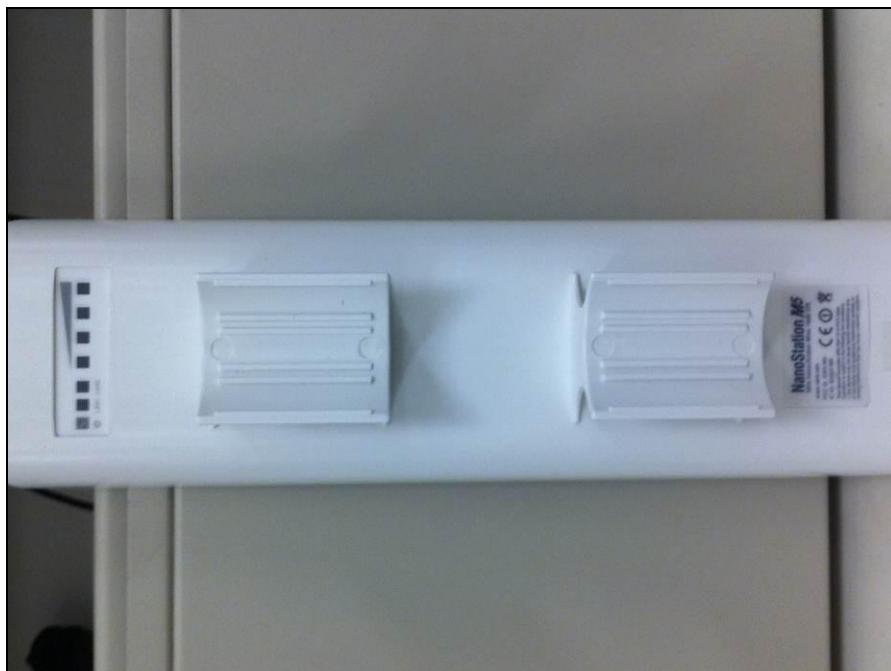
**Photograph 2. Ubiquiti Networks NanoStationM5, Rear View**
