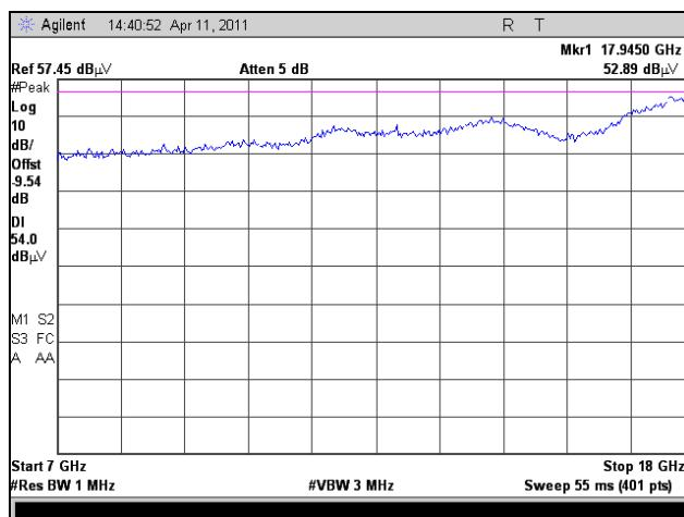
Plot 185. Radiated Harmonics, Low Channel, 7 GHz – 18 GHz, 802.11a 40 MHz
