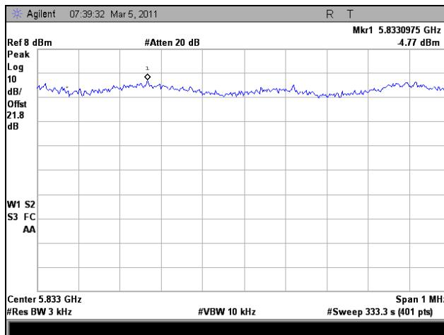
Plot 370. Peak Power Spectral Density, High Channel, 802.11n HT20, Port 2
