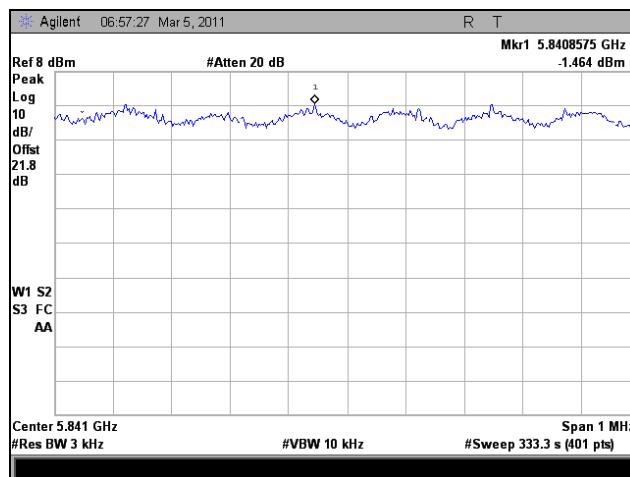
Plot 364. Peak Power Spectral Density, High Channel, 802.11n HT10, Port 2
