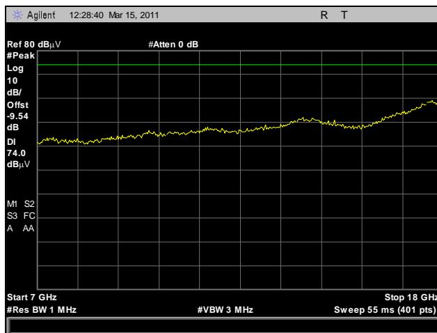
**Plot 210. Radiated Harmonics, High Channel, 7 GHz – 18 GHz, Peak, 802.11n HT20**
