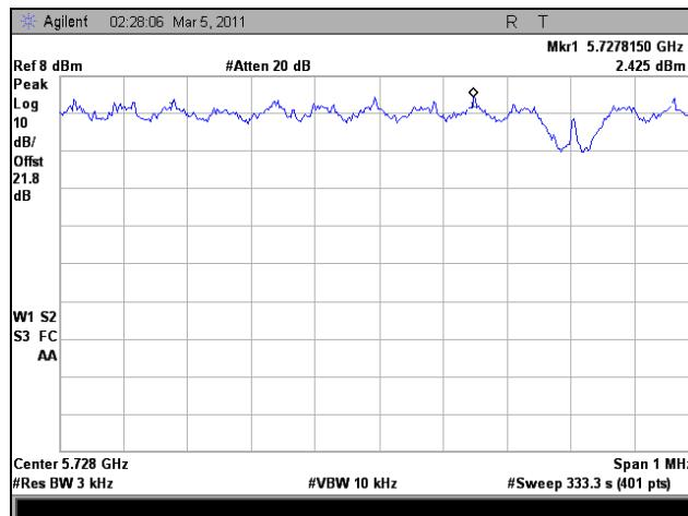
Plot 347. Peak Power Spectral Density, Low Channel, 802.11n HT5, Port 1
