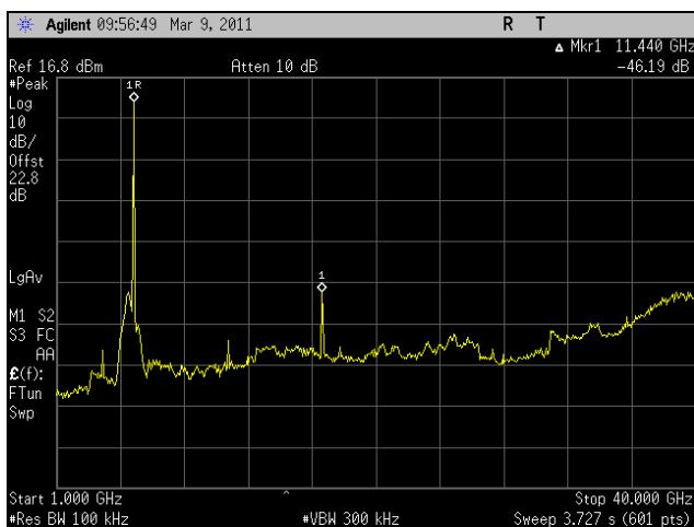
**Plot 272. Conducted Spurious Emissions, Low Channel, 1 GHz – 40 GHz, 802.11n HT20, Port 1**
