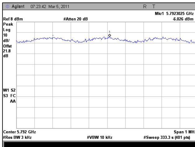
Plot 369. Peak Power Spectral Density, Mid Channel, 802.11n HT20, Port 2
