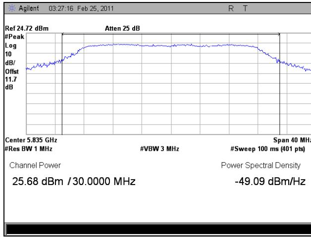
Plot 126. Peak Power Output, High Channel, 802.11n HT30, Port 2
