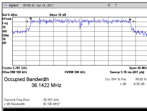
Plot 11. 6 dB Occupied Bandwidth, Mid Channel, 802.11a 40 MHz
