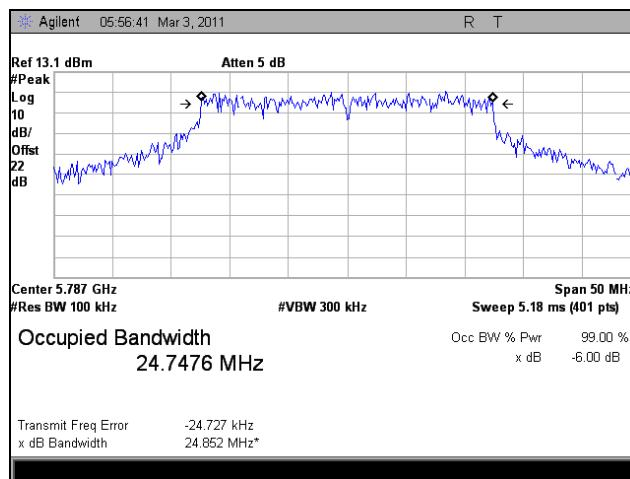
Plot 41. 6 dB Occupied Bandwidth, Mid Channel, 802.11n HT30, Port 2
