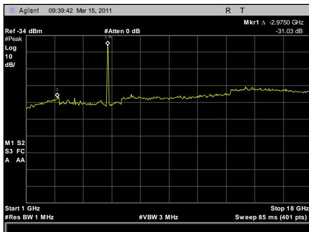
Plot 176. Radiated Spurious Emissions, Low Channel, 1 GHz – 18 GHz, 802.11n HT40
