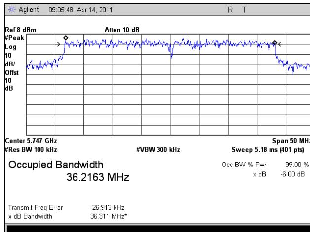
Plot 10. 6 dB Occupied Bandwidth, Low Channel, 802.11a 40 MHz
