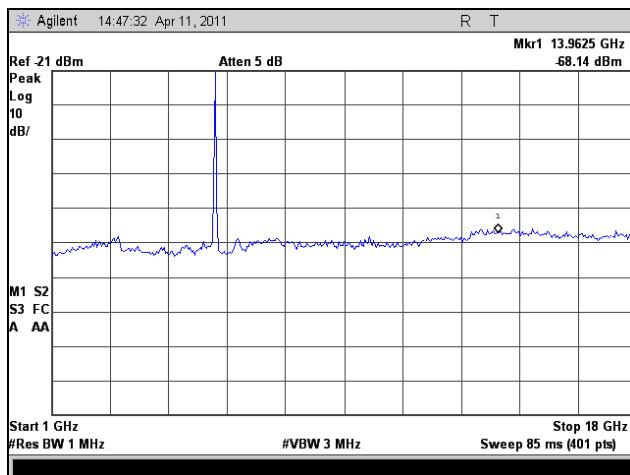
Plot 134. Radiated Spurious Emissions, Low Channel, 1 GHz – 18 GHz, 802.11a 20 MHz
