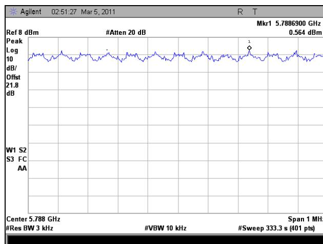
Plot 348. Peak Power Spectral Density, Mid Channel, 802.11n HT5, Port 1
