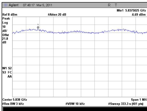
Plot 367. Peak Power Spectral Density, High Channel, 802.11n HT20, Port 1
