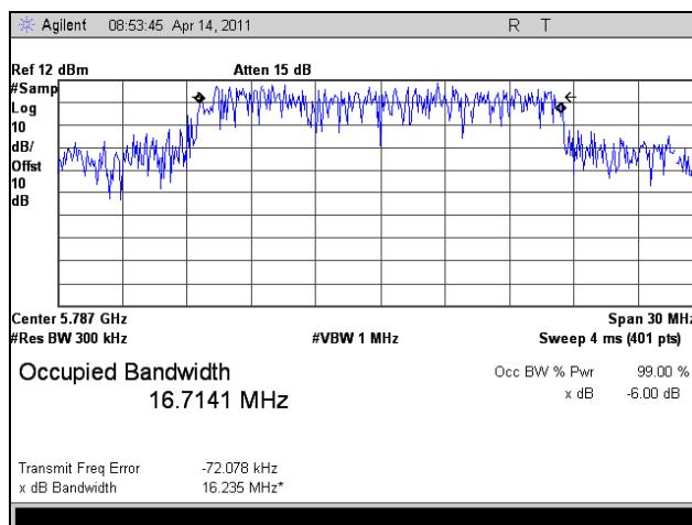
Plot 50. 99% Occupied Bandwidth, Mid Channel, 802.11a 20 MHz
