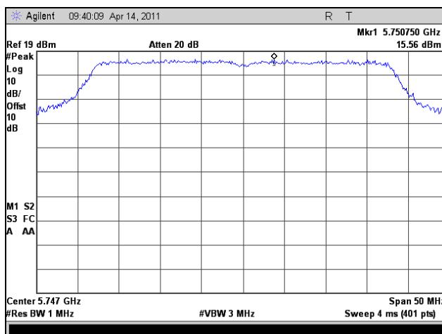
Plot 342. Peak Power Spectral Density, Low Channel, Peak, 802.11a 40 MHz
