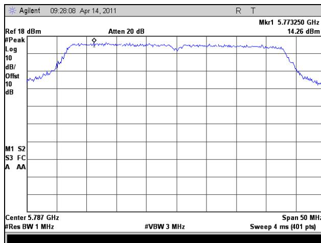
Plot 344. Peak Power Spectral Density, Mid Channel, Peak, 802.11a 40 MHz
