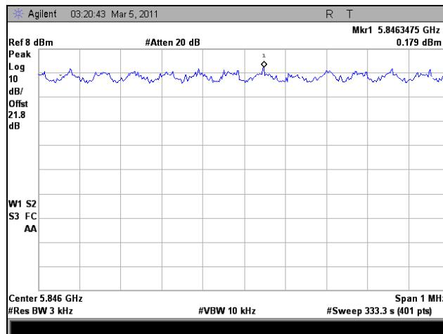
Plot 349. Peak Power Spectral Density, High Channel, 802.11n HT5, Port 1
