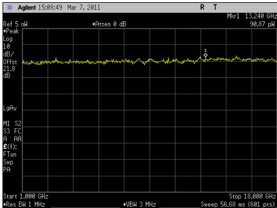
Plot 384. Receiver Spurious Emission, 1 GHz – 18 GHz, Port 1
