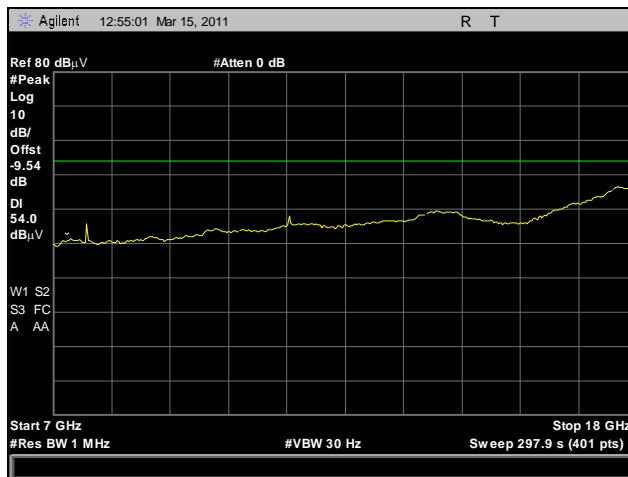
Plot 199. Radiated Harmonics, Low Channel, 7 GHz – 18 GHz, Average, 802.11n HT10
