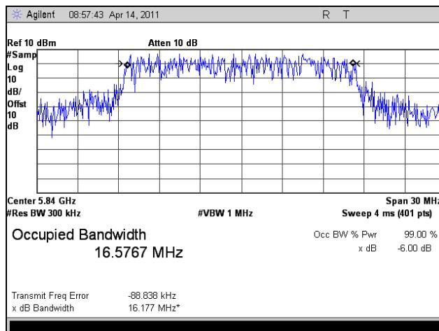
Plot 51. 99% Occupied Bandwidth, High Channel, 802.11a 20 MHz
