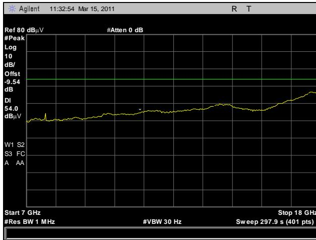
Plot 219. Radiated Harmonics, Mid Channel, 7 GHz – 18 GHz, Average, 802.11n HT40
