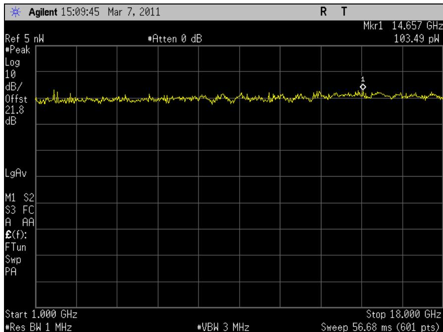
Plot 386. Receiver Spurious Emission, 1 GHz – 18 GHz, Port 2
