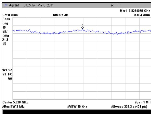
Plot 376. Peak Power Spectral Density, High Channel, 802.11n HT30, Port 2
