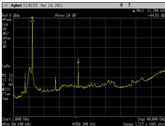
Plot 230. Conducted Spurious Emissions, Low Channel, 1 GHz – 40 GHz, 802.11a 40 MHz
