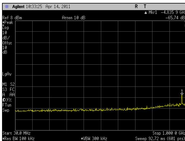
Plot 225. Conducted Spurious Emissions, Mid Channel, 30 MHz – 1 GHz, 802.11a 20 MHz
