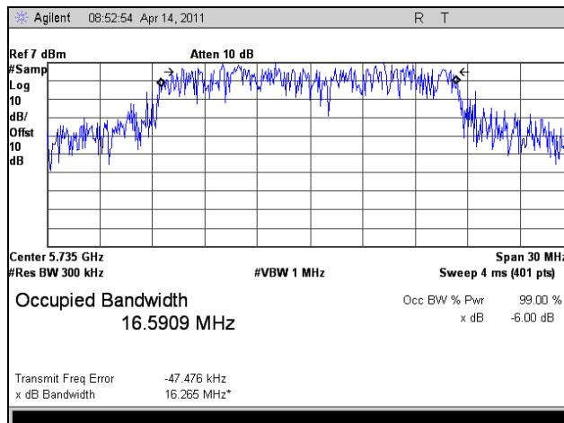
Plot 49. 99% Occupied Bandwidth, Low Channel, 802.11a 20 MHz
