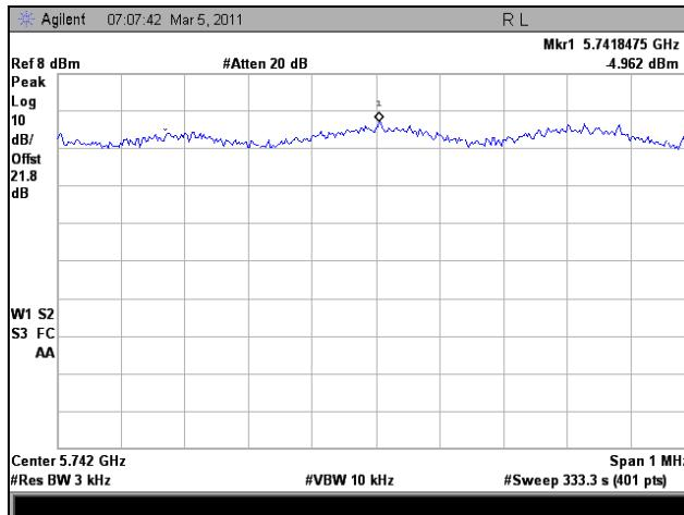
Plot 368. Peak Power Spectral Density, Low Channel, 802.11n HT20, Port 2
