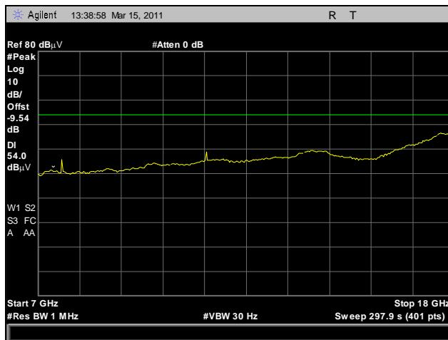
Plot 187. Radiated Harmonics, Low Channel, 7 GHz – 18 GHz, Average, 802.11n HT5
