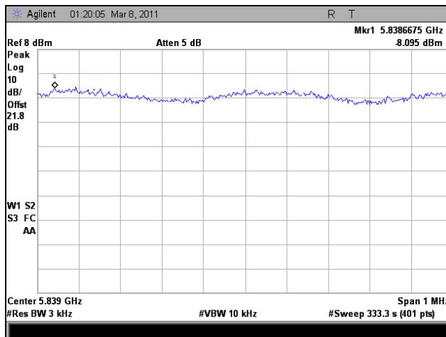
Plot 373. Peak Power Spectral Density, High Channel, 802.11n HT30, Port 1
