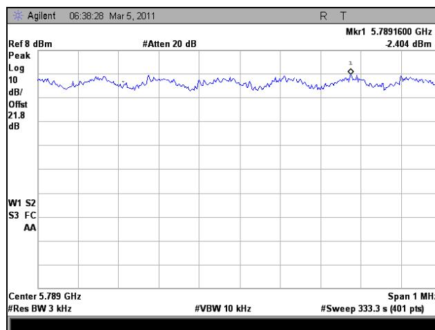
Plot 363. Peak Power Spectral Density, Mid Channel, 802.11n HT10, Port 2
