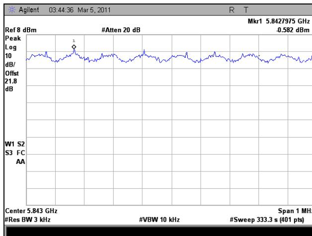
Plot 355. Peak Power Spectral Density, High Channel, 802.11n HT8, Port 1
