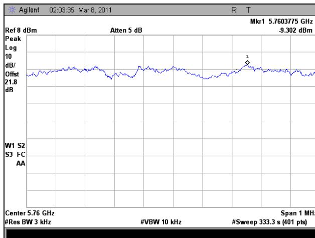
Plot 377. Peak Power Spectral Density, Low Channel, 802.11n HT40, Port 1
