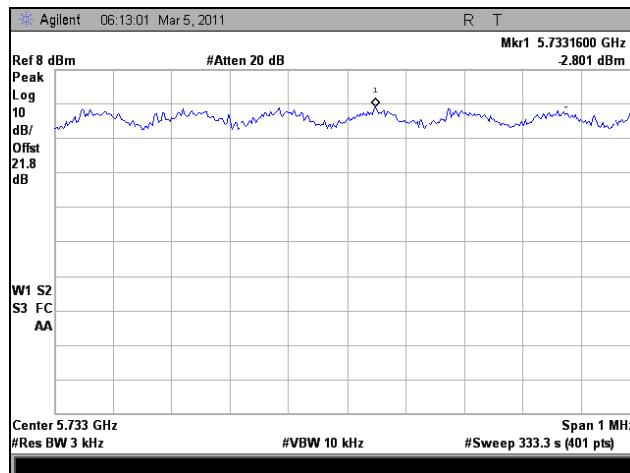
Plot 362. Peak Power Spectral Density, Low Channel, 802.11n HT10, Port 2
