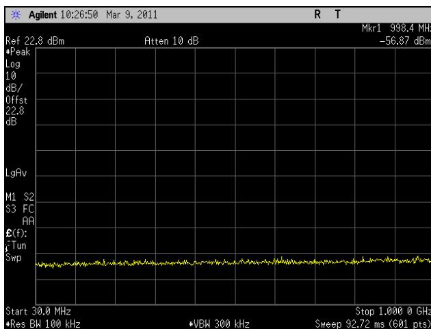
Plot 237. Conducted Spurious Emissions, Mid Channel, 30 MHz – 1 GHz, 802.11n HT5, Port 1
