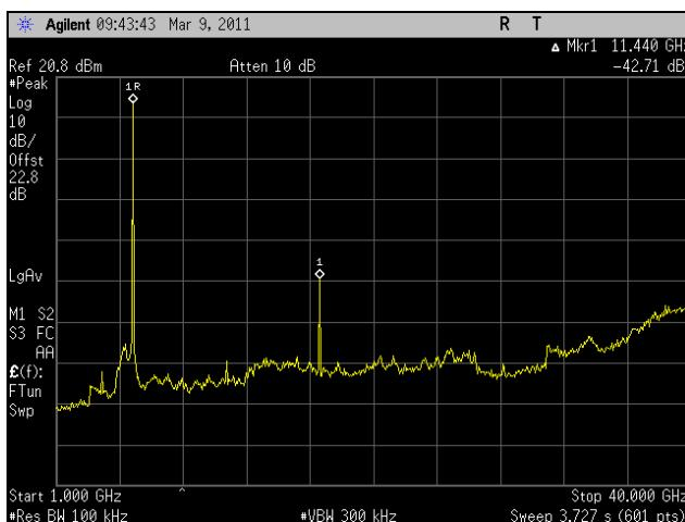
**Plot 242.** Conducted Spurious Emissions, Low Channel, 1 GHz – 40 GHz, 802.11n HT5, Port 2
