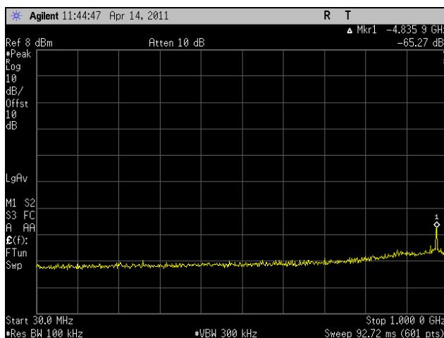
Plot 231. Conducted Spurious Emissions, Mid Channel, 30 MHz – 1 GHz, 802.11a 40 MHz
