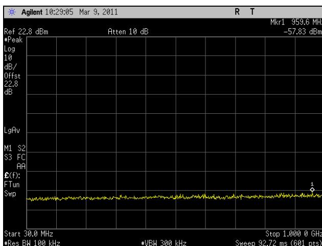
**Plot 243.** Conducted Spurious Emissions, Mid Channel, 30 MHz – 1 GHz, 802.11n HT5, Port 2
