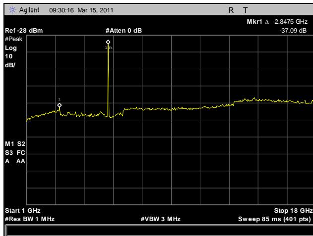
Plot 160. Radiated Spurious Emissions, Mid Channel, 1 GHz – 18 GHz, 802.11n HT10
