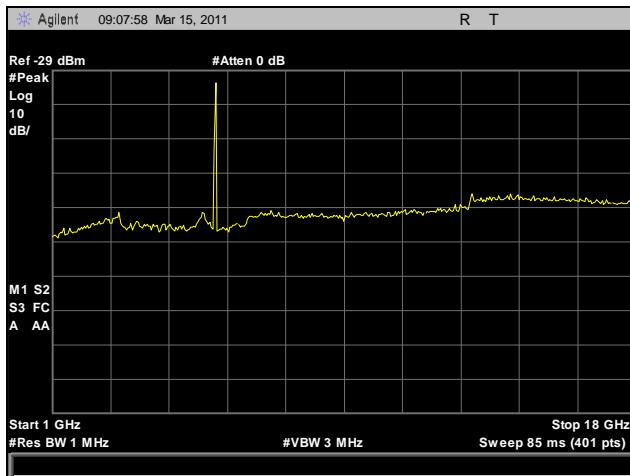
**Plot 168.** Radiated Spurious Emissions, High Channel, 1 GHz – 18 GHz, 802.11n HT20
