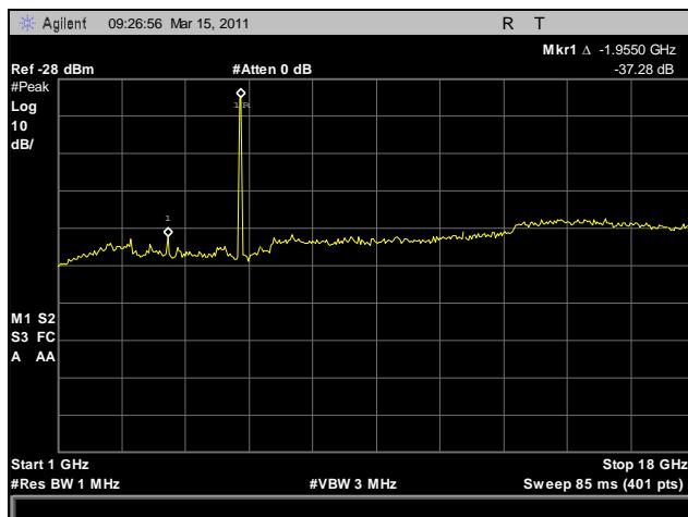
Plot 152. Radiated Spurious Emissions, Low Channel, 1 GHz – 18 GHz, 802.11n HT8
