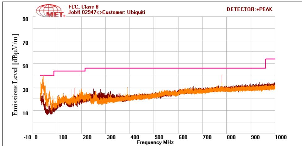
Plot 175. Radiated Spurious Emissions, Low Channel, 30 MHz – 1 GHz, 802.11n HT40
