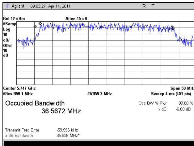
Plot 52. 99% Occupied Bandwidth, Low Channel, 802.11a 40 MHz
