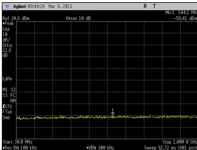
**Plot 241.** Conducted Spurious Emissions, Low Channel, 30 MHz – 1 GHz, 802.11n HT5, Port 2
