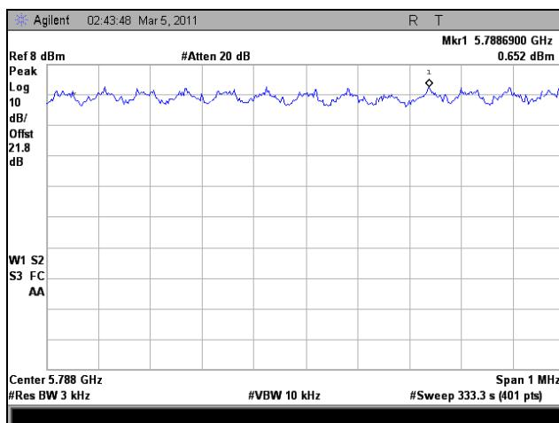
Plot 351. Peak Power Spectral Density, Mid Channel, 802.11n HT5, Port 2
