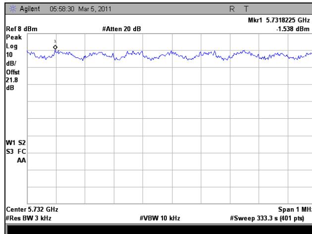
Plot 356. Peak Power Spectral Density, Low Channel, 802.11n HT8, Port 2
