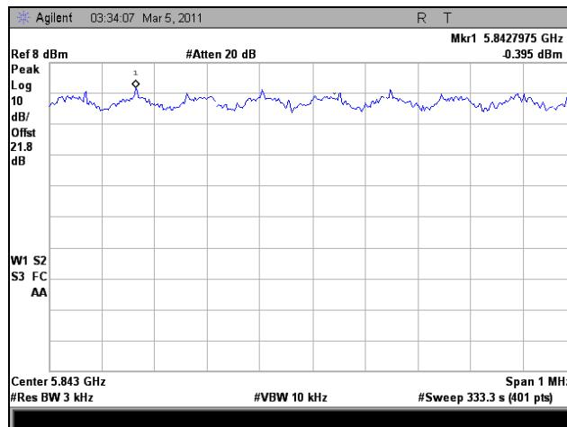
Plot 358. Peak Power Spectral Density, High Channel, 802.11n HT8, Port 2
