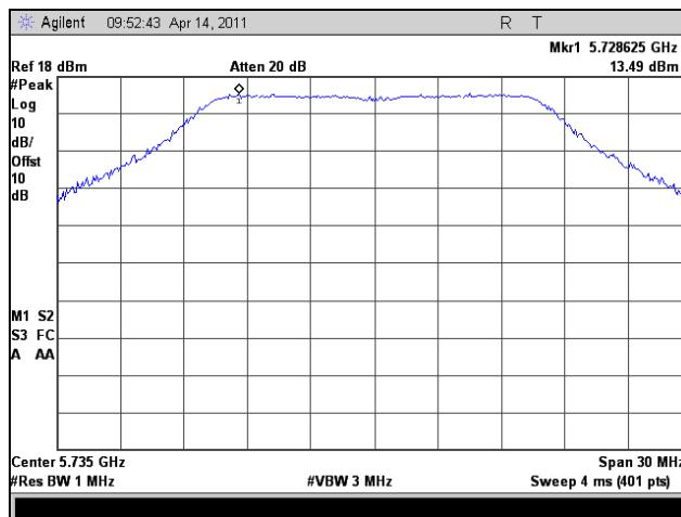
Plot 336. Peak Power Spectral Density, Low Channel, Peak, 802.11a 20 MHz
