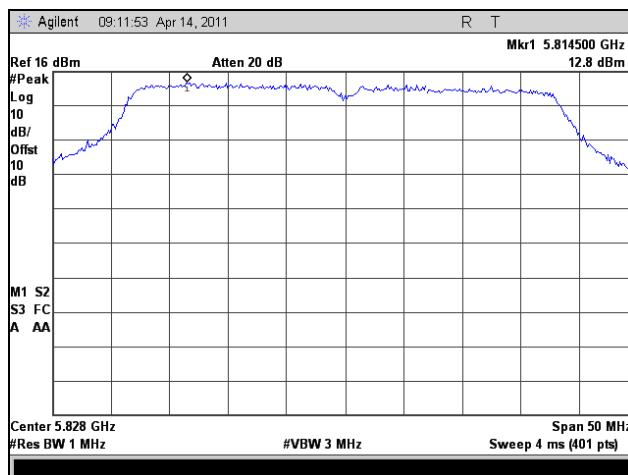
Plot 346. Peak Power Spectral Density, High Channel, Peak, 802.11a 40 MHz
