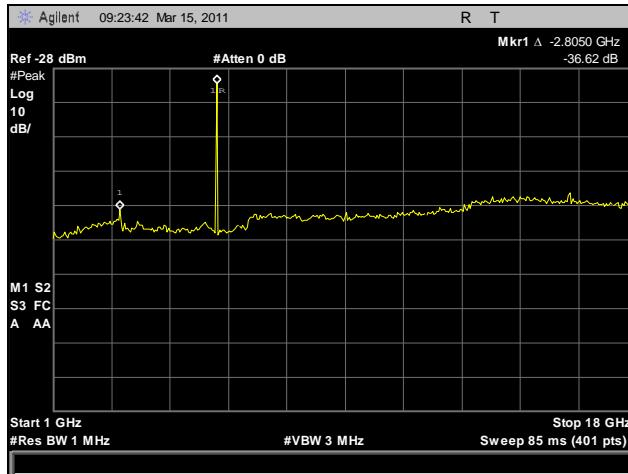
Plot 156. Radiated Spurious Emissions, High Channel, 1 GHz – 18 GHz, 802.11n HT8
