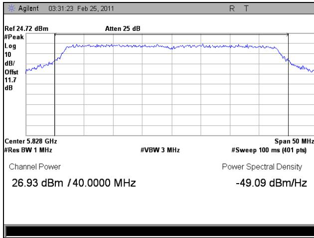
Plot 129. Peak Power Output, High Channel, 802.11n HT40, Port 1
