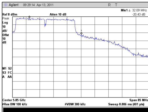
Plot 310. Conducted Band Edge, High Channel, 802.11a 40 MHz
