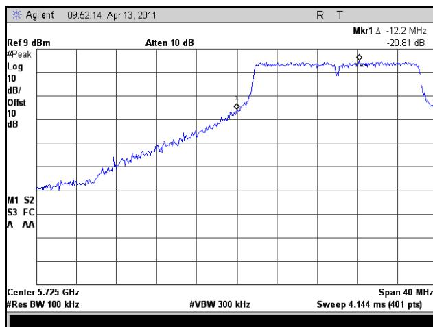
Plot 307. Conducted Band Edge, Low Channel, 802.11a 20 MHz
