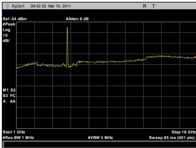
Plot 180. Radiated Spurious Emissions, High Channel, 1 GHz – 18 GHz, 802.11n HT40
