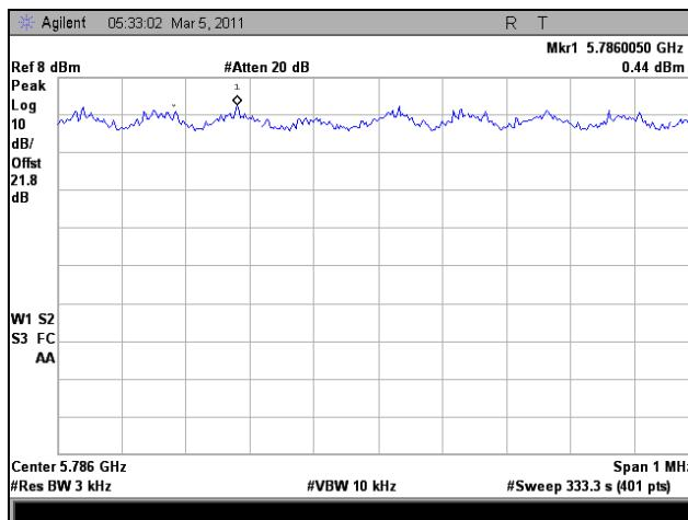
Plot 354. Peak Power Spectral Density, Mid Channel, 802.11n HT8, Port 1
