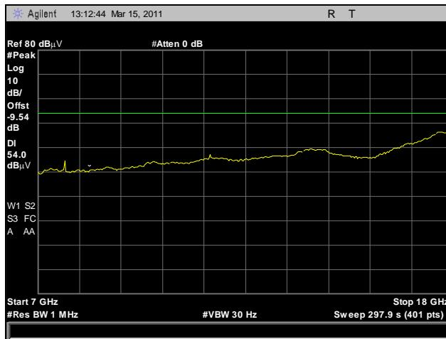
Plot 195. Radiated Harmonics, Mid Channel, 7 GHz – 18 GHz, Average, 802.11n HT8
