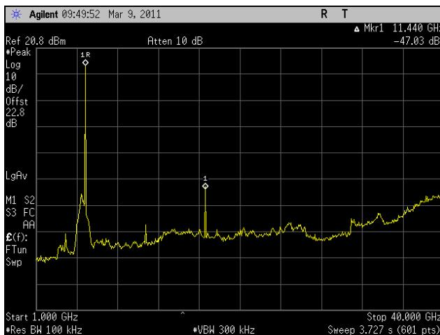
**Plot 248. Conducted Spurious Emissions, Low Channel, 1 GHz – 40 GHz, 802.11n HT8, Port 1**
