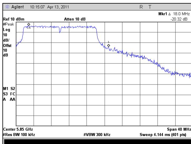
Plot 308. Conducted Band Edge, High Channel, 802.11a 20 MHz
