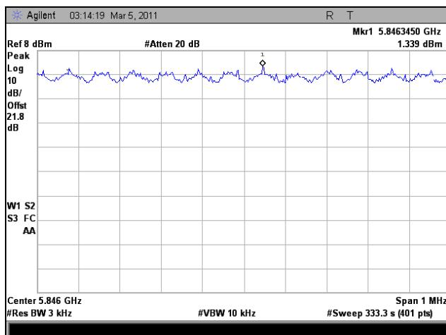
Plot 352. Peak Power Spectral Density, High Channel, 802.11n HT5, Port 2
