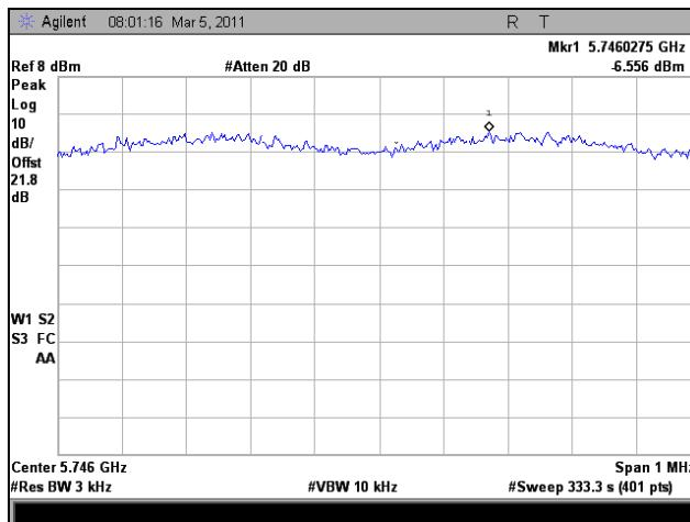
Plot 374. Peak Power Spectral Density, Low Channel, 802.11n HT30, Port 2
