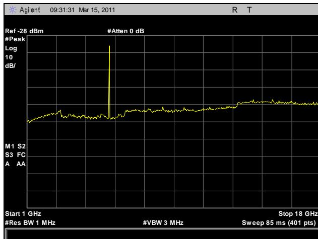
Plot 158. Radiated Spurious Emissions, Low Channel, 1 GHz – 18 GHz, 802.11n HT10
