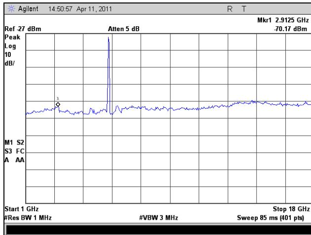
Plot 144. Radiated Spurious Emissions, High Channel, 1 GHz – 18 GHz, 802.11a 40 MHz
