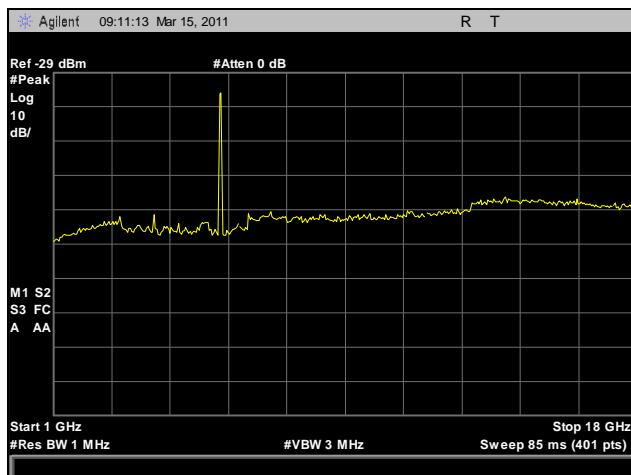
Plot 164. Radiated Spurious Emissions, Low Channel, 1 GHz – 18 GHz, 802.11n HT20
