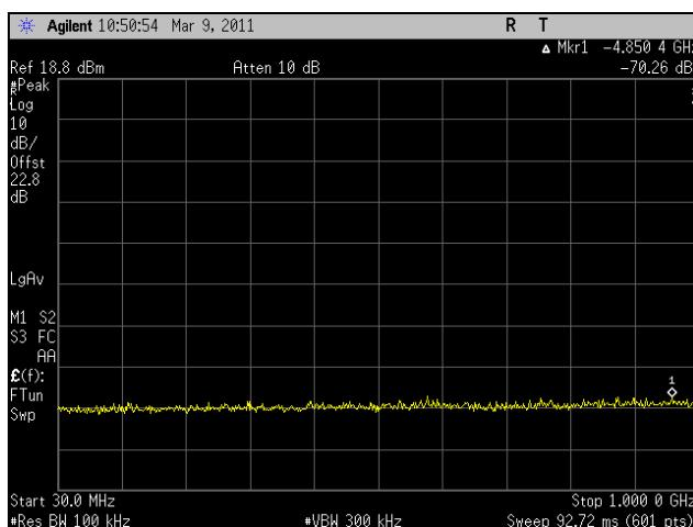
Plot 303. Conducted Spurious Emissions, Mid Channel, 30 MHz – 1 GHz, 802.11n HT40, Port 2
