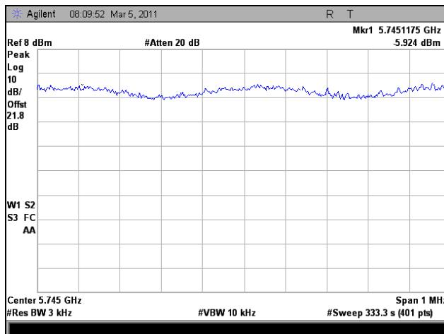
Plot 371. Peak Power Spectral Density, Low Channel, 802.11n HT30, Port 1
