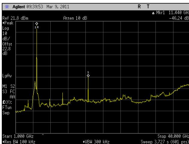
Plot 236. Conducted Spurious Emissions, Low Channel, 1 GHz – 40 GHz, 802.11n HT5, Port 1
