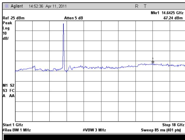
Plot 142. Radiated Spurious Emissions, Mid Channel, 1 GHz – 18 GHz, 802.11a 40 MHz
