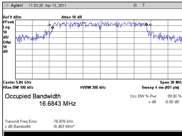
Plot 9. 6 dB Occupied Bandwidth, High Channel, 802.11a 20MHz
