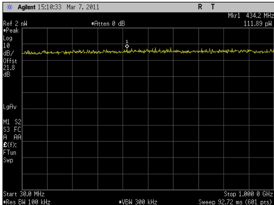
Plot 385. Receiver Spurious Emission, 30 MHz – 1 GHz, Port 2
