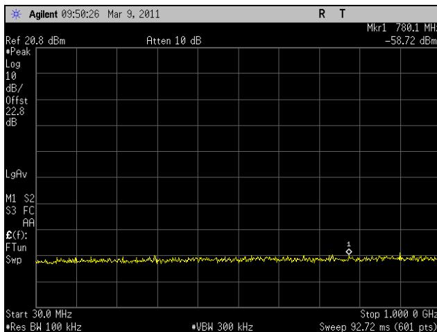
**Plot 247. Conducted Spurious Emissions, Low Channel, 30 MHz – 1 GHz, 802.11n HT8, Port 1**
