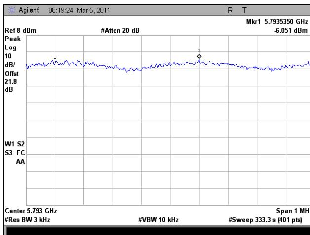
Plot 375. Peak Power Spectral Density, Mid Channel, 802.11n HT30, Port 2
