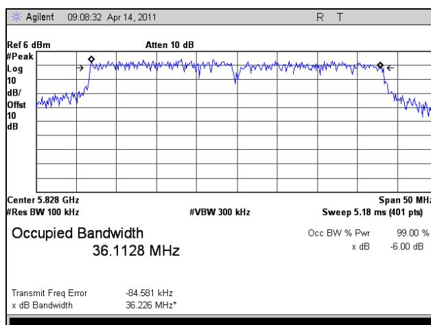
Plot 12. 6 dB Occupied Bandwidth, High Channel, 802.11a 40 MHz
