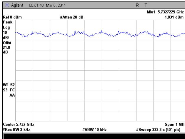
Plot 353. Peak Power Spectral Density, Low Channel, 802.11n HT8, Port 1
