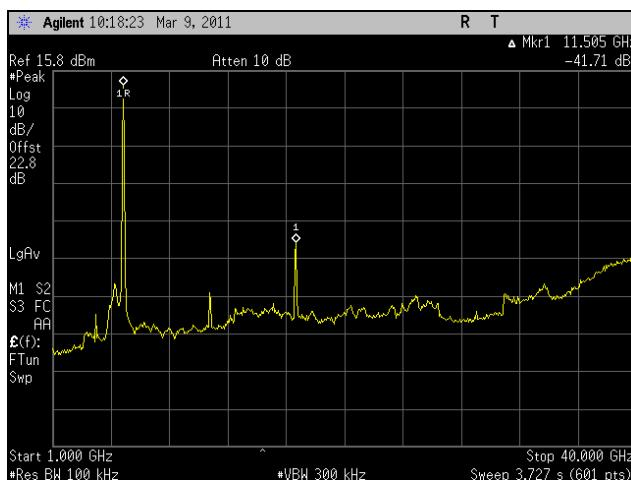
Plot 302. Conducted Spurious Emissions, Low Channel, 1 GHz – 40 GHz, 802.11n HT40, Port 2
