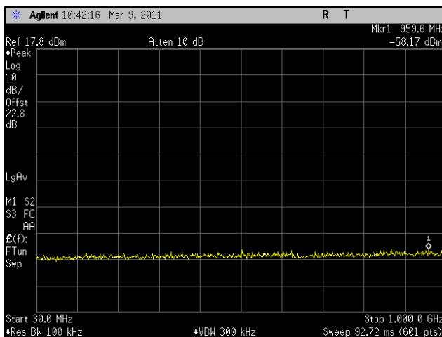
Plot 261. Conducted Spurious Emissions, Mid Channel, 30 MHz – 1 GHz, 802.11n HT10, Port 1
