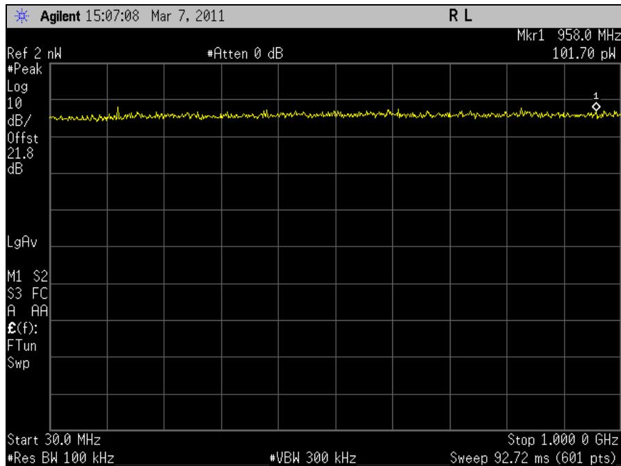
Plot 383. Receiver Spurious Emission, 30 MHz – 1 GHz, Port 1
