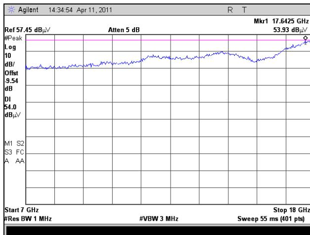
Plot 181. Radiated Harmonics, Low Channel, 7 GHz – 18 GHz, 802.11a 20 MHz
