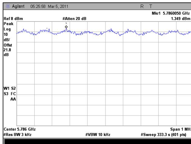
Plot 357. Peak Power Spectral Density, Mid Channel, 802.11n HT8, Port 2
