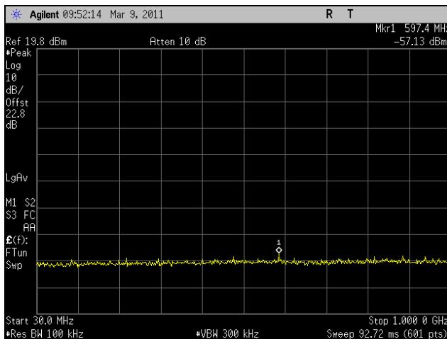
Plot 259. Conducted Spurious Emissions, Low Channel, 30 MHz – 1 GHz, 802.11n HT10, Port 1
