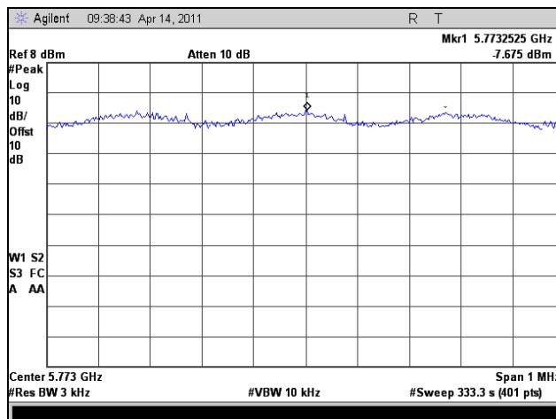
Plot 343. Peak Power Spectral Density, Mid Channel, Average, 802.11a 40 MHz
