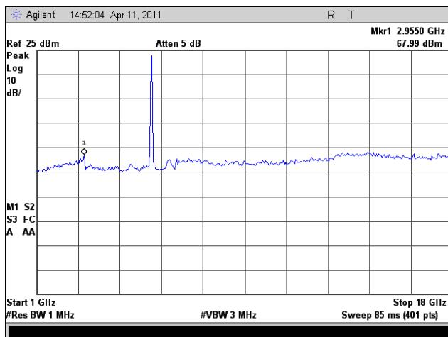
Plot 140. Radiated Spurious Emissions, Low Channel, 1 GHz – 18 GHz, 802.11a 40 MHz
