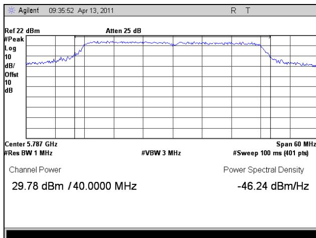
Plot 95. Peak Power Output, Mid Channel, 802.11a 40 MHz
