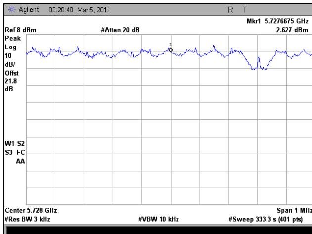
Plot 350. Peak Power Spectral Density, Low Channel, 802.11n HT5, Port 2
