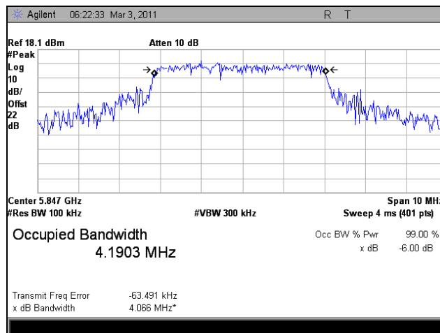
Plot 18. 6 dB Occupied Bandwidth, High Channel, 802.11n HT5, Port 2
