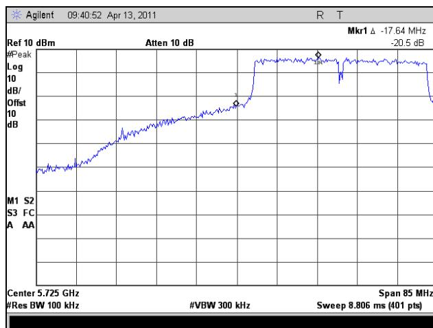
Plot 309. Conducted Band Edge, Low Channel, 802.11a 40 MHz
