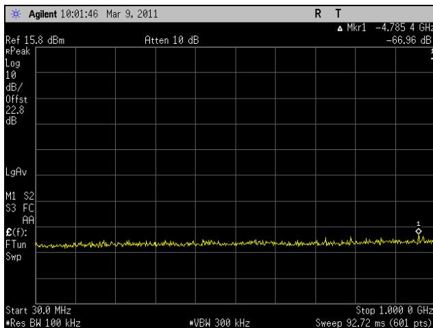
Plot 289. Conducted Spurious Emissions, Low Channel, 30 MHz – 1 GHz, 802.11n HT30, Port 2
