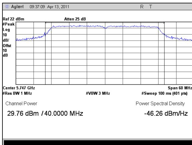
Plot 94. Peak Power Output, Low Channel, 802.11a 40 MHz
