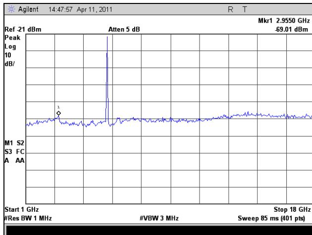
Plot 136. Radiated Spurious Emissions, Mid Channel, 1 GHz – 18 GHz, 802.11a 20 MHz
