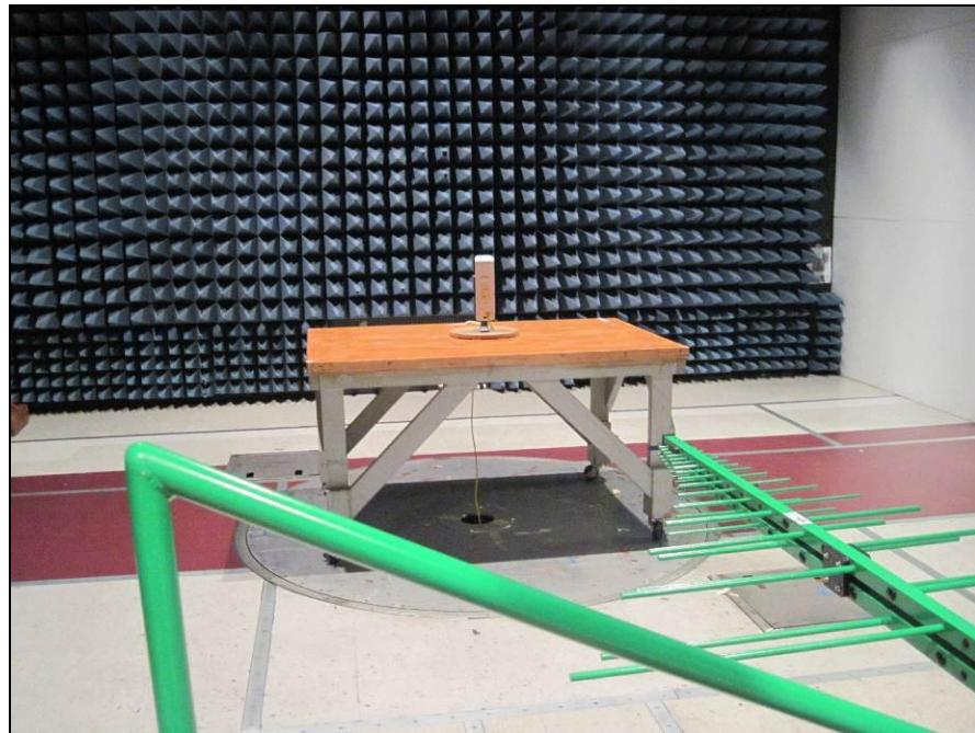
Photograph 6. Radiated Spurious Emissions, Test Setup, 30 MHz – 1 GHz
