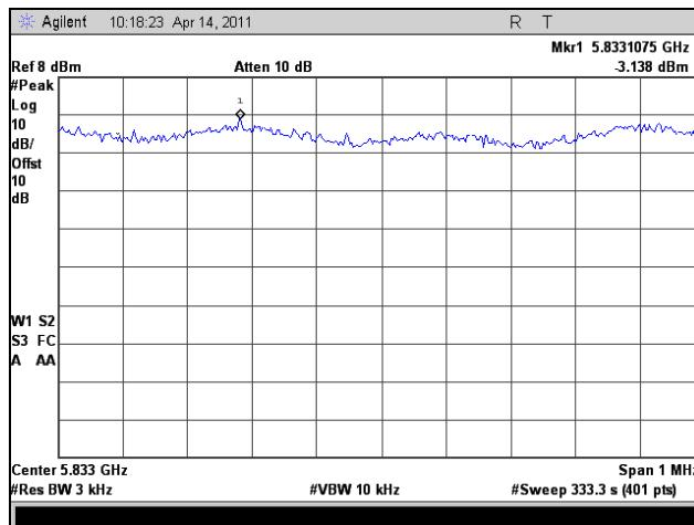
Plot 339. Peak Power Spectral Density, High Channel, Average, 802.11a 20 MHz
