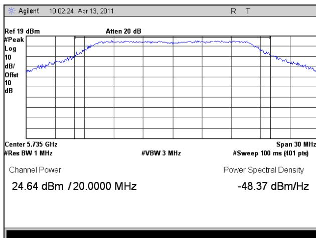
Plot 91. Peak Power Output, Low Channel, 802.11a 20 MHz
