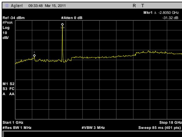
Plot 170. Radiated Spurious Emissions, Low Channel, 1 GHz – 18 GHz, 802.11n HT30
