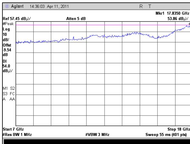
Plot 182. Radiated Harmonics, Low Channel, 7 GHz – 18 GHz, 802.11a 20 MHz
