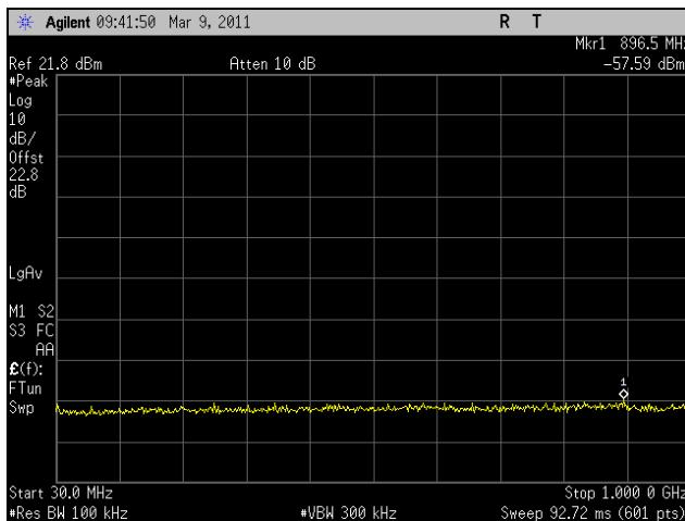
Plot 235. Conducted Spurious Emissions, Low Channel, 30 MHz – 1 GHz, 802.11n HT5, Port 1
