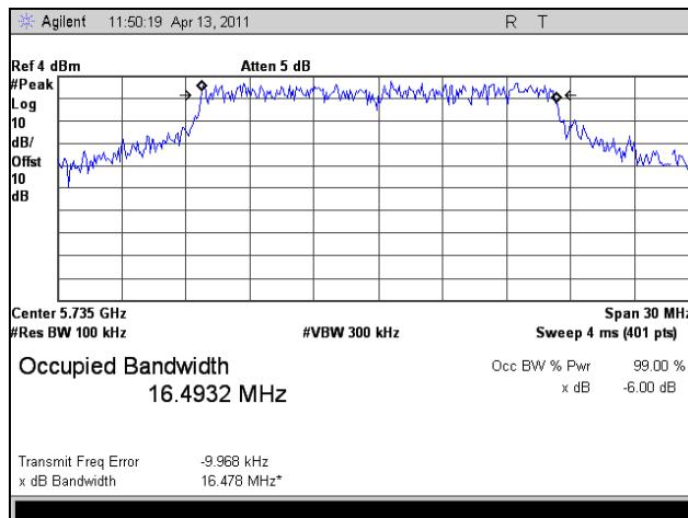
Plot 7. 6 dB Occupied Bandwidth, Low Channel, 802.11a 20MHz
