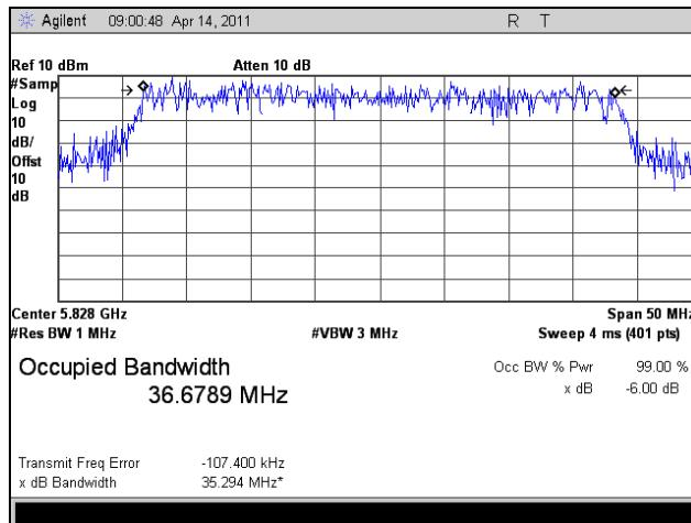
Plot 54. 99% Occupied Bandwidth, High Channel, 802.11a 40 MHz
