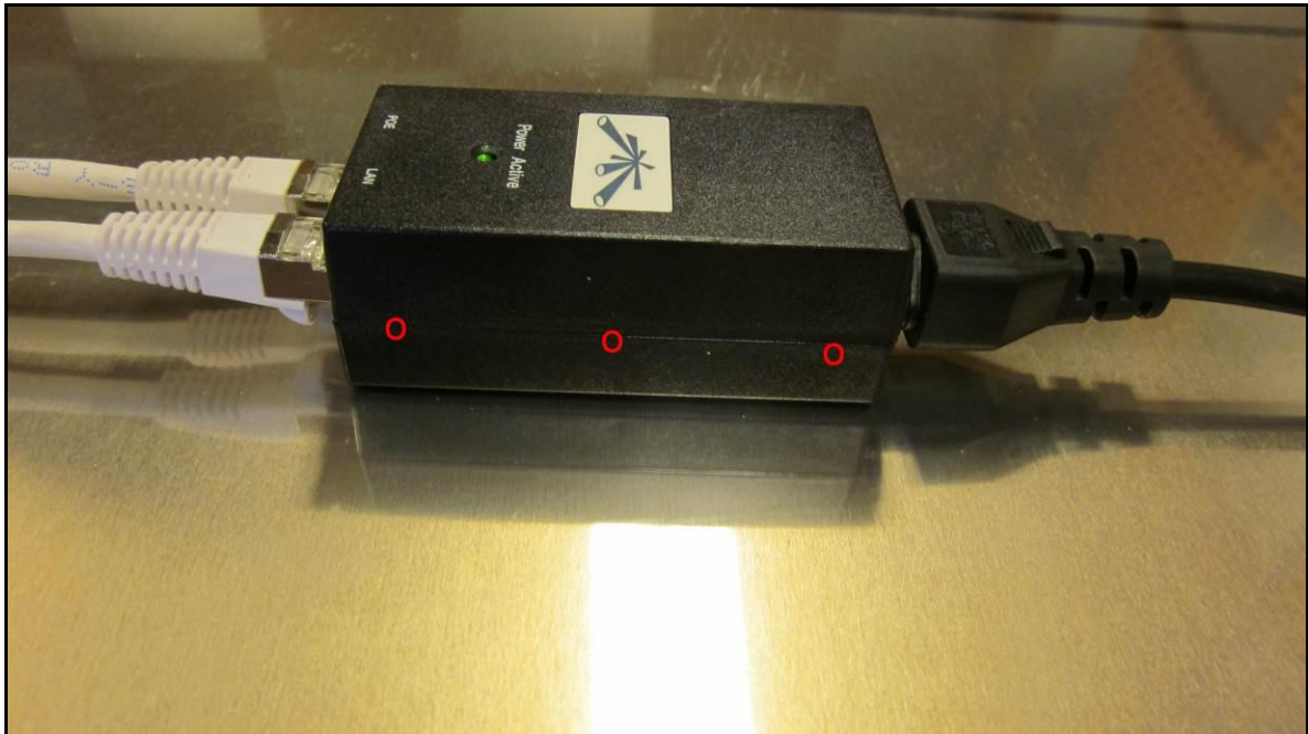
Photograph 13. ESD, Test Points, POE Left View
