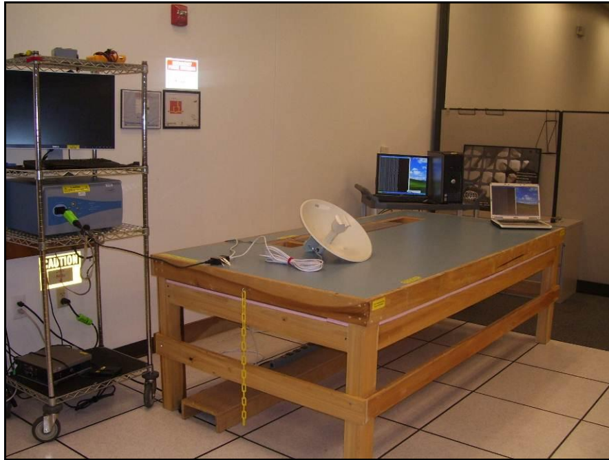
Photograph 17. Fast Transient, Common Mode, Test Setup
