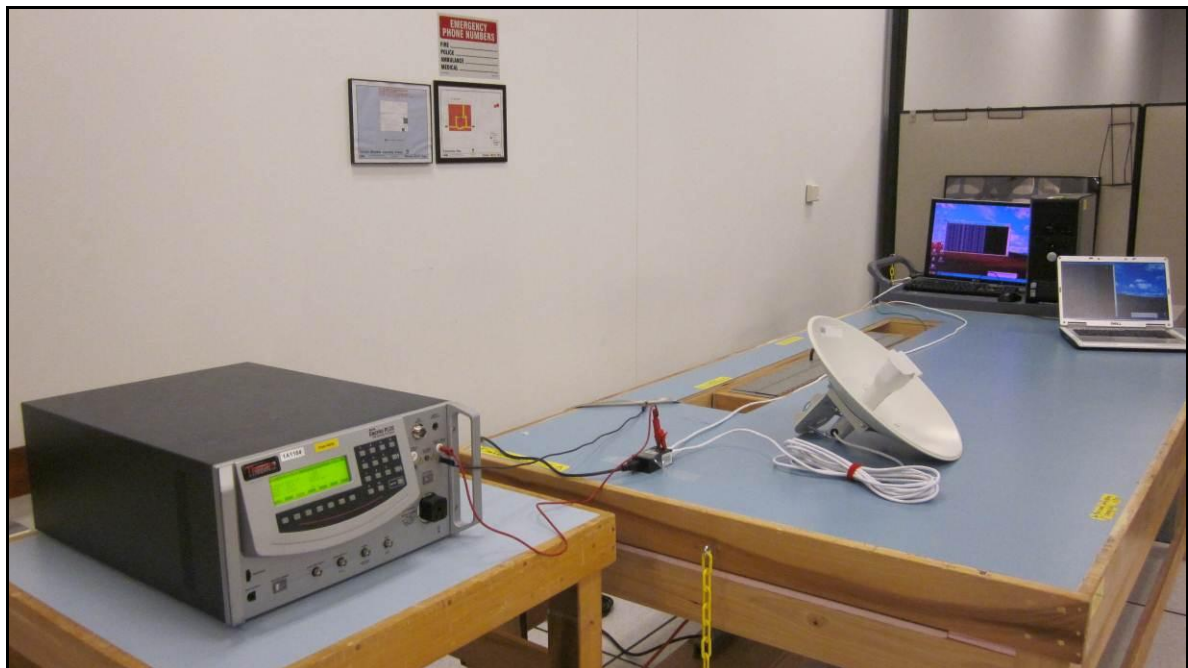
Photograph 23. Surges, I/O Setup
