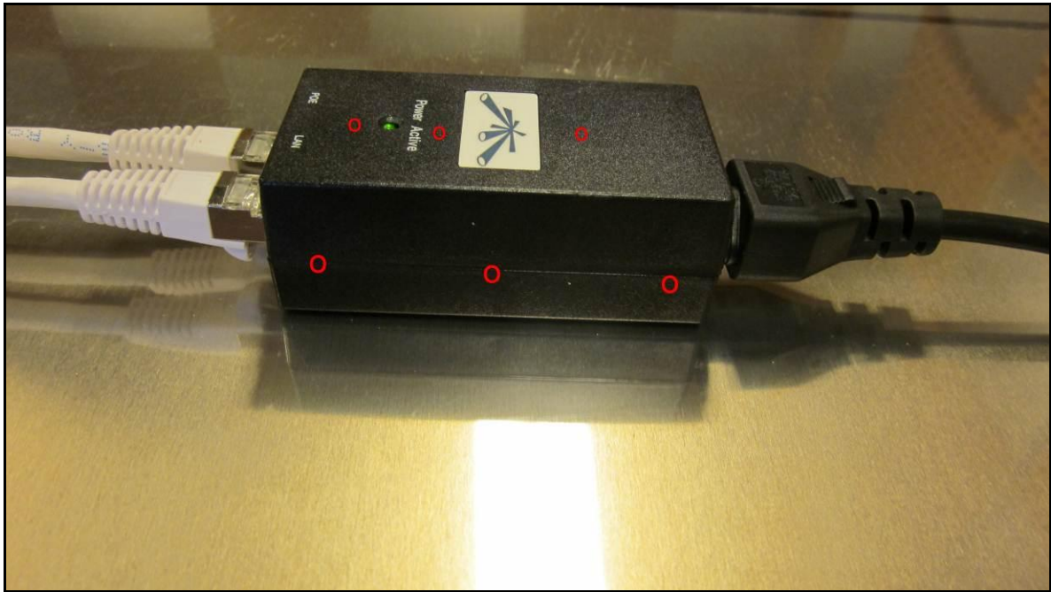
Photograph 11. ESD, Test Points, POE Left Top View
