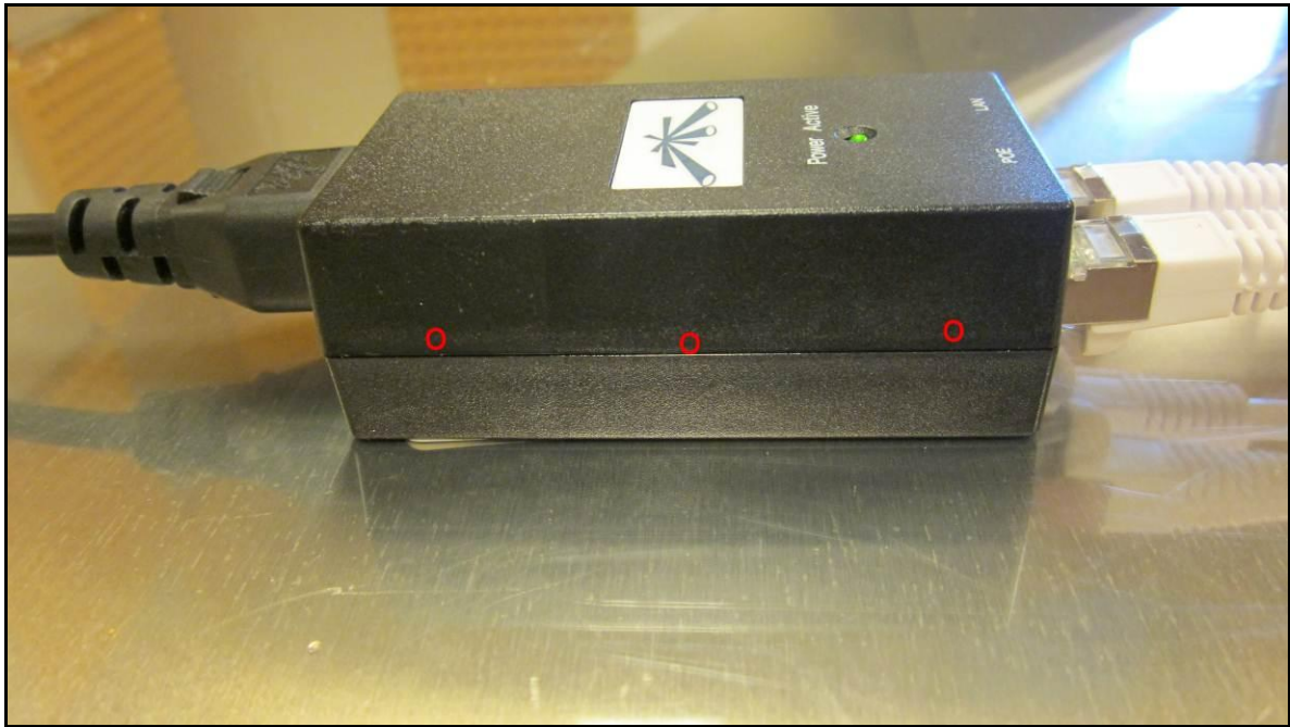
Photograph 15. ESD, Test Points, POE Right View
