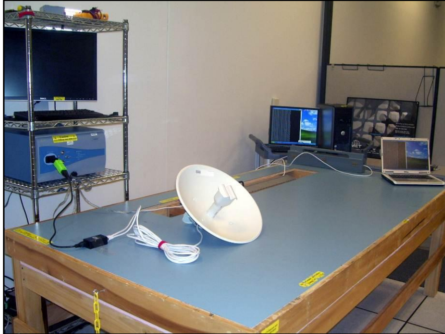
Photograph 22. Surges, AC power Test Setup
