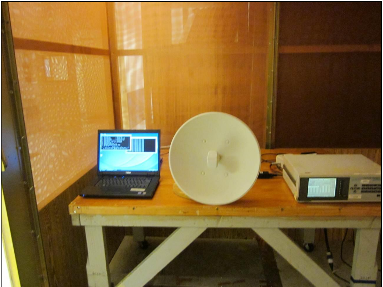
Photograph 3. Voltage Fluctuations (Flicker), Test Setup
