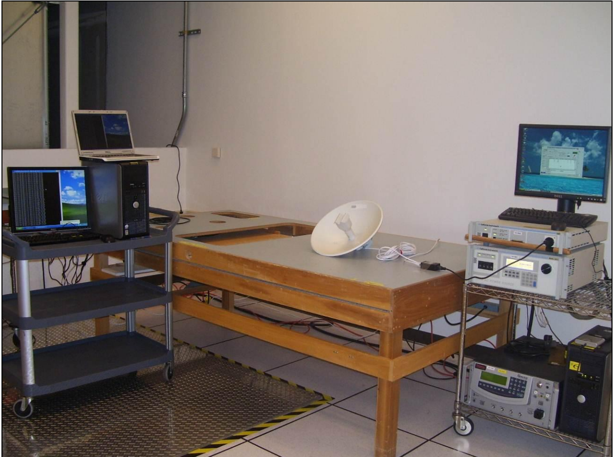
Photograph 21. Voltage Dips and Interruptions, Test Setup
