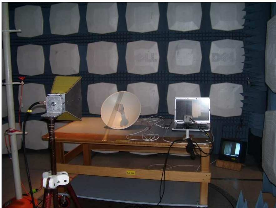
Photograph 6. Radio Frequency Electromagnetic Field, Test Setup, 1.4 GHz – 2.7 GHz
