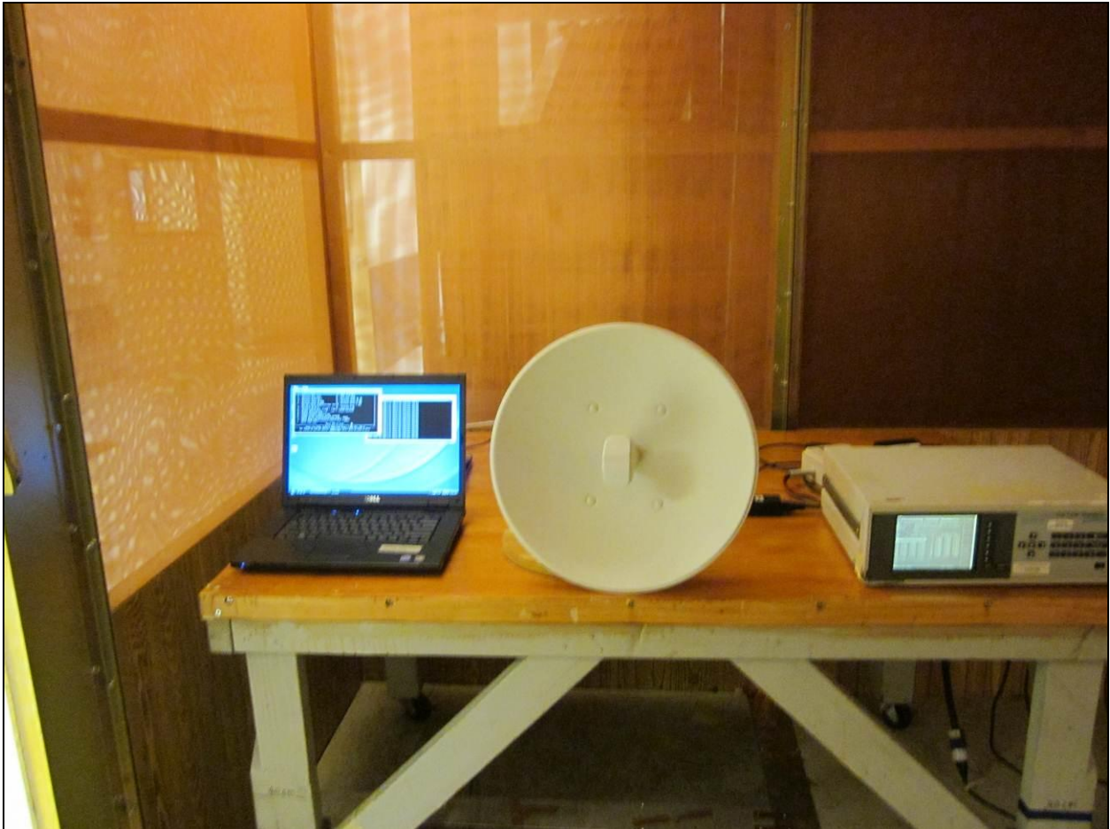
Photograph 2. Harmonic Current Emissions, Test Setup
