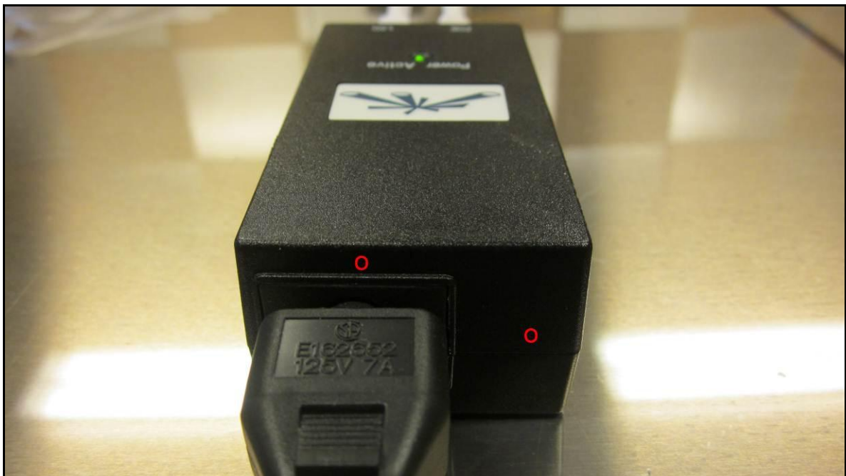
Photograph 14. ESD, Test Points, POE Rear View
