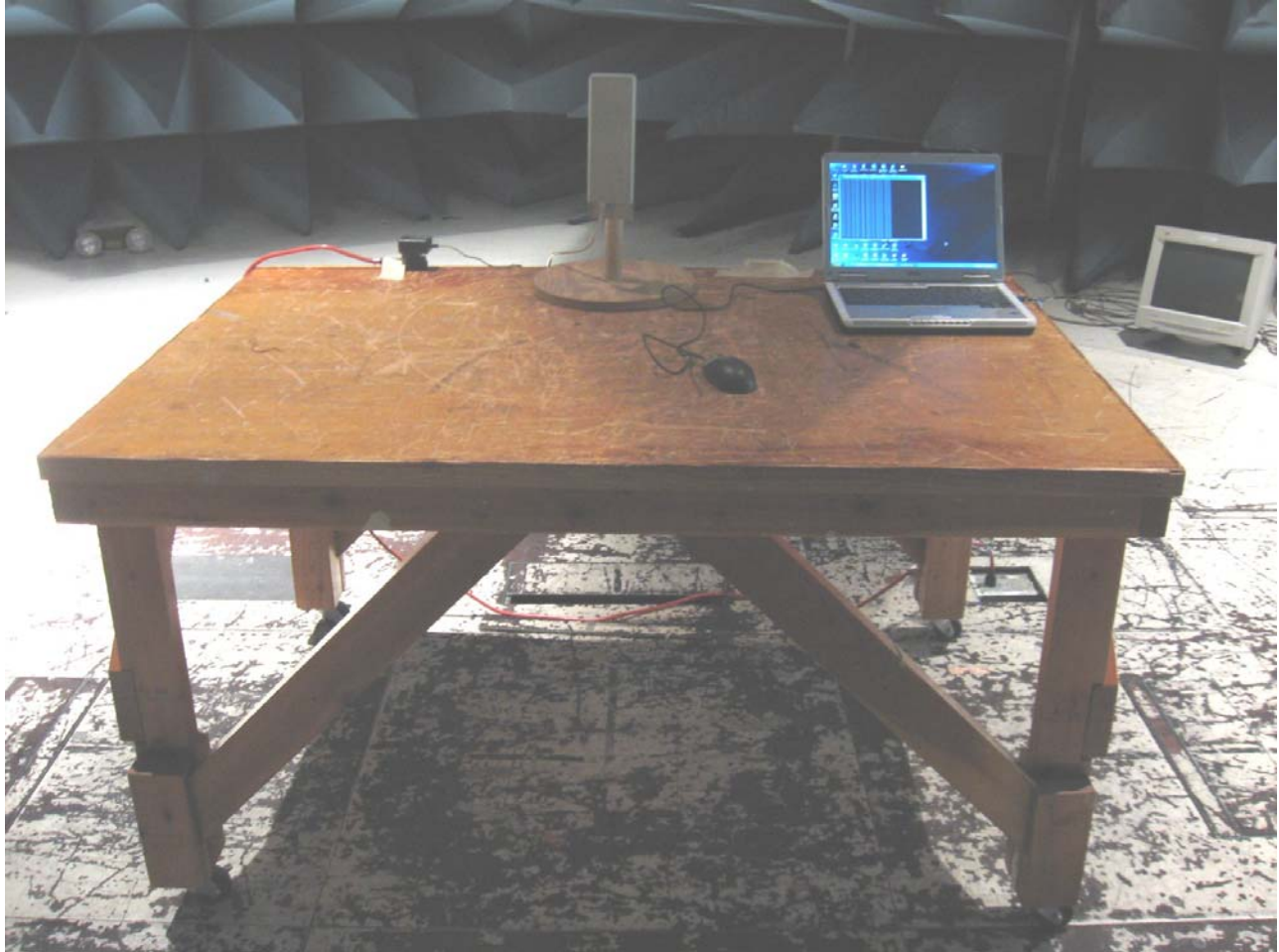
Photograph 3. Radiated Emission Test Setup 30 MHz - 2 GHz
