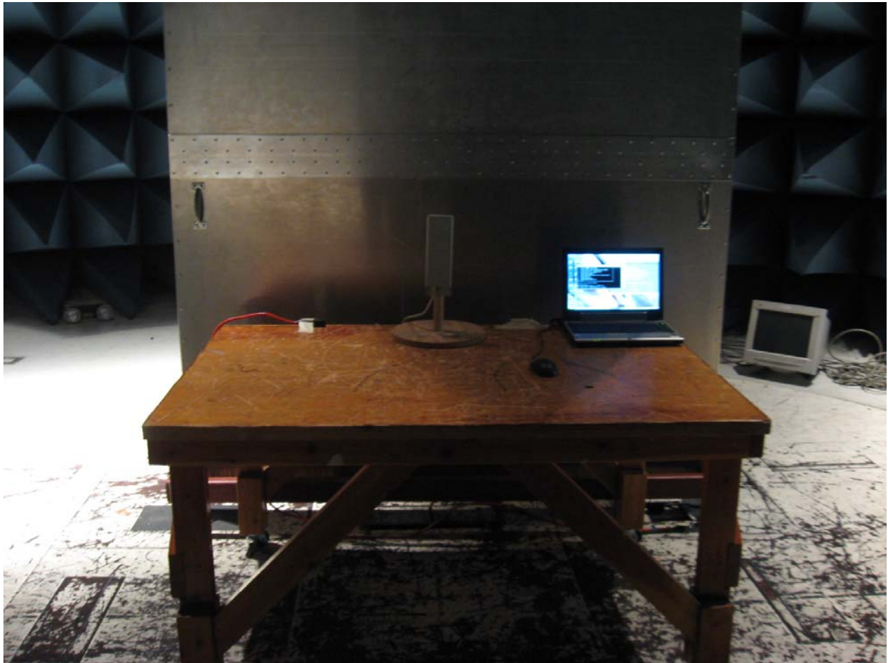
Photograph 4. Conducted Emissions Test Setup
