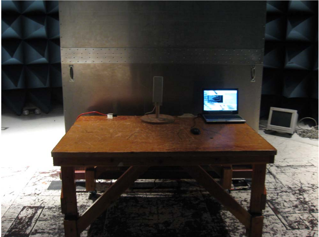
Photograph 2. Conducted Emissions Test Setup
