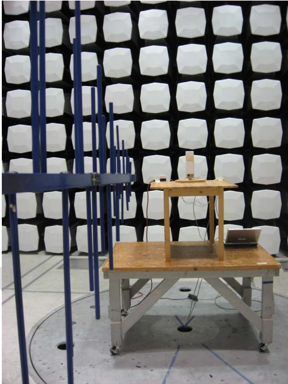
Photograph 2. Radiated Emissions Setup, 30MHz – 1GHz
