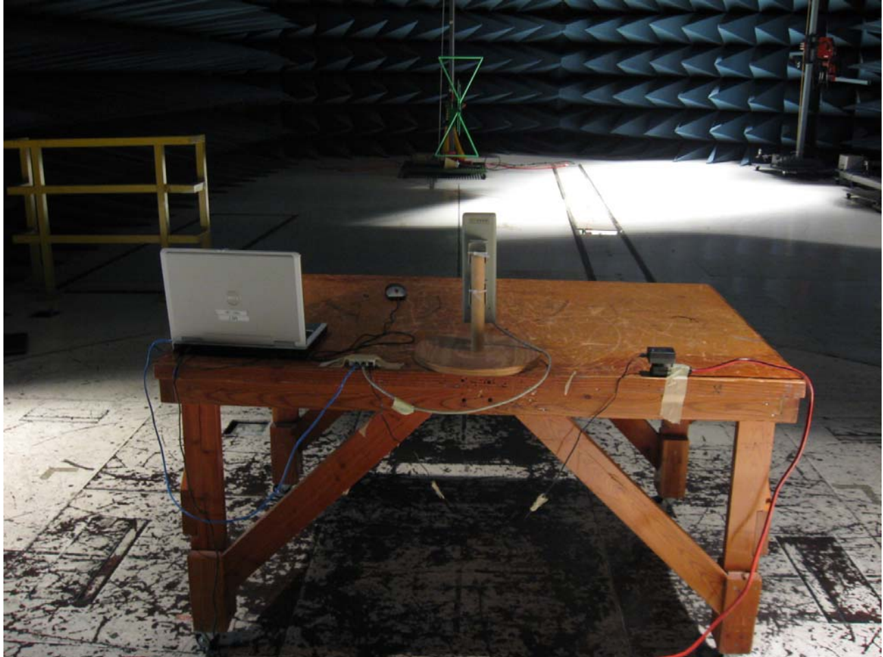
Photograph 3. Radiated Emission Test Setup 30 MHz - 2 GHz
