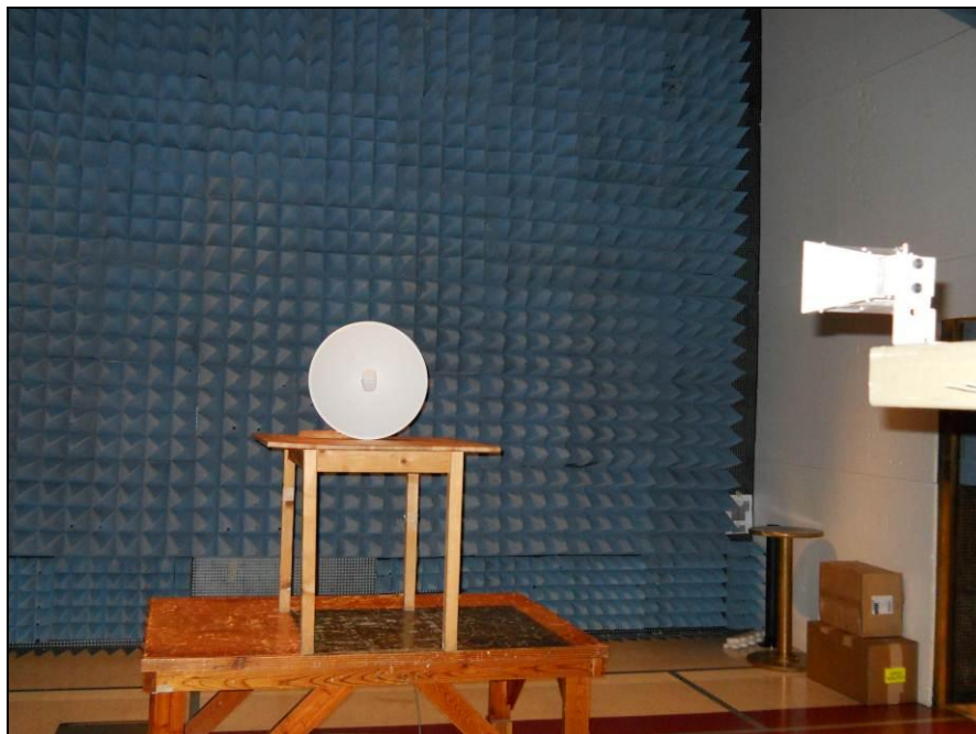
Photograph 4. Transmitter Radiated Emissions, Test Setup 3
