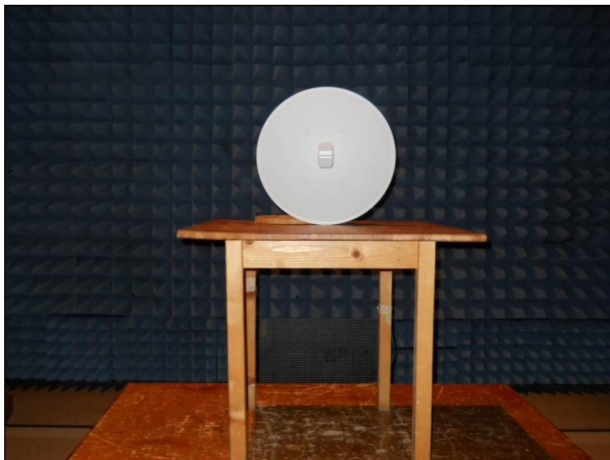
Photograph 3. Transmitter Radiated Emissions, Test Setup 2
