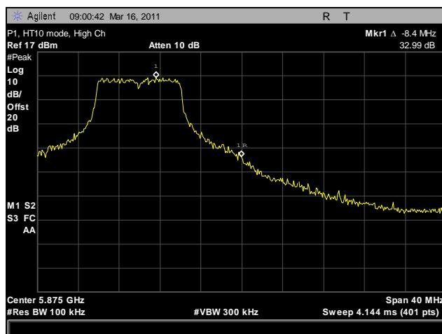
Plot 140. Conducted Spurious Emissions, High Channel, HT10, P1, 20 dBc
