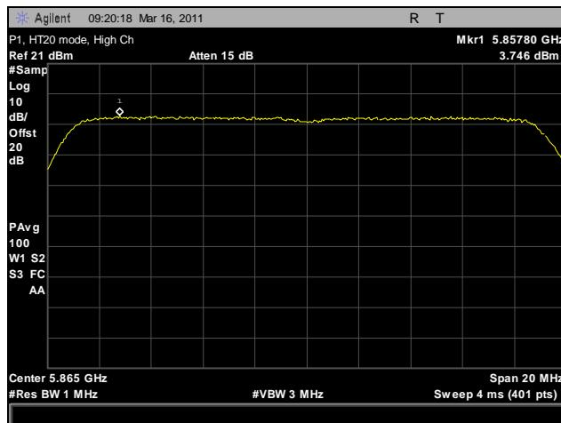
Plot 160. Peak Power Spectral Density, High Channel, HT20, Port 1
