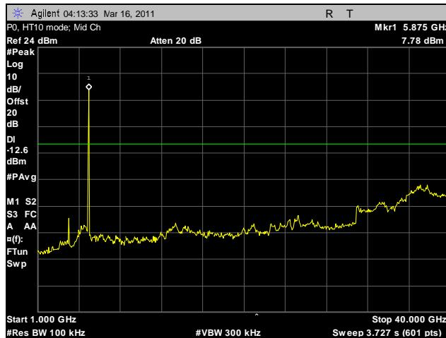
Plot 113. Conducted Spurious Emissions, Mid Channel, HT10, 1 GHz – 40 GHz, Port 0
