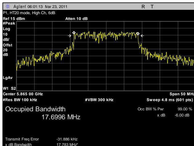
Plot 28. 6 dB Occupied Bandwidth, High Channel, HT20, Port 1
