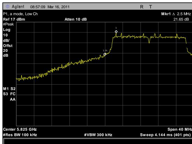
Plot 131. Conducted Spurious Emissions, Low Channel, a Mode, P0, 20 dBc
