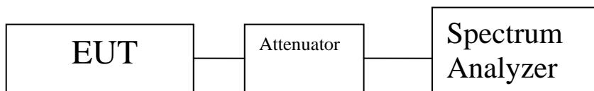
**Figure 2. Block Diagram, Occupied Bandwidth Test Setup**
