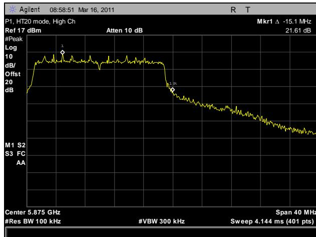
**Plot 142. Conducted Spurious Emissions, High Channel, HT20, P1, 20 dBc**
