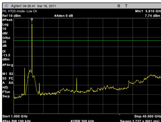
Plot 117. Conducted Spurious Emissions, Low Channel, HT20, 1 GHz – 40 GHz, Port 0
