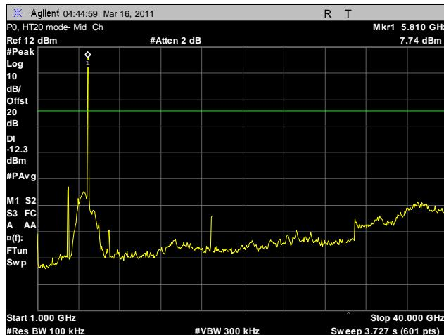
Plot 119. Conducted Spurious Emissions, Mid Channel, HT20, 1 GHz – 40 GHz, Port 0
