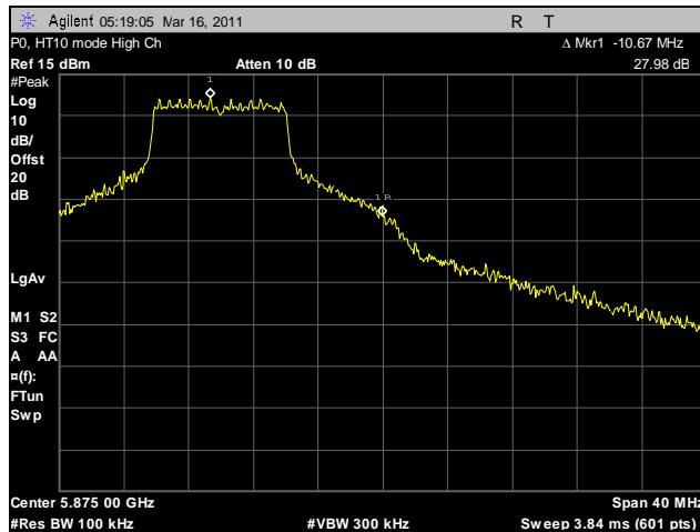
**Plot 134. Conducted Spurious Emissions, High Channel, HT10, P0, 20 dBc**
