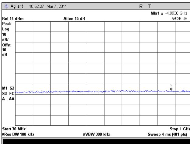
Plot 265. Conducted Spurious Emissions, High Channel, 30 MHz – 1 GHz, 802.11n HT8, Port 1
