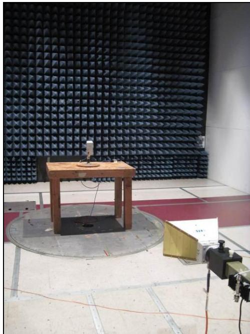
Photograph 6. Radiated Spurious Emissions, Test Setup, 1 GHz – 18 GHz
