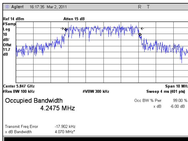
Plot 66. 99% Occupied Bandwidth, High Channel, 802.11n HT5, Port 2
