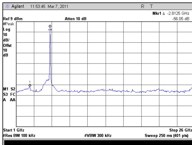
Plot 341. Conducted Spurious Emissions, Low Channel, 1 GHz – 26 GHz, 802.11n HT40, Port 2
