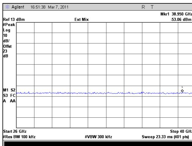
Plot 243. Conducted Spurious Emissions, Low Channel, 26 GHz – 40 GHz, 802.11n HT5, Port 1
