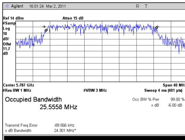
Plot 89. 99% Occupied Bandwidth, Mid Channel, 802.11n HT30, Port 2
