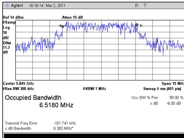
Plot 72. 99% Occupied Bandwidth, High Channel, 802.11n HT8, Port 2
