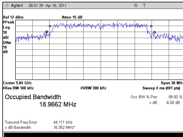
Plot 15. 6 dB Occupied Bandwidth, 802.11a 20 MHz, High Channel
