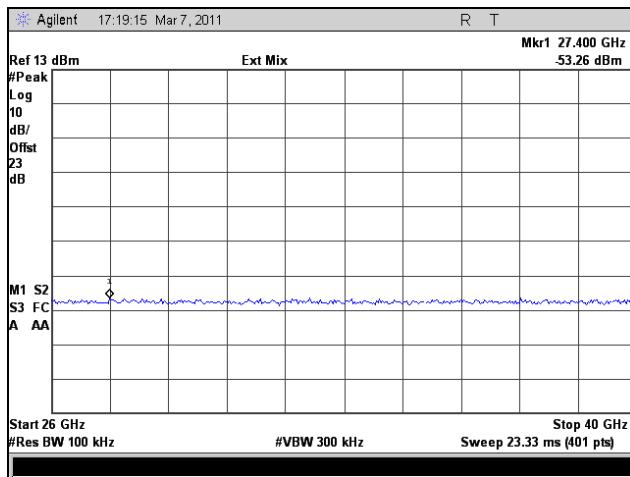
**Plot 273. Conducted Spurious Emissions, Mid Channel, 26 GHz – 40 GHz, 802.11n HT8, Port 2**
