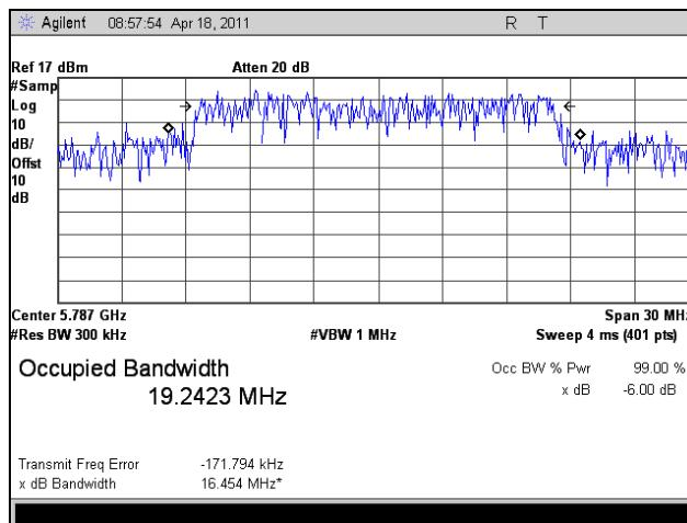
Plot 56. 99% Occupied Bandwidth, 802.11a 20 MHz, Mid Channel
