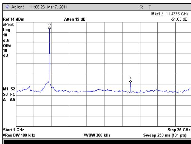
Plot 278. Conducted Spurious Emissions, Low Channel, 1 GHz – 26 GHz, 802.11n HT10, Port 1
