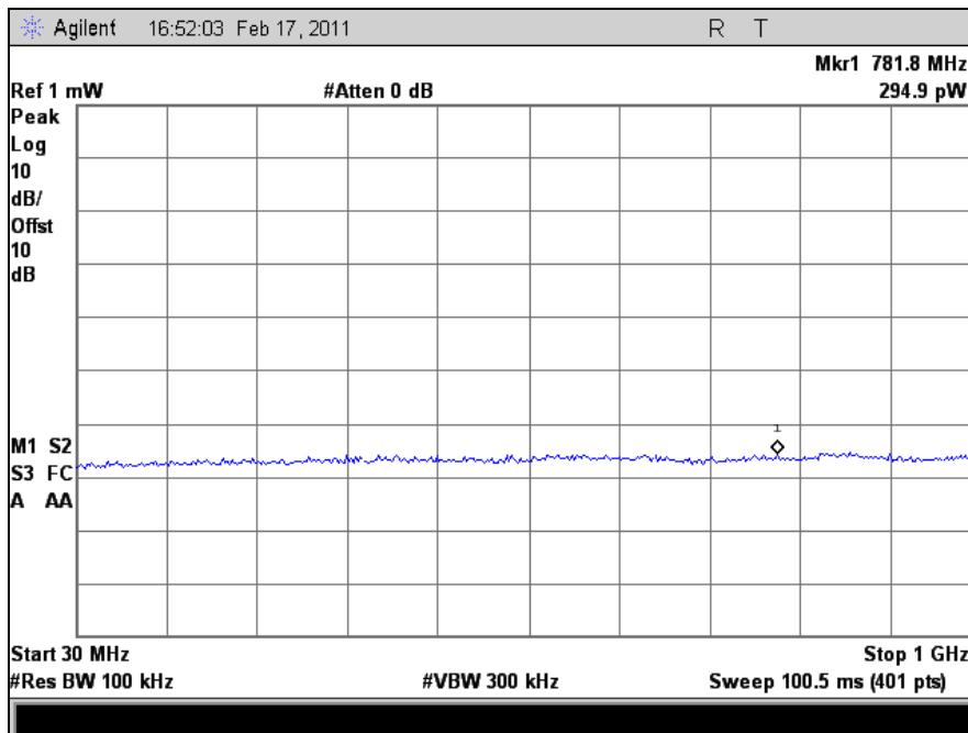
Plot 419. Receiver Spurious Emission, 30 MHz – 1 GHz, Port 1
