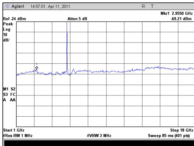
Plot 142. Radiated Spurious Emissions, 802.11a 20 MHz, Mid Channel, 1 GHz – 18 GHz
