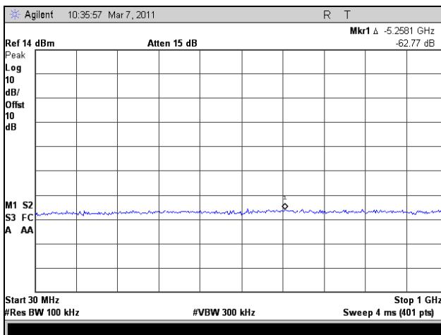
Plot 247. Conducted Spurious Emissions, High Channel, 30 MHz – 1 GHz, 802.11n HT5, Port 1
