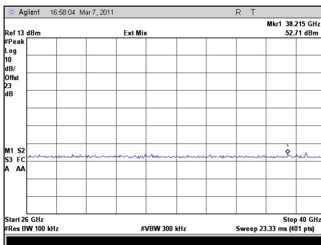
Plot 285. Conducted Spurious Emissions, High Channel, 26 GHz – 40 GHz, 802.11n HT10, Port 1
