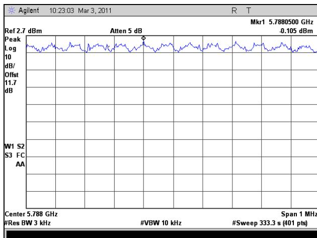
Plot 385. Peak Power Spectral Density, Mid Channel, 802.11n HT5, Port 1
