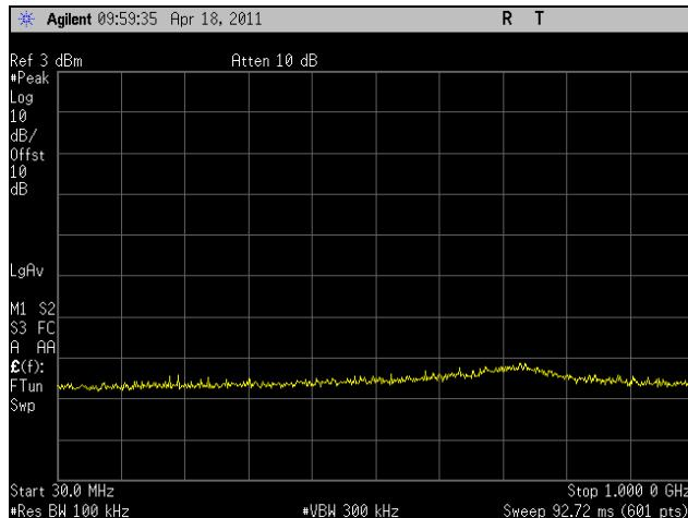
Plot 229. Conducted Spurious Emissions, Low Channel, 802.11a 20 MHz, 30 MHz – 1 GHz
