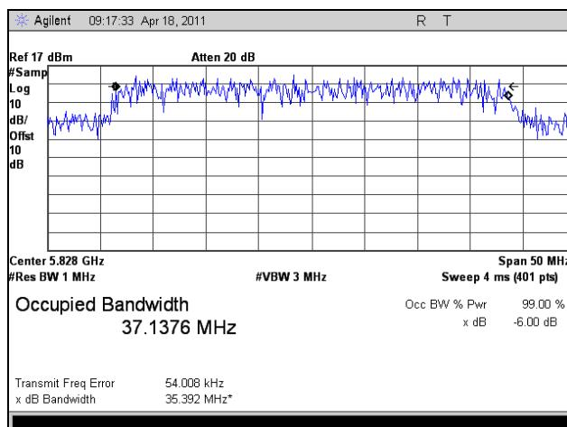
Plot 60. 99% Occupied Bandwidth, 802.11a 40 MHz, High Channel
