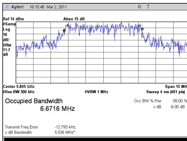
Plot 69. 99% Occupied Bandwidth, High Channel, 802.11n HT8, Port 1
