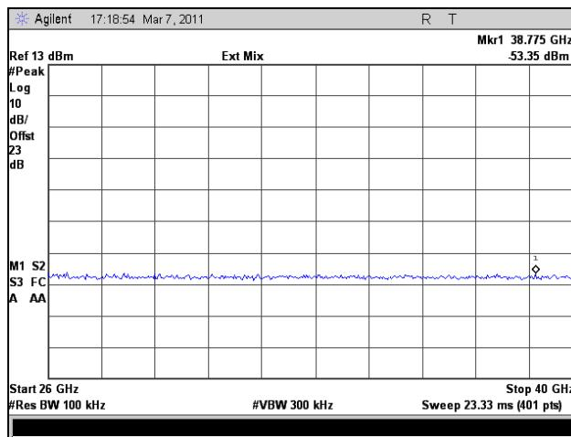
Plot 270. Conducted Spurious Emissions, Low Channel, 26 GHz – 40 GHz, 802.11n HT8, Port 2
