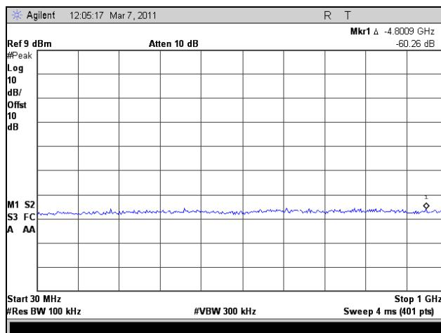
Plot 340. Conducted Spurious Emissions, Low Channel, 30 MHz – 1 GHz, 802.11n HT40, Port 2
