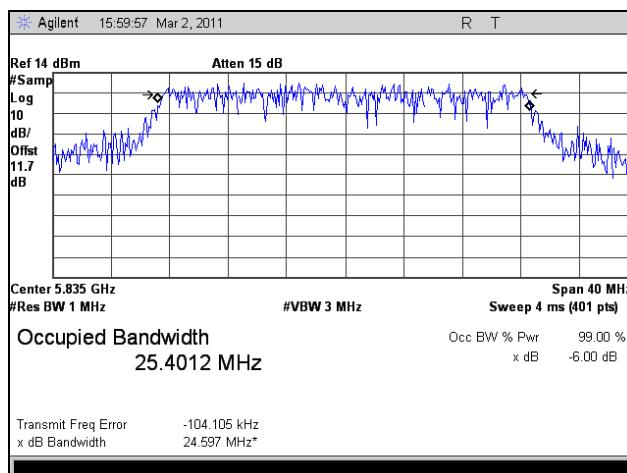
Plot 90. 99% Occupied Bandwidth, High Channel, 802.11n HT30, Port 2
