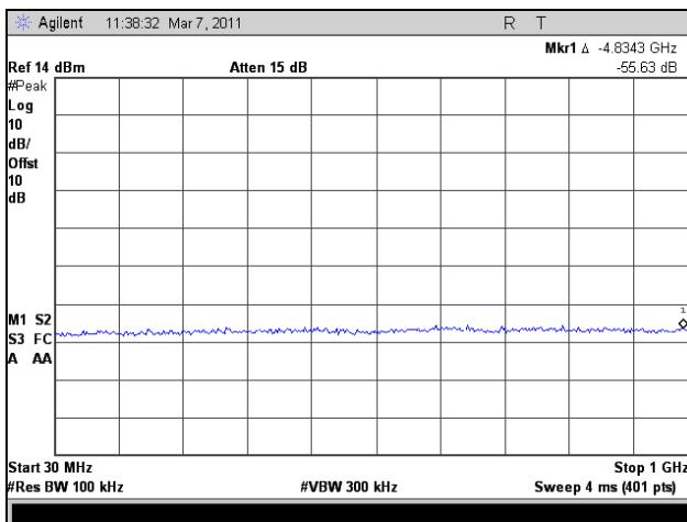
Plot 319. Conducted Spurious Emissions, High Channel, 30 MHz – 1 GHz, 802.11n HT30, Port 1
