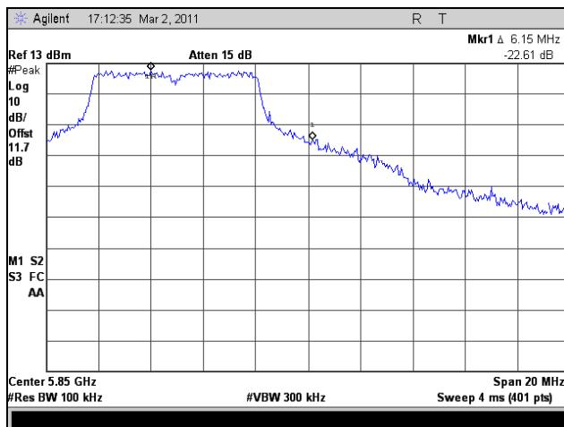
Plot 358. Conducted Band Edge, High Channel, 802.11n HT8, Port 1
