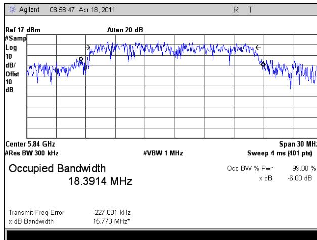
Plot 57. 99% Occupied Bandwidth, 802.11a 20 MHz, High Channel
