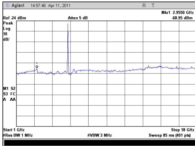
Plot 144. Radiated Spurious Emissions, 802.11a 20 MHz, High Channel, 1 GHz – 18 GHz
