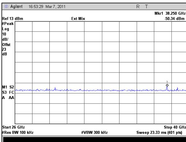
Plot 249. Conducted Spurious Emissions, High Channel, 26 GHz – 40 GHz, 802.11n HT5, Port 1
