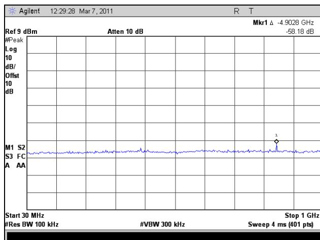
Plot 304. Conducted Spurious Emissions, Low Channel, 30 MHz – 1 GHz, 802.11n HT20, Port 2
