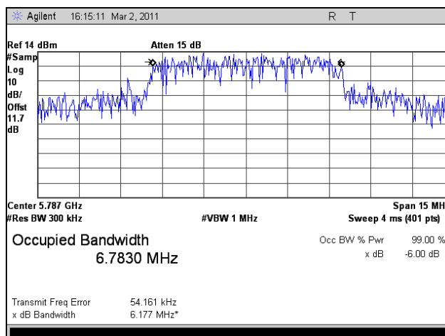
Plot 68. 99% Occupied Bandwidth, Mid Channel, 802.11n HT8, Port 1
