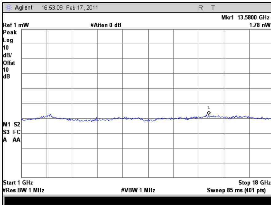
Plot 420. Receiver Spurious Emission, 1 GHz – 18 GHz, Port 1
