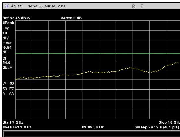
Plot 219. Radiated Harmonics, Mid Channel, 7 GHz – 18 GHz, Average, 802.11n HT30
