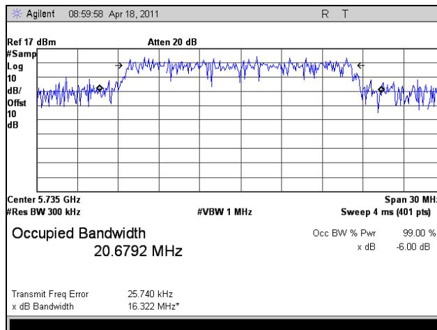
Plot 55. 99% Occupied Bandwidth, 802.11a 20 MHz, Low Channel
