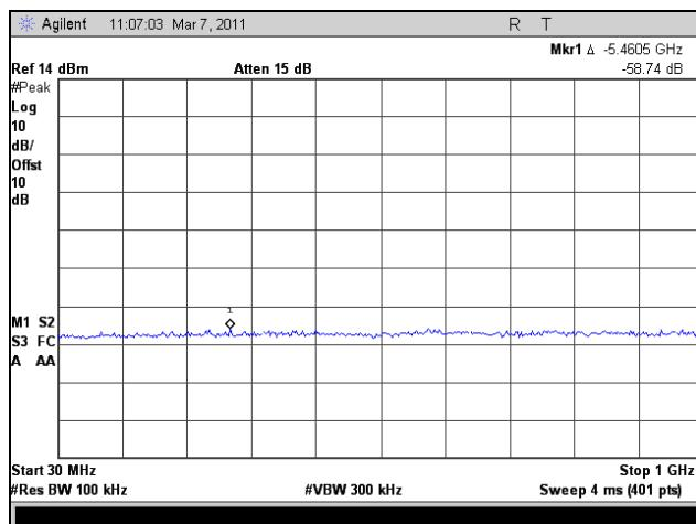
Plot 277. Conducted Spurious Emissions, Low Channel, 30 MHz – 1 GHz, 802.11n HT10, Port 1
