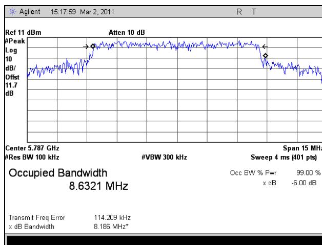
Plot 32. 6 dB Occupied Bandwidth, Mid Channel, 802.11n HT10, Port 1
