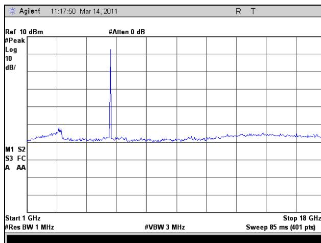
**Plot 168.** Radiated Spurious Emissions, High Channel, 1 GHz – 18 GHz, 802.11n HT10
