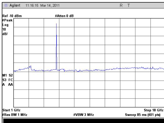
Plot 160. Radiated Spurious Emissions, Mid Channel, 1 GHz – 18 GHz, 802.11n HT8
