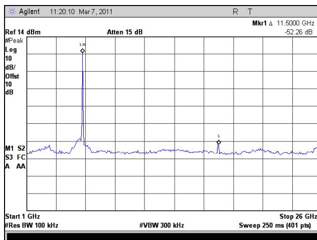
Plot 296. Conducted Spurious Emissions, Low Channel, 1 GHz – 26 GHz, 802.11n HT20, Port 1
