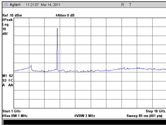
Plot 174. Radiated Spurious Emissions, High Channel, 1 GHz – 18 GHz, 802.11n HT20
