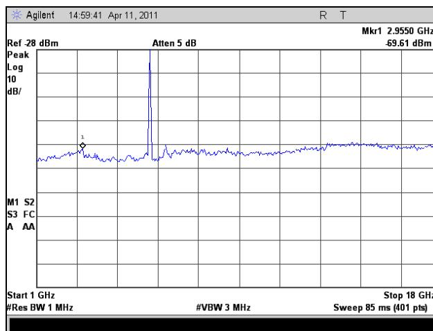
Plot 146. Radiated Spurious Emissions, 802.11a 40 MHz, Low Channel, 1 GHz – 18 GHz
