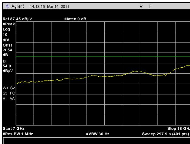
**Plot 221. Radiated Harmonics, High Channel, 7 GHz – 18 GHz, Average, 802.11n HT30**
