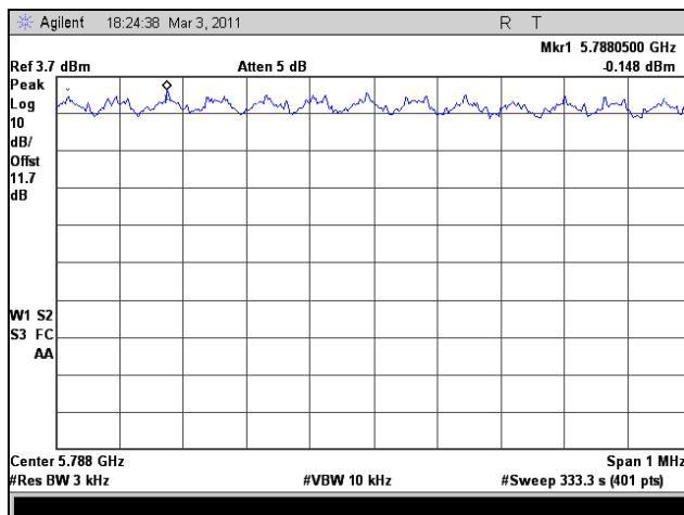
**Plot 386. Peak Power Spectral Density, Mid Channel, 802.11n HT5, Port 2**
