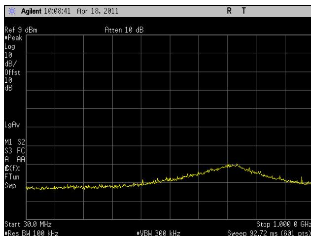
Plot 231. Conducted Spurious Emissions, Mid Channel, 802.11a 20 MHz, 30 MHz – 1 GHz
