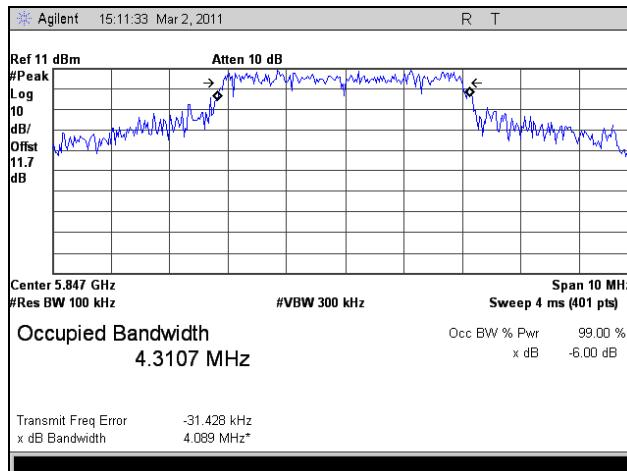
Plot 21. 6 dB Occupied Bandwidth, High Channel, 802.11n HT5, Port 1
