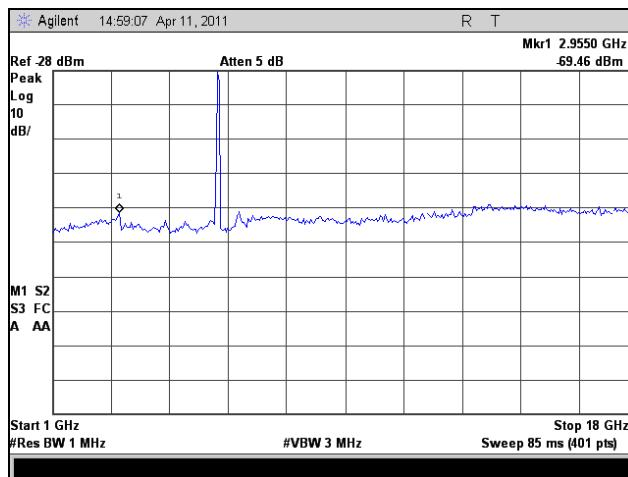
Plot 148. Radiated Spurious Emissions, 802.11a 40 MHz, Mid Channel, 1 GHz – 18 GHz
