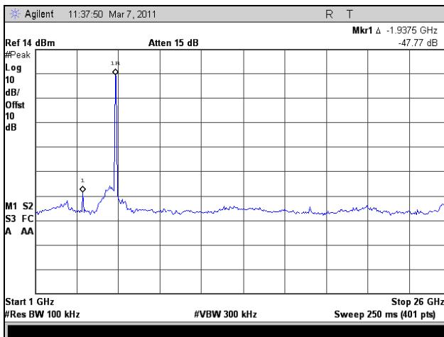
Plot 320. Conducted Spurious Emissions, High Channel, 1 GHz – 26 GHz, 802.11n HT30, Port 1
