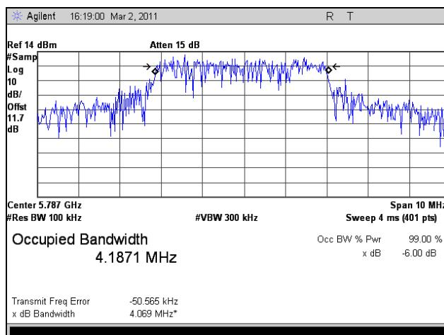
Plot 65. 99% Occupied Bandwidth, Mid Channel, 802.11n HT5, Port 2
