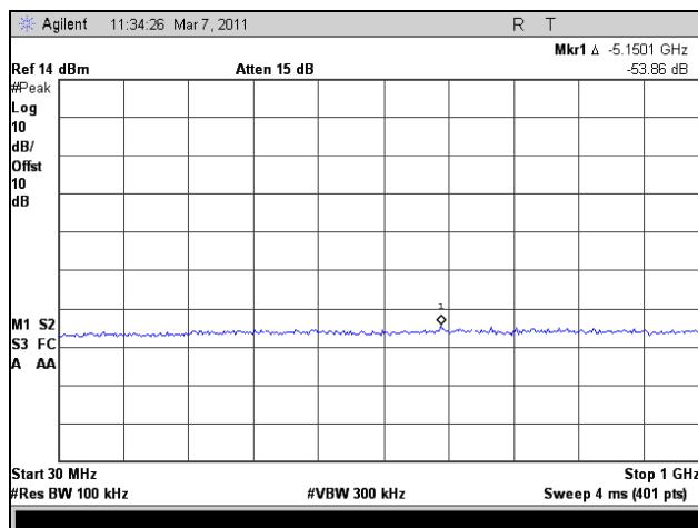
Plot 313. Conducted Spurious Emissions, Low Channel, 30 MHz – 1 GHz, 802.11n HT30, Port 1
