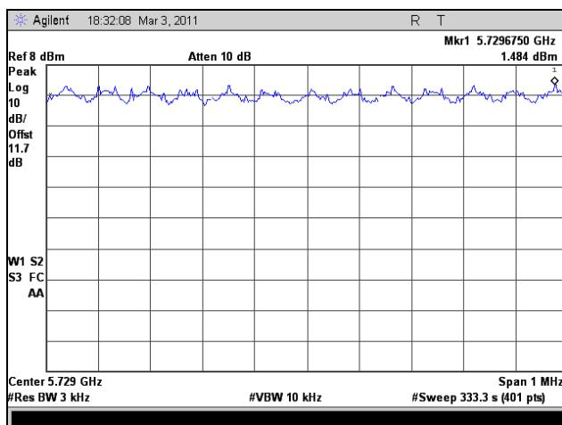
Plot 384. Peak Power Spectral Density, Low Channel, 802.11n HT5, Port 2
