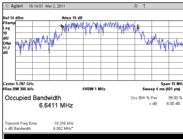
Plot 71. 99% Occupied Bandwidth, Mid Channel, 802.11n HT8, Port 2
