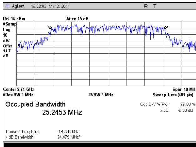
Plot 88. 99% Occupied Bandwidth, Low Channel, 802.11n HT30, Port 2
