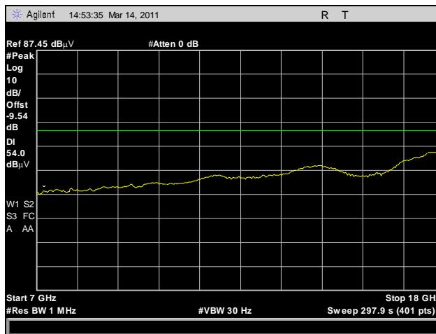
**Plot 215. Radiated Harmonics, High Channel, 7 GHz – 18 GHz, Average, 802.11n HT20**
