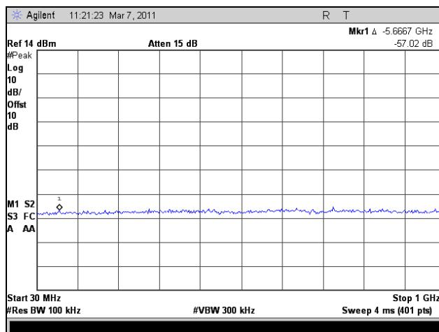
Plot 295. Conducted Spurious Emissions, Low Channel, 30 MHz – 1 GHz, 802.11n HT20, Port 1
