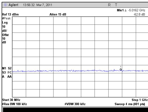
**Plot 271. Conducted Spurious Emissions, Mid Channel, 30 MHz – 1 GHz, 802.11n HT8, Port 2**
