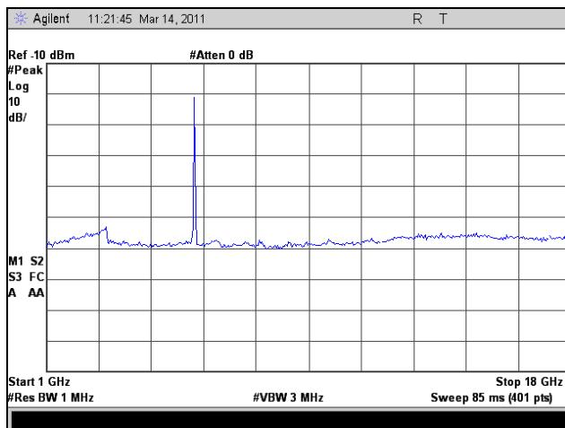
Plot 172. Radiated Spurious Emissions, Mid Channel, 1 GHz – 18 GHz, 802.11n HT20
