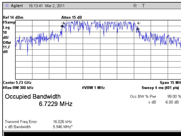
Plot 67. 99% Occupied Bandwidth, Low Channel, 802.11n HT8, Port 1
