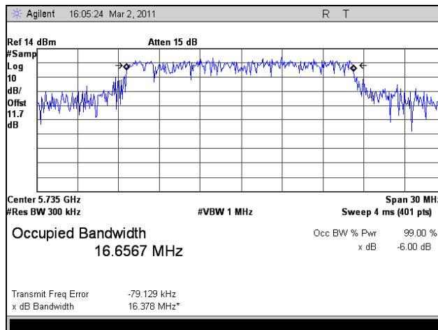
Plot 82. 99% Occupied Bandwidth, Low Channel, 802.11n HT20, Port 2
