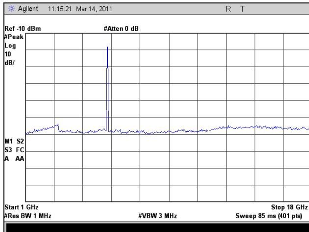
Plot 162. Radiated Spurious Emissions, High Channel, 1 GHz – 18 GHz, 802.11n HT8
