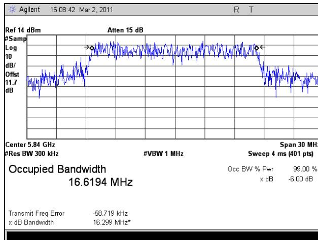
Plot 84. 99% Occupied Bandwidth, High Channel, 802.11n HT20, Port 2
