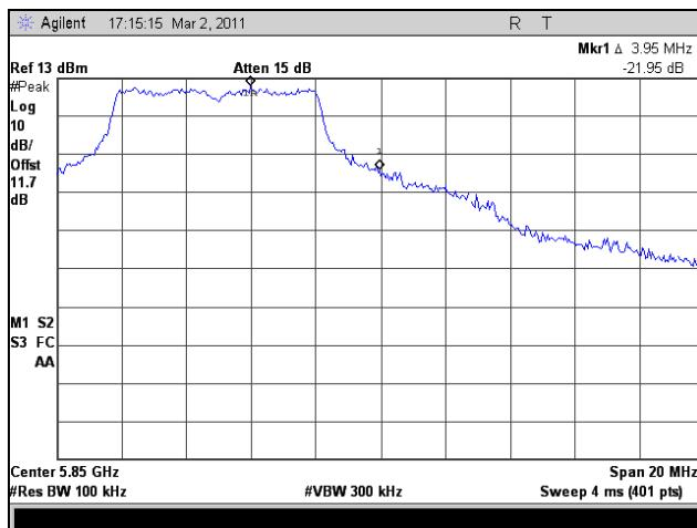
Plot 360. Conducted Band Edge, High Channel, 802.11n HT8, Port 2
