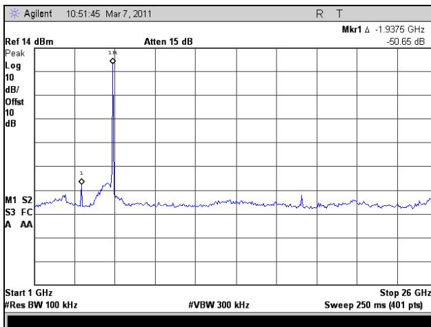
Plot 266. Conducted Spurious Emissions, High Channel, 1 GHz – 26 GHz, 802.11n HT8, Port 1
