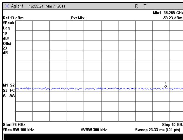
Plot 261. Conducted Spurious Emissions, Low Channel, 26 GHz – 40 GHz, 802.11n HT8, Port 1
