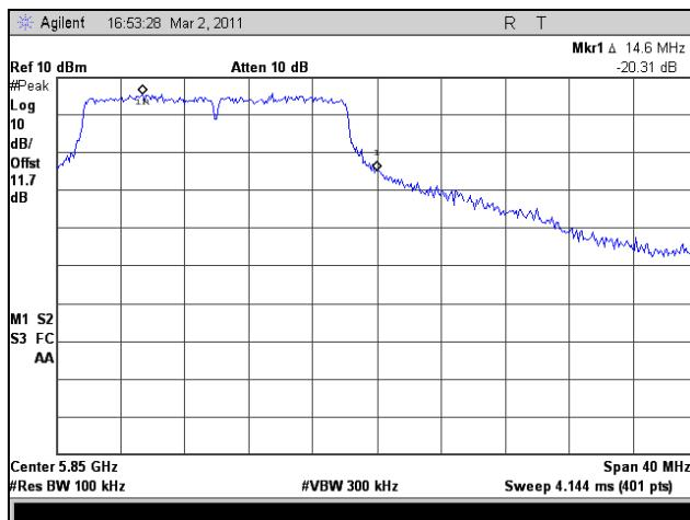
Plot 368. Conducted Band Edge, High Channel, 802.11n HT20, Port 2
