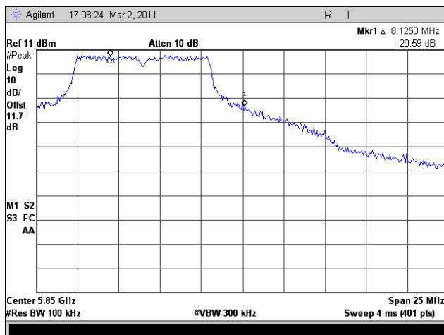
Plot 364. Conducted Band Edge, High Channel, 802.11n HT10, Port 2
