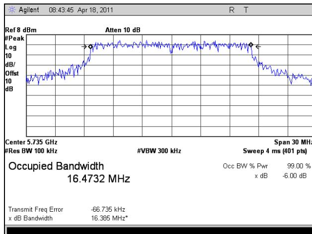
Plot 13. 6 dB Occupied Bandwidth, 802.11a 20 MHz, Low Channel
