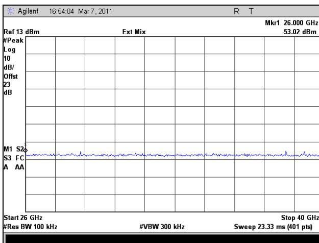
Plot 267. Conducted Spurious Emissions, High Channel, 26 GHz – 40 GHz, 802.11n HT8, Port 1
