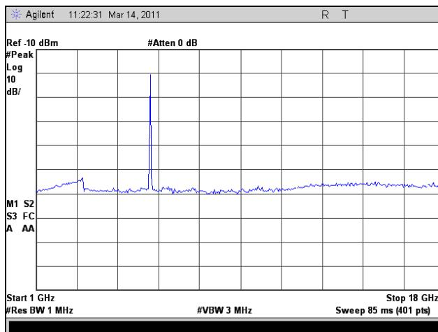
Plot 170. Radiated Spurious Emissions, Low Channel, 1 GHz – 18 GHz, 802.11n HT20
