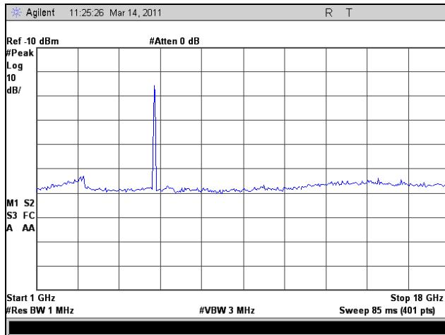
**Plot 186.** Radiated Spurious Emissions, High Channel, 1 GHz – 18 GHz, 802.11n HT40
