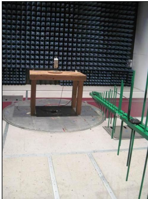
Photograph 5. Radiated Spurious Emissions, Test Setup, 30 MHz – 1 GHz
