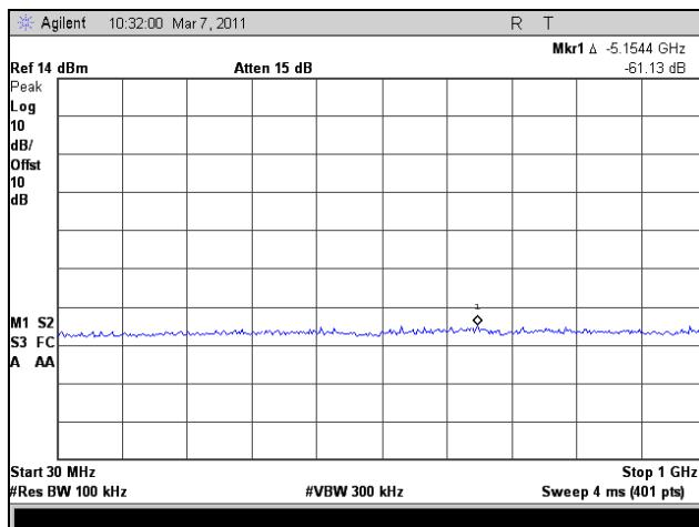
**Plot 244. Conducted Spurious Emissions, Mid Channel, 30 MHz – 1 GHz, 802.11n HT5, Port 1**
