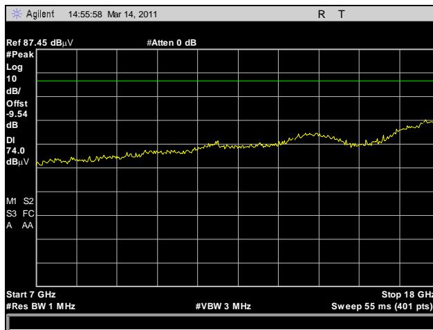
**Plot 210. Radiated Harmonics, High Channel, 7 GHz – 18 GHz, Peak, 802.11n HT10**
