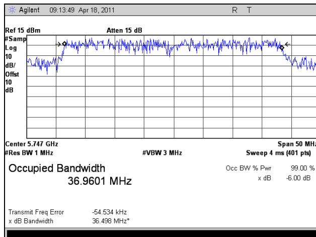
Plot 58. 99% Occupied Bandwidth, 802.11a 40 MHz, Low Channel
