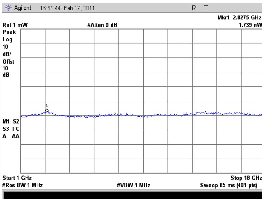
Plot 422. Receiver Spurious Emission, 1 GHz – 18 GHz, Port 2
