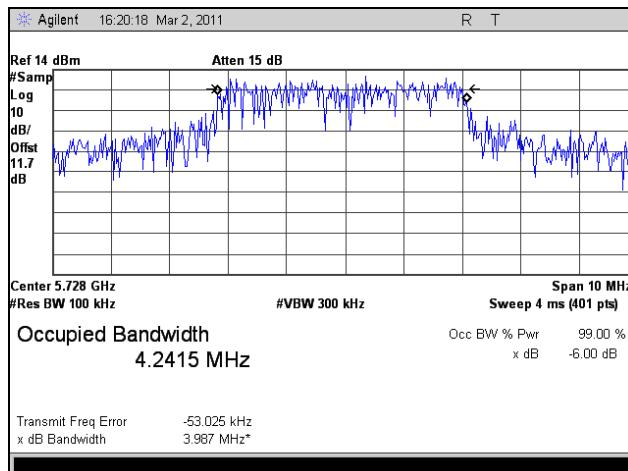
Plot 64. 99% Occupied Bandwidth, Low Channel, 802.11n HT5, Port 2
