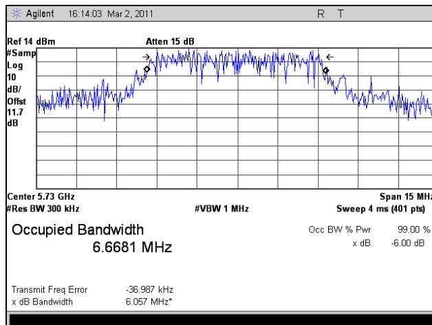
Plot 70. 99% Occupied Bandwidth, Low Channel, 802.11n HT8, Port 2
