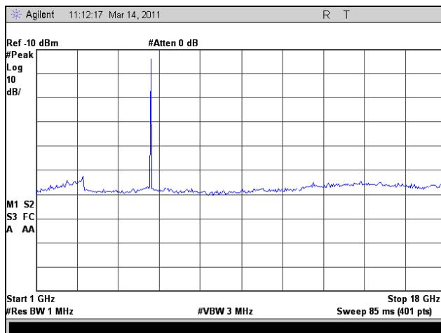
Plot 152. Radiated Spurious Emissions, Low Channel, 1 GHz – 18 GHz, 802.11n HT5
