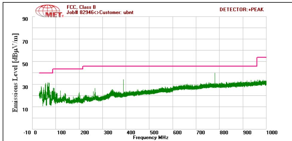
Plot 141. Radiated Spurious Emissions, 802.11a 20 MHz, Mid Channel, 30 MHz – 1 GHz
