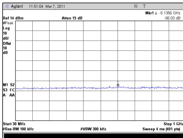
Plot 331. Conducted Spurious Emissions, Low Channel, 30 MHz – 1 GHz, 802.11n HT40, Port 1
