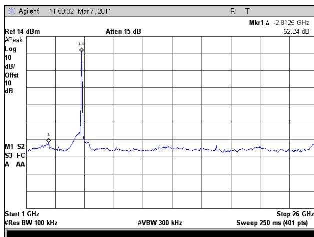
Plot 332. Conducted Spurious Emissions, Low Channel, 1 GHz – 26 GHz, 802.11n HT40, Port 1
