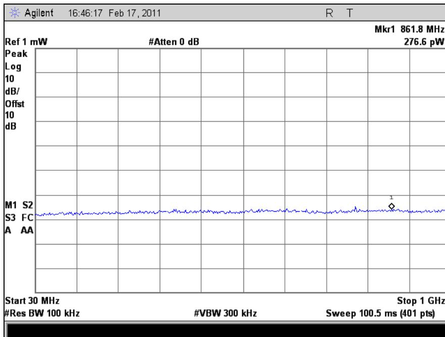
Plot 421. Receiver Spurious Emission, 30 MHz – 1 GHz, Port 2
