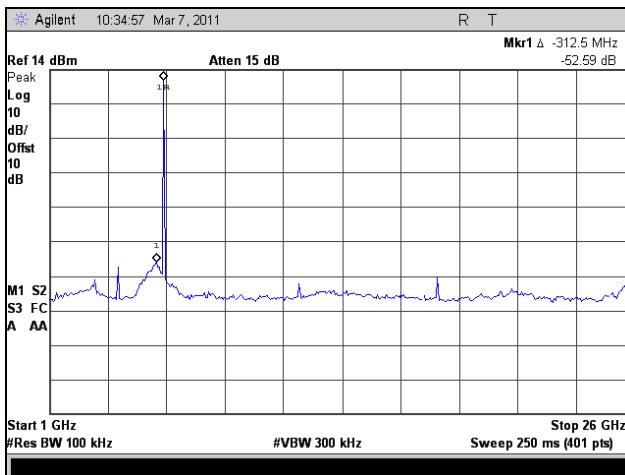
Plot 248. Conducted Spurious Emissions, High Channel, 1 GHz – 26 GHz, 802.11n HT5, Port 1
