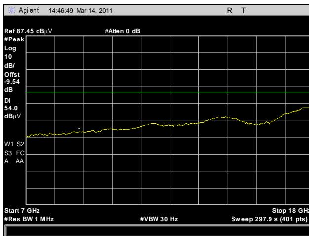
Plot 213. Radiated Harmonics, Mid Channel, 7 GHz – 18 GHz, Average, 802.11n HT20
