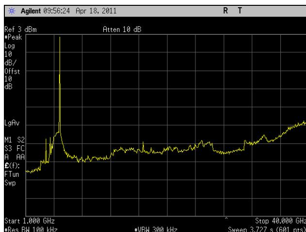
Plot 230. Conducted Spurious Emissions, Low Channel, 802.11a 20 MHz, 1 GHz – 40 GHz
