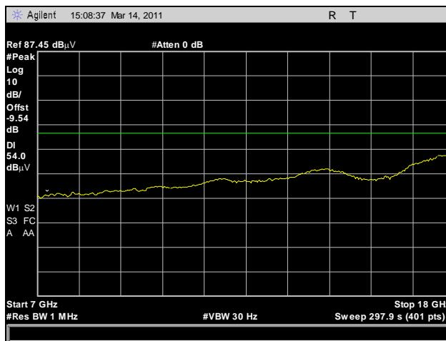
Plot 207. Radiated Harmonics, Mid Channel, 7 GHz – 18 GHz, Average, 802.11n HT10
