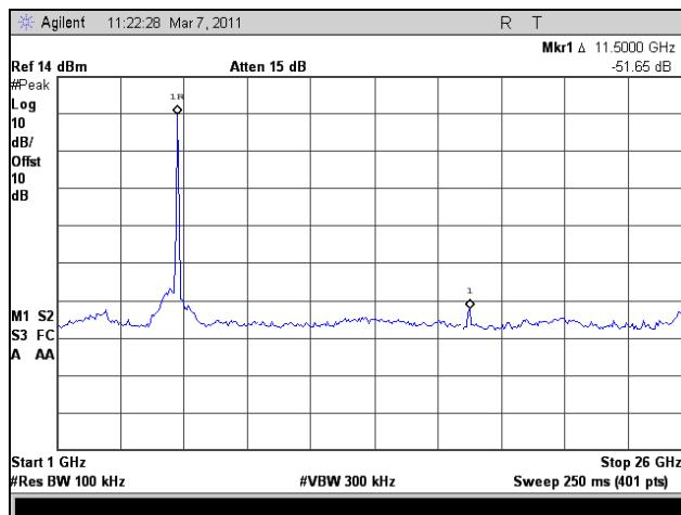
Plot 314. Conducted Spurious Emissions, Low Channel, 1 GHz – 26 GHz, 802.11n HT30, Port 1
