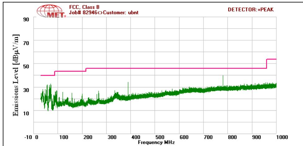
Plot 145. Radiated Spurious Emissions, 802.11a 40 MHz, Low Channel, 30 MHz – 1 GHz
