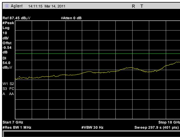
**Plot 227. Radiated Harmonics, High Channel, 7 GHz – 18 GHz, Average, 802.11n HT40**
