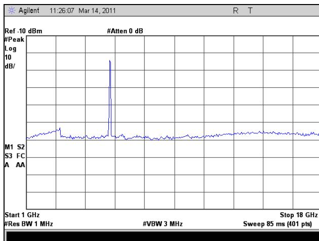
**Plot 184.** Radiated Spurious Emissions, Mid Channel, 1 GHz – 18 GHz, 802.11n HT40
