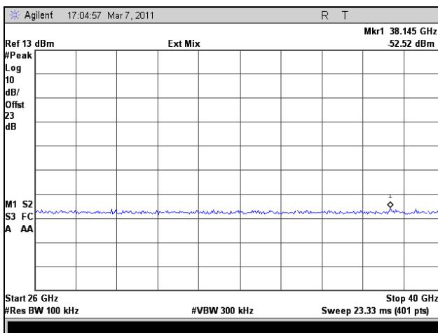
Plot 321. Conducted Spurious Emissions, High Channel, 26 GHz – 40 GHz, 802.11n HT30, Port 1
