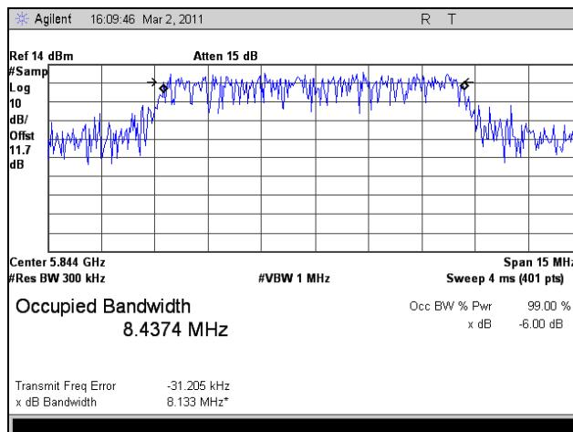
Plot 78. 99% Occupied Bandwidth, High Channel, 802.11n HT10, Port 2
