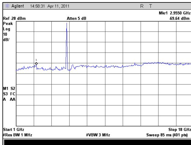
Plot 150. Radiated Spurious Emissions, 802.11a 40 MHz, High Channel, 1 GHz – 18 GHz
