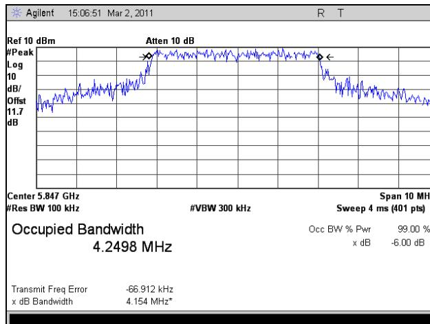
Plot 24. 6 dB Occupied Bandwidth, High Channel, 802.11n HT5, Port 2
