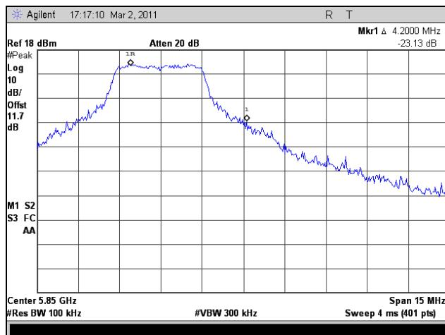
Plot 356. Conducted Band Edge, High Channel, 802.11n HT5, Port 2
