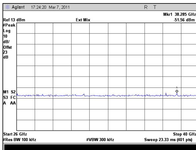
Plot 252. Conducted Spurious Emissions, Low Channel, 26 GHz – 40 GHz, 802.11n HT5, Port 2
