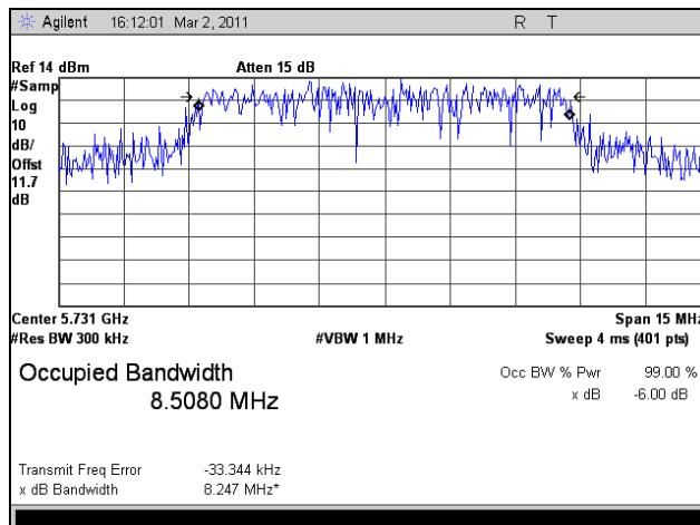
Plot 76. 99% Occupied Bandwidth, Low Channel, 802.11n HT10, Port 2
