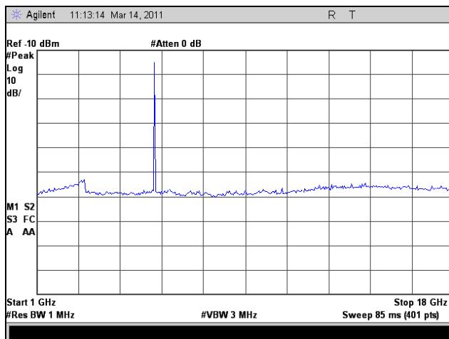
Plot 154. Radiated Spurious Emissions, Mid Channel, 1 GHz – 18 GHz, 802.11n HT5
