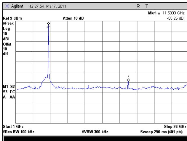
Plot 305. Conducted Spurious Emissions, Low Channel, 1 GHz – 26 GHz, 802.11n HT20, Port 2
