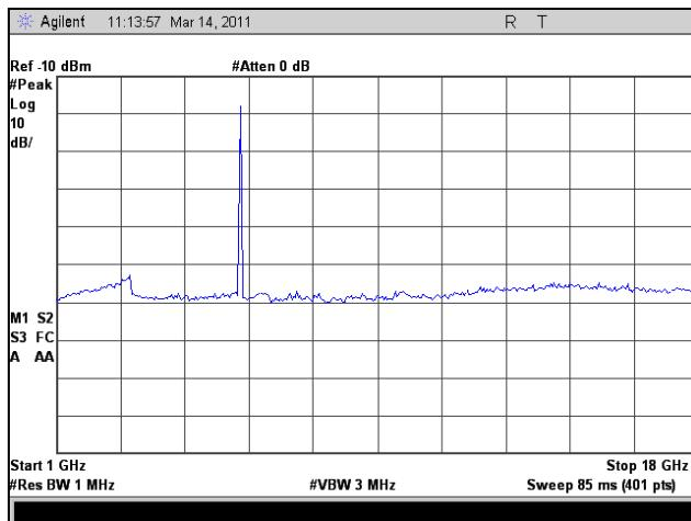
Plot 156. Radiated Spurious Emissions, High Channel, 1 GHz – 18 GHz, 802.11n HT5
