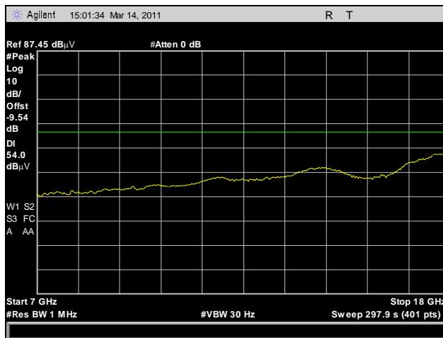
**Plot 209. Radiated Harmonics, High Channel, 7 GHz – 18 GHz, Average, 802.11n HT10**
