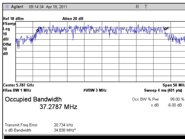
Plot 59. 99% Occupied Bandwidth, 802.11a 40 MHz, Mid Channel
