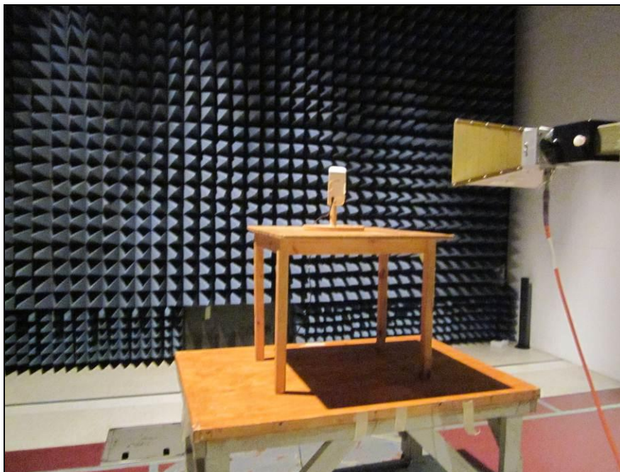
Photograph 3. Radiated Emissions, Test Setup, 1 GHz – 18 GHz
