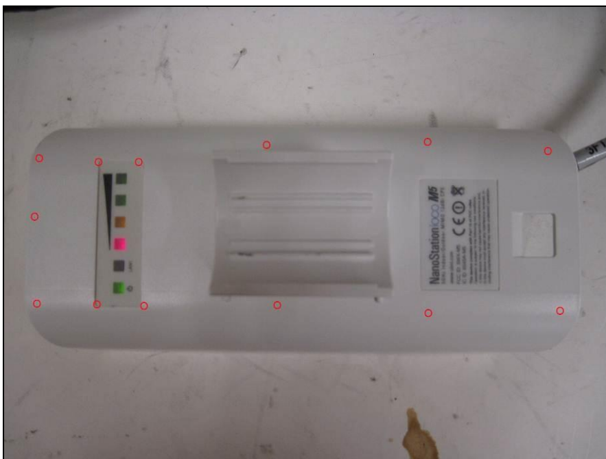
Photograph 8. ESD, Test Points, Rear View, CETUS Power Supply
