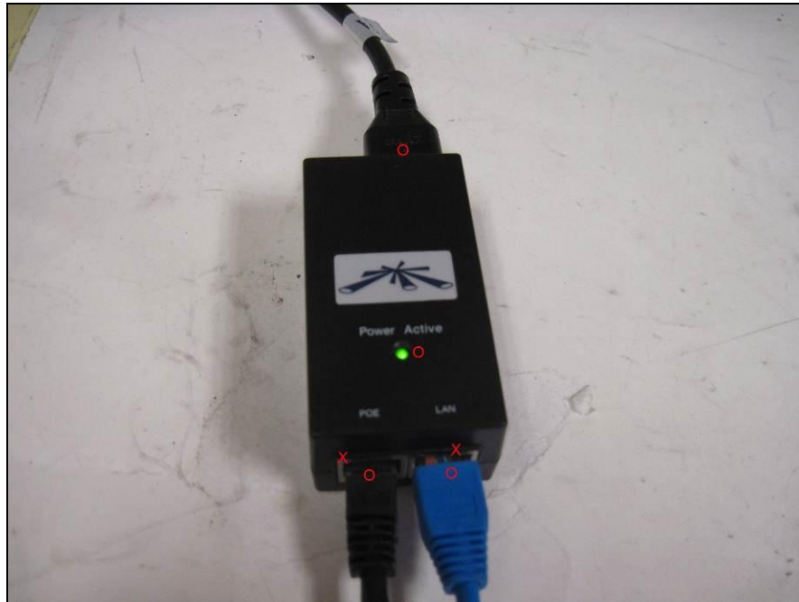
Photograph 12. ESD, Test Points, GME Power Supply
