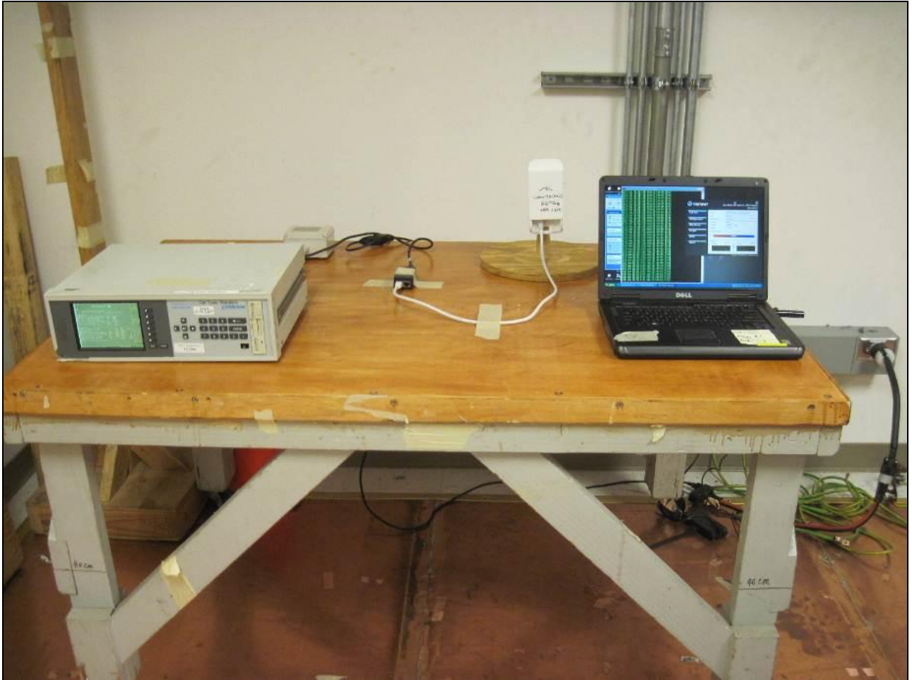
Photograph 2. Harmonic Current Emissions, Test Setup
