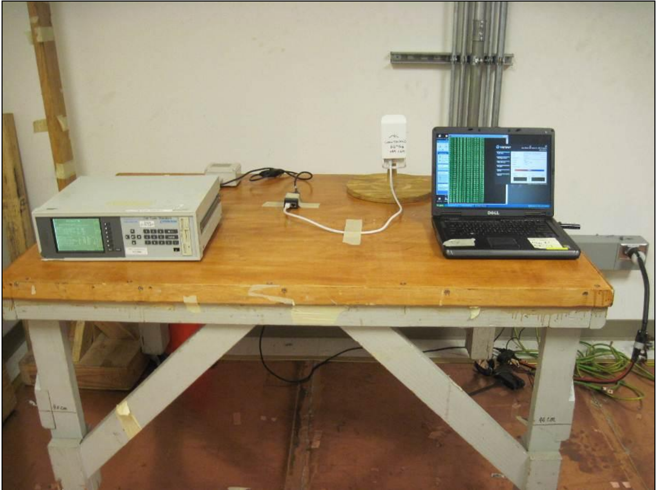
Photograph 3. Voltage Fluctuations (Flicker), Test Setup
