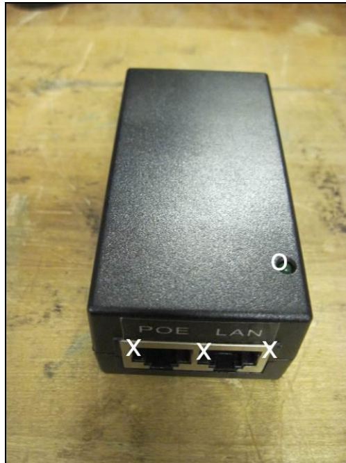
Photograph 9. ESD, Test Points, CETUS Power Supply
