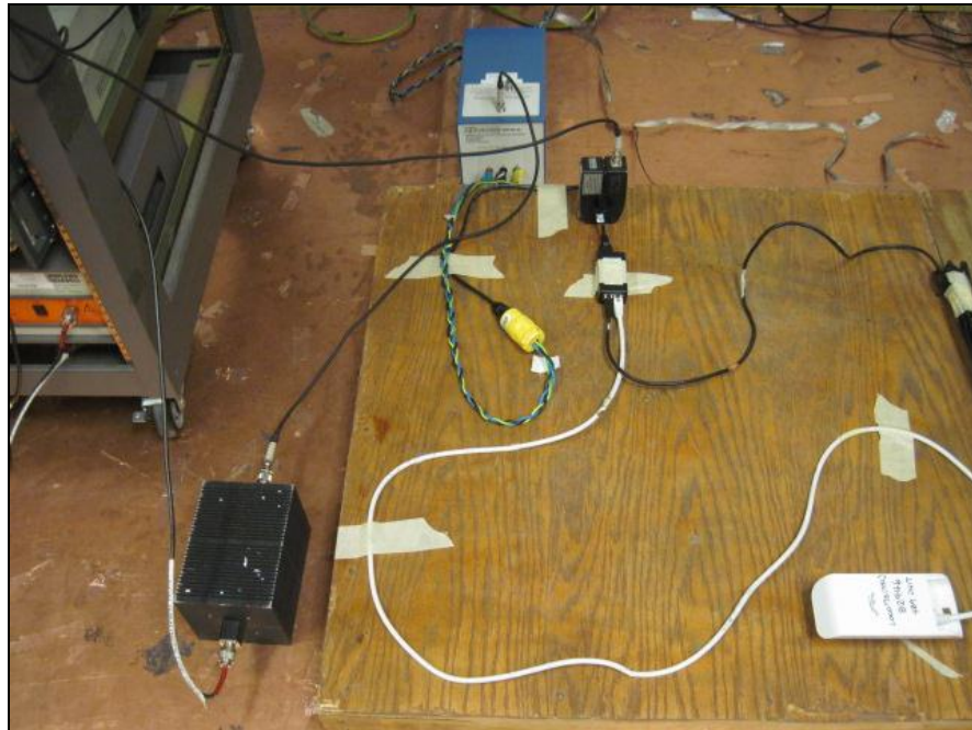
Photograph 16. Radio Frequency, Common Mode, Test Setup, AC Mode
