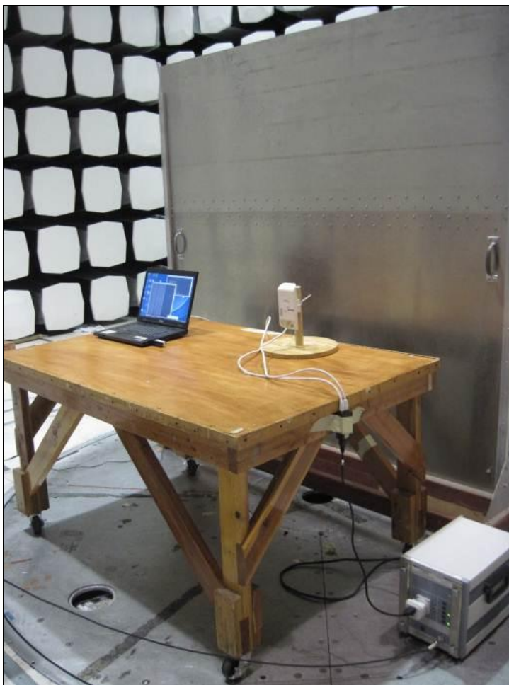
Photograph 1. AC Mains Power Conducted Disturbance, Test Setup
