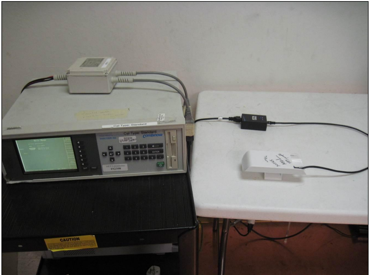
Photograph 3. Harmonic Current Emissions, Test Setup
