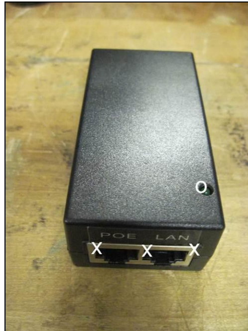
Photograph 10. ESD, Test Points 1
