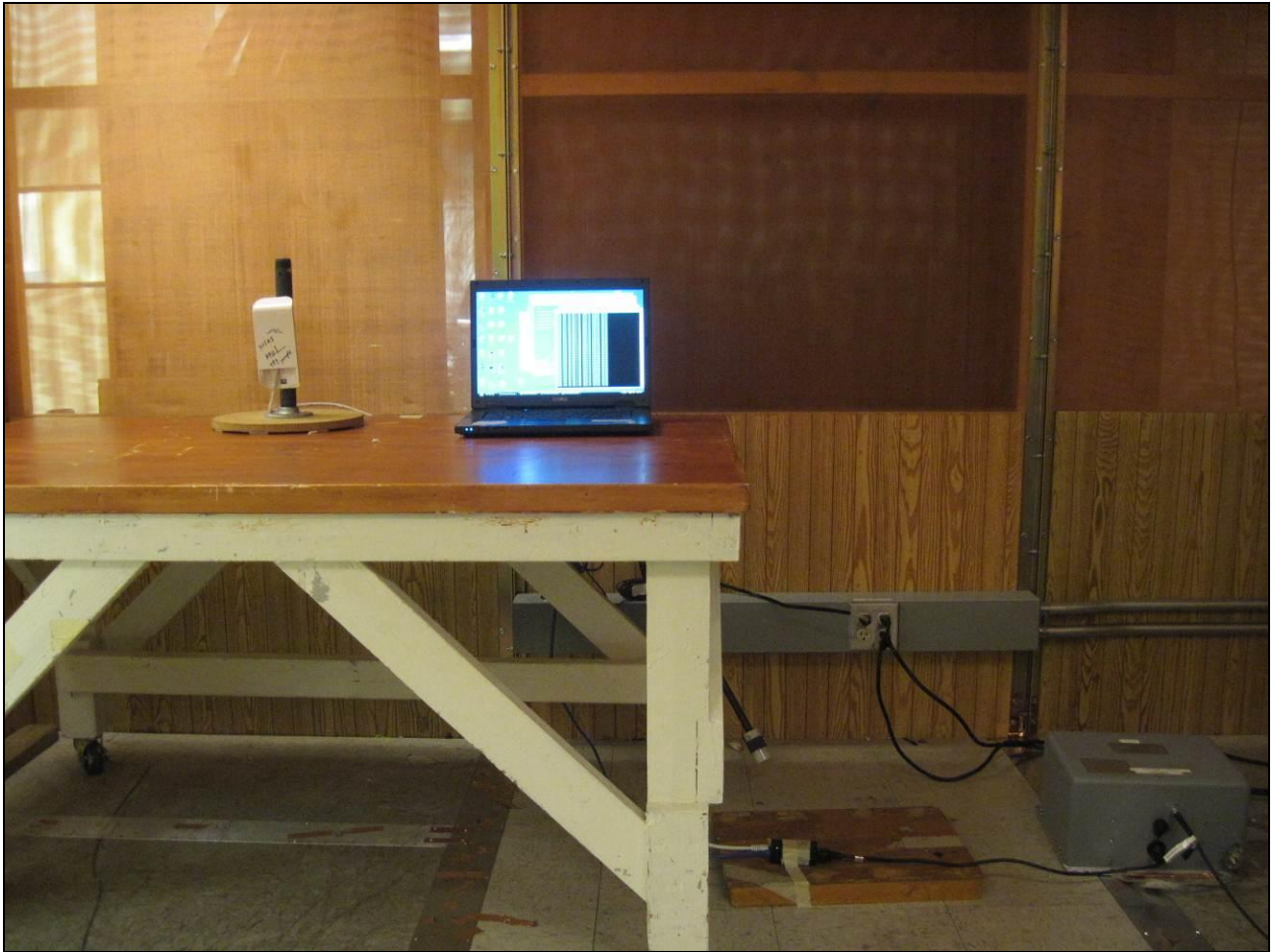
Photograph 2. AC Mains Power Input/Output Ports, Conducted Disturbance, Test Setup
