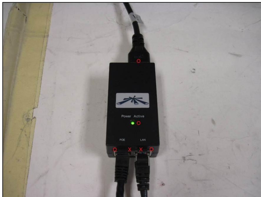
Photograph 11. ESD, Test Points 2
