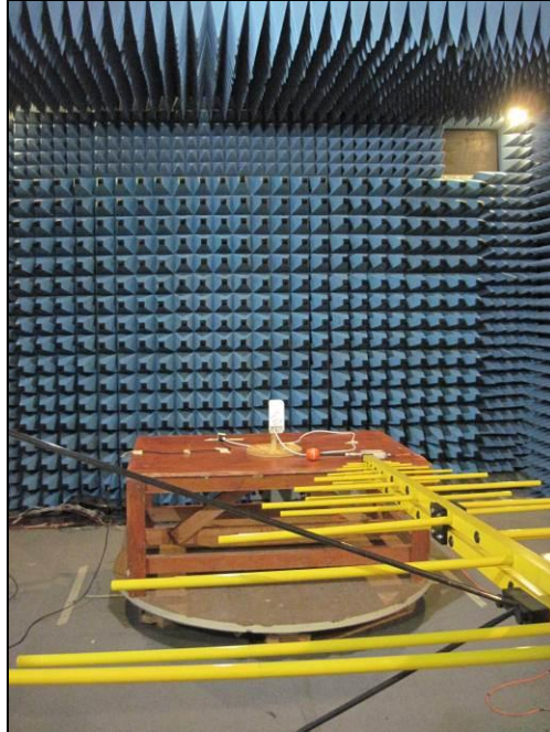
Photograph 6. Radio Frequency Electromagnetic Field, Test Setup, 80 MHz – 1 GHz
