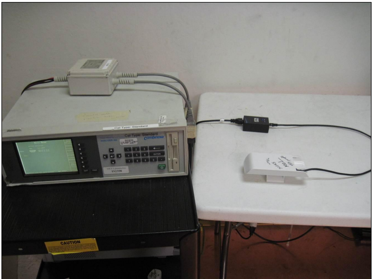
Photograph 4. Voltage Fluctuations (Flicker), Test Setup
