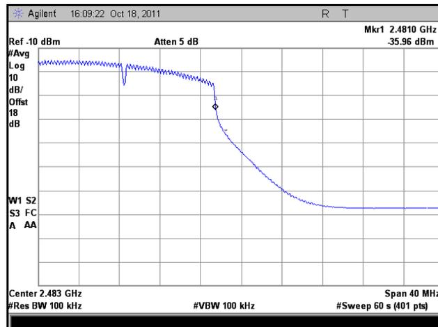
Plot 104. Frequency Range, HT20, High Channel, High Temp., High Voltage
