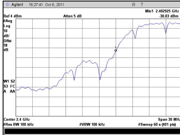
Plot 52. Frequency Range, 802.11b, Low Channel, Low Temp., Low Voltage
