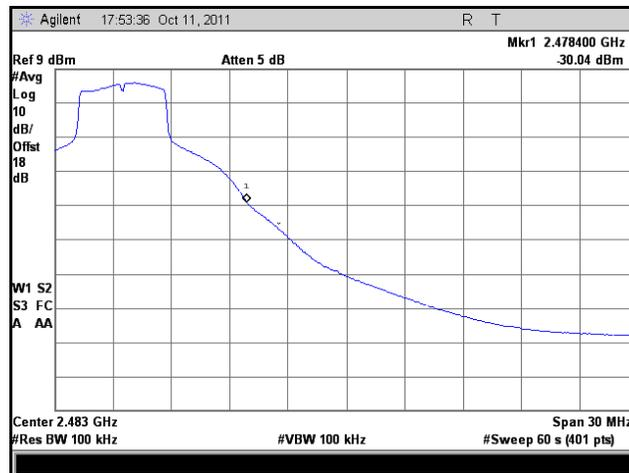
Plot 77. Frequency Range, HT5, High Channel, Low Temp., Low Voltage
