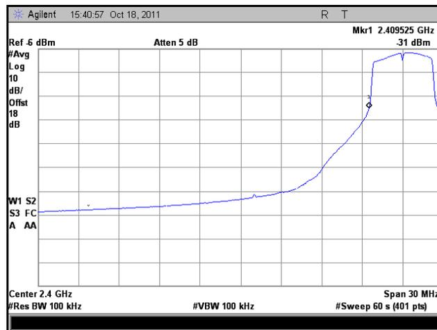
**Plot 70. Frequency Range, HT5, Low Channel, High Temp., Low Voltage**
