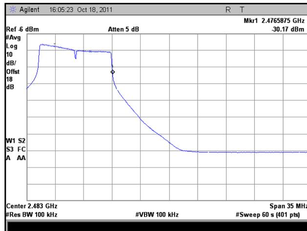
Plot 94. Frequency Range, HT10, High Channel, High Temp., High Voltage
