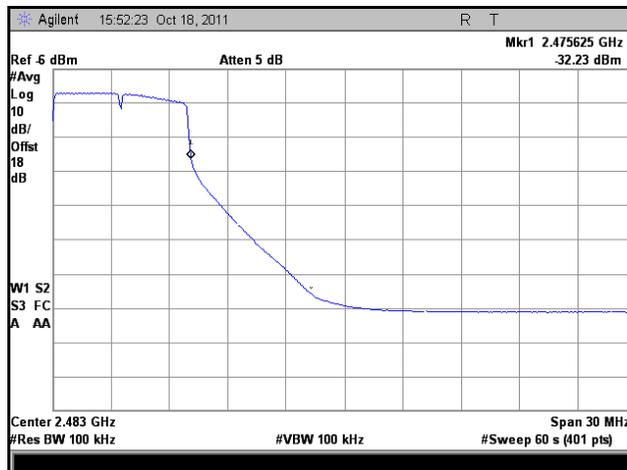
Plot 84. Frequency Range, HT8, High Channel, High Temp., High Voltage
