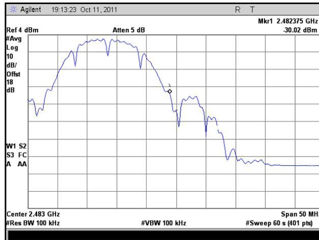
Plot 57. Frequency Range, 802.11b, High Channel, Low Temp., Low Voltage
