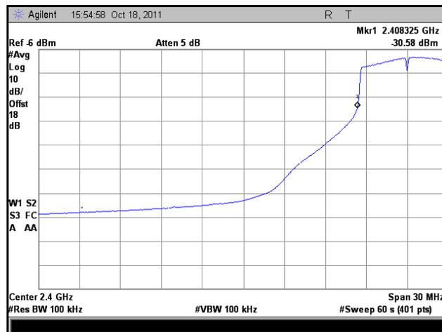
Plot 80. Frequency Range, HT8, Low Channel, High Temp., Low Voltage
