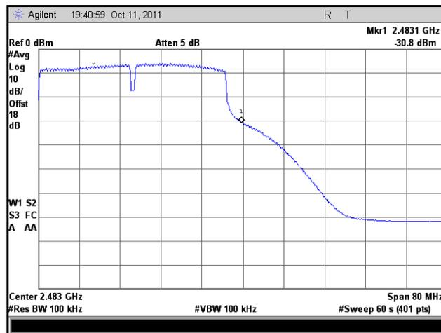
Plot 126. Frequency Range, HT40, High Channel, Low Temp., High Voltage
