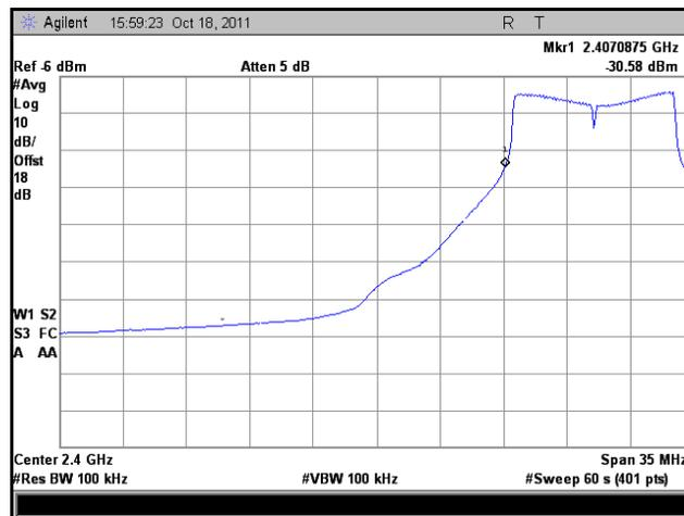
**Plot 90. Frequency Range, HT10, Low Channel, High Temp., Low Voltage**
