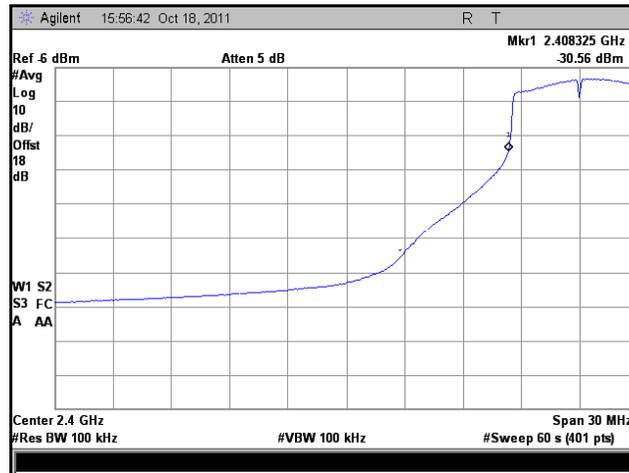
Plot 79. Frequency Range, HT8, Low Channel, High Temp., High Voltage
