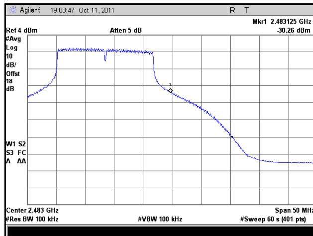
Plot 66. Frequency Range, 802.11g, High Channel, Low Temp., High Voltage
