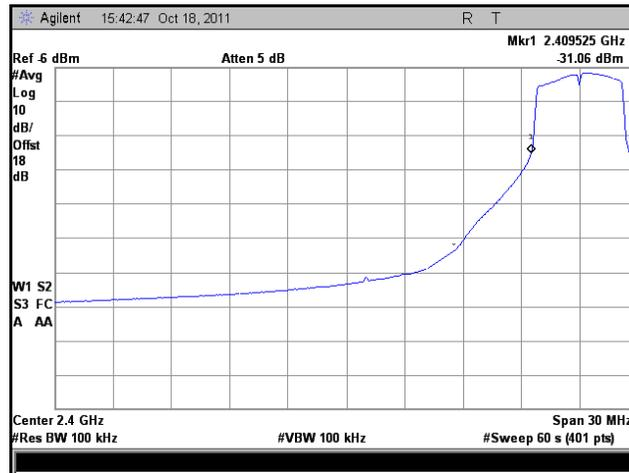
**Plot 69. Frequency Range, HT5, Low Channel, High Temp., High Voltage**
