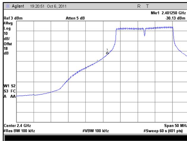
Plot 63. Frequency Range, 802.11g, Low Channel, Room Temp., Nom. Voltage
