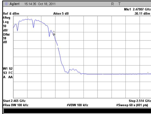
Plot 55. Frequency Range, 802.11b, High Channel, High Temp., Low Voltage
