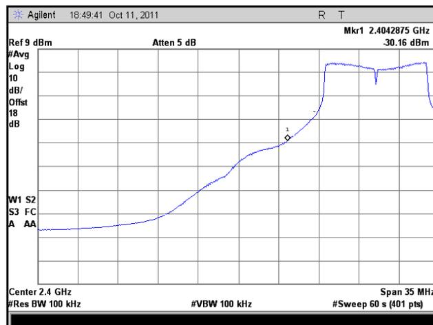
**Plot 91. Frequency Range, HT10, Low Channel, Low Temp., High Voltage**
