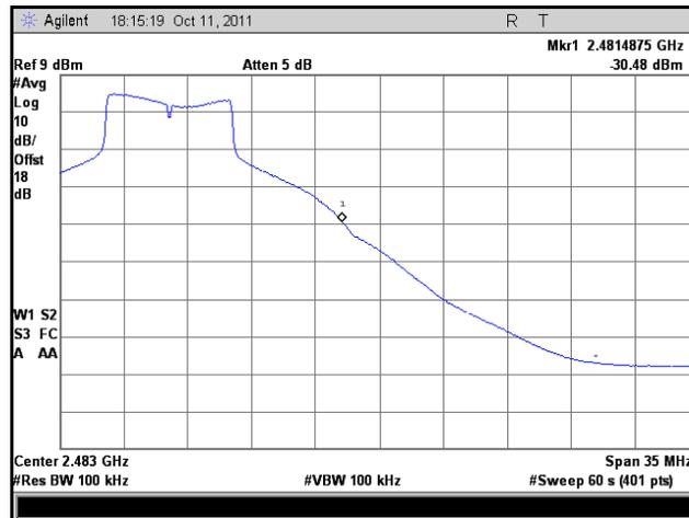
**Plot 86. Frequency Range, HT8, High Channel, Low Temp., High Voltage**
