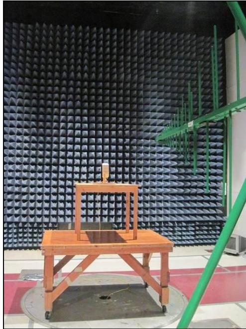
**Photograph 2. Radiated Emissions, Test Setup, 30 MHz – 1 GHz**
