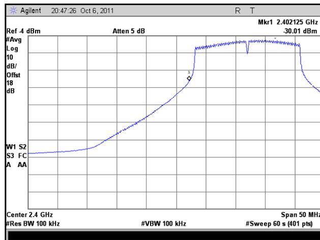
Plot 100. Frequency Range, HT20, Low Channel, High Temp., Low Voltage
