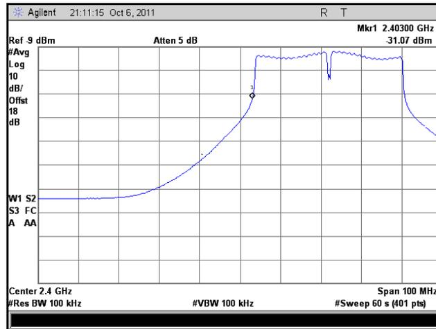
Plot 119. Frequency Range, HT40, Low Channel, High Temp., High Voltage
