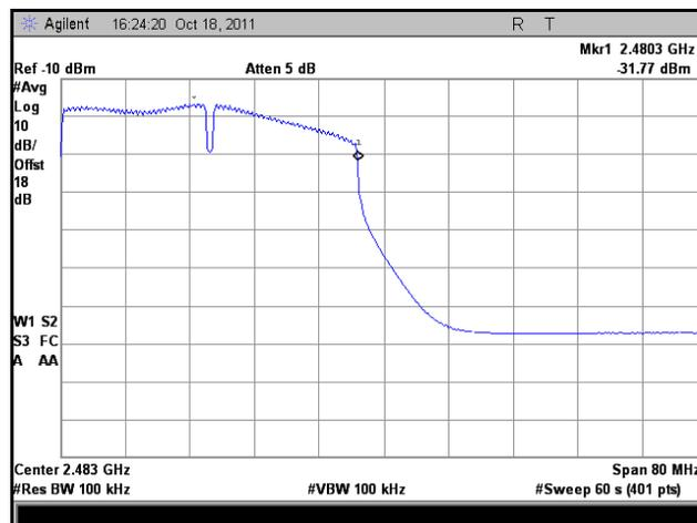
Plot 124. Frequency Range, HT40, High Channel, High Temp., High Voltage
