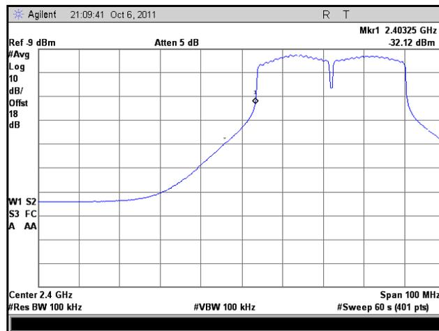
Plot 120. Frequency Range, HT40, Low Channel, High Temp., Low Voltage
