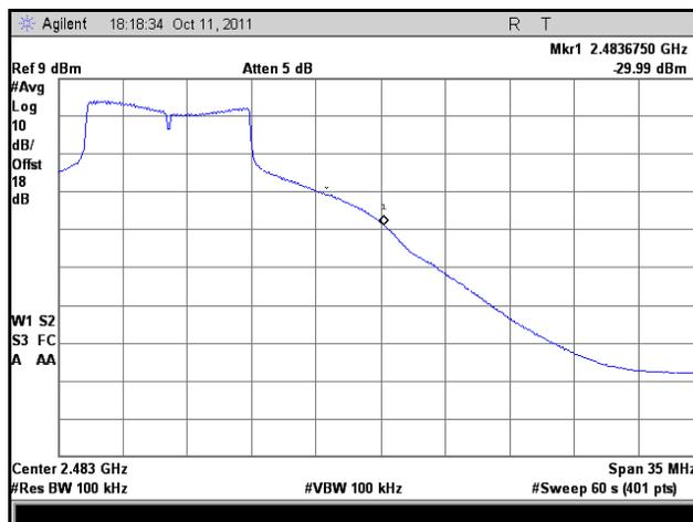
**Plot 97. Frequency Range, HT10, High Channel, Low Temp., Low Voltage**
