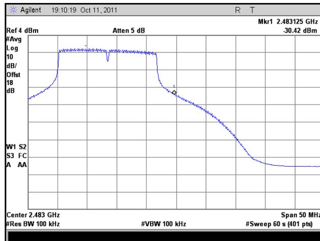
Plot 67. Frequency Range, 802.11g, High Channel, Low Temp., Low Voltage
