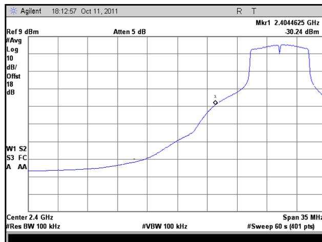
Plot 81. Frequency Range, HT8, Low Channel, Low Temp., High Voltage
