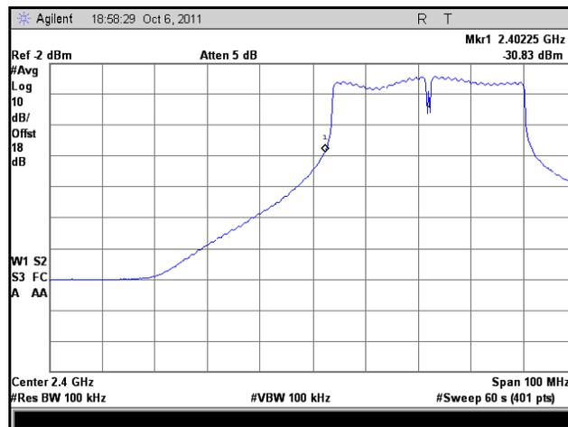
Plot 123. Frequency Range, HT40, Low Channel, Room Temp., Nom. Voltage
