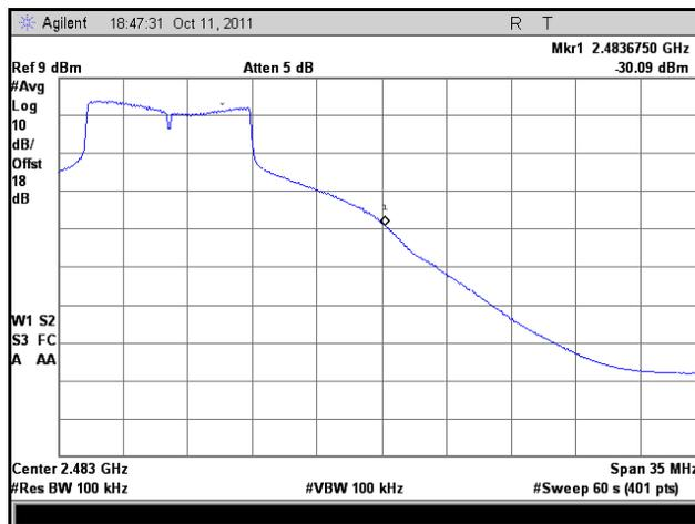
**Plot 96. Frequency Range, HT10, High Channel, Low Temp., High Voltage**
