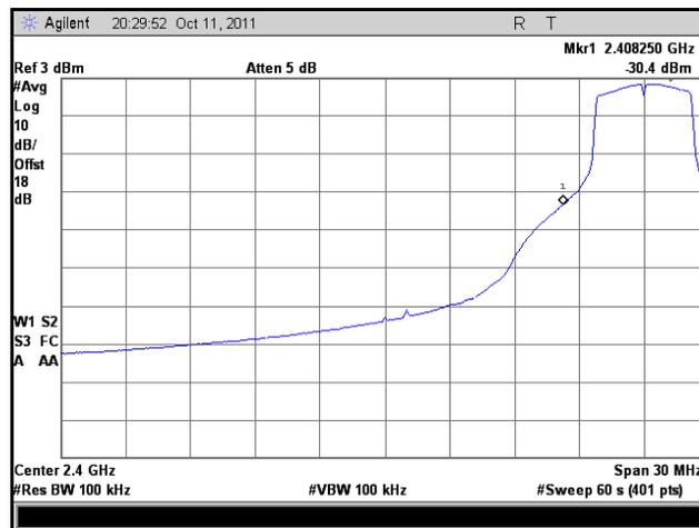
Plot 73. Frequency Range, HT5, Low Channel, Room Temp., Nom. Voltage
