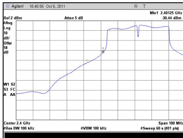
Plot 121. Frequency Range, HT40, Low Channel, Low Temp., High Voltage
