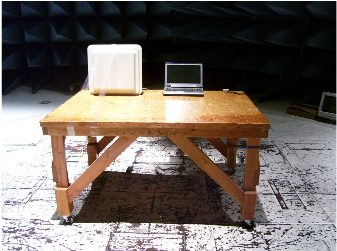
Photograph 4. Radiated Emission Limits Test Setup
