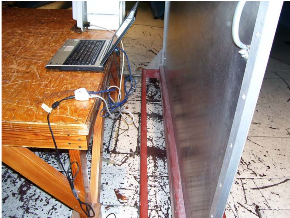
Photograph 3. Conducted Emissions Test Setup, Side View
