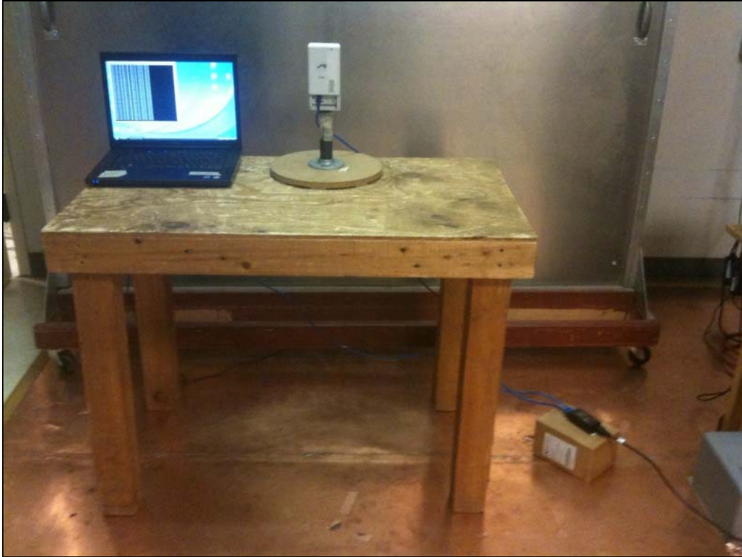
Photograph 5. Conducted Emissions, 15.207(a), Test Setup
