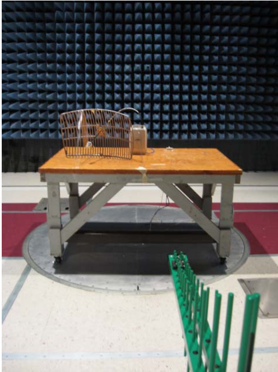
Photograph 3. Radiated Emission Test Setup 30 MHz - 1 GHz
