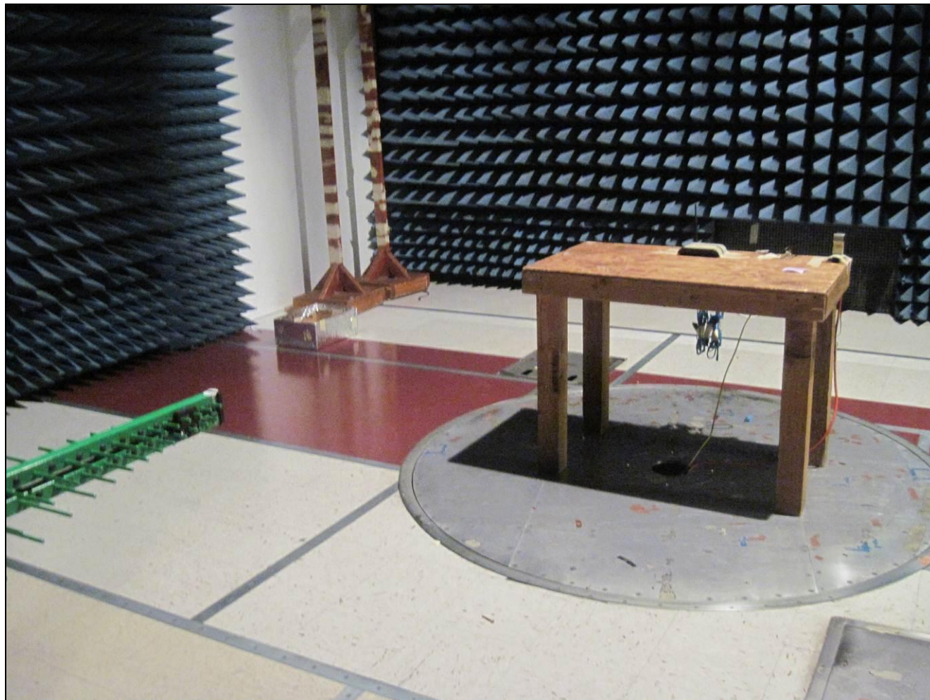
Photograph 3. Radiated Emission, Test Setup, 30 MHz – 1 GHz
