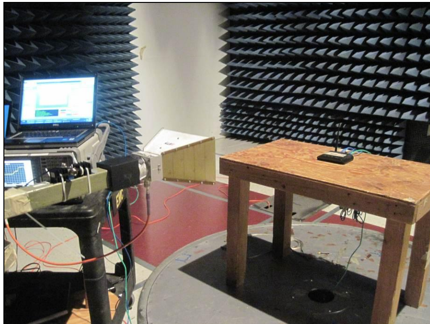
Photograph 6. Radiated Spurious Emissions, Test Setup, 1 GHz – 18 GHz
