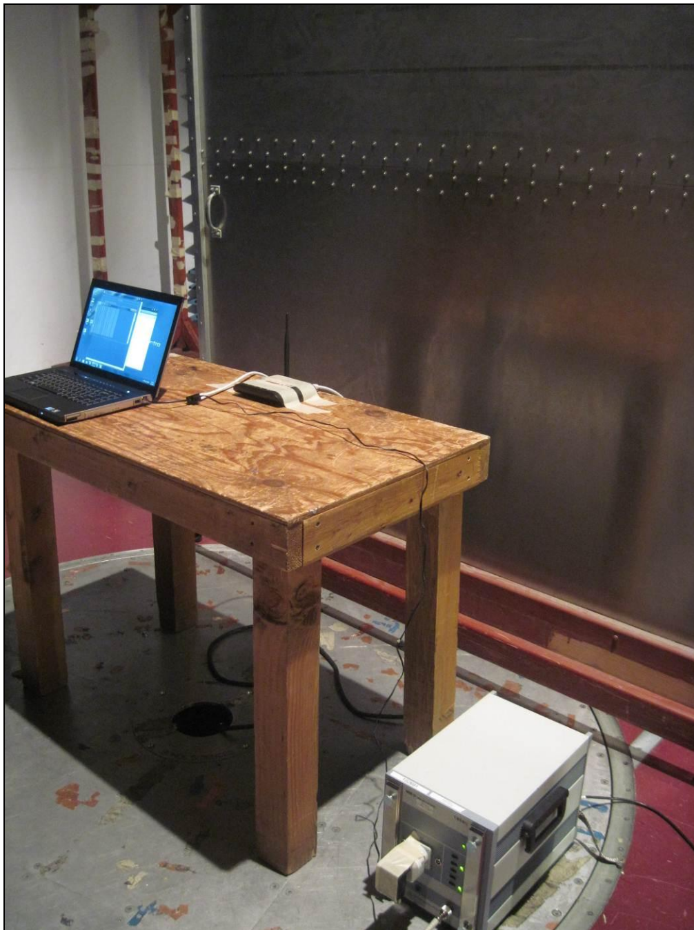
Photograph 2. Conducted Emissions, Test Setup
