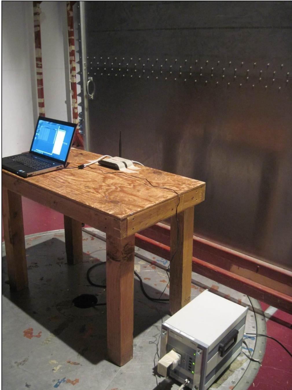
Photograph 4. Conducted Emissions, 15.207(a), Test Setup
