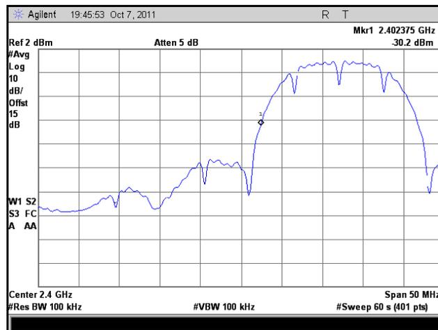
Plot 29. Frequency Range, 802.11b, Low Channel, High Temperature, High Voltage
