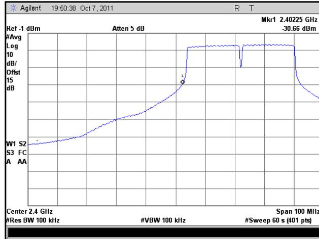
Plot 58. Frequency Range, 802.11n 40 MHz, Low Channel, High Temperature, Low Voltage
