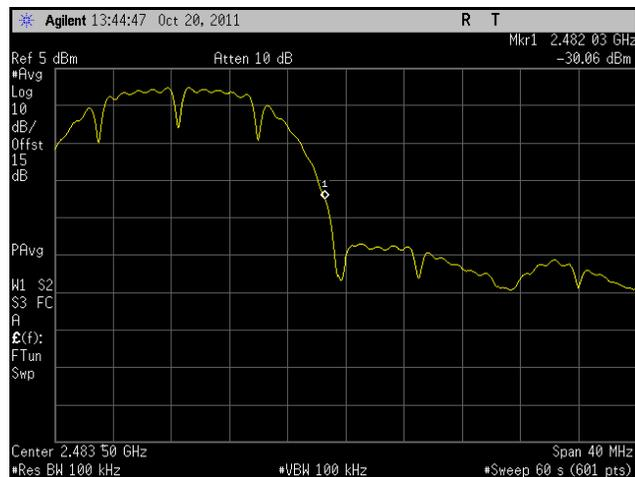
Plot 30. Frequency Range, 802.11b, High Channel, Low Temperature, Low Voltage
