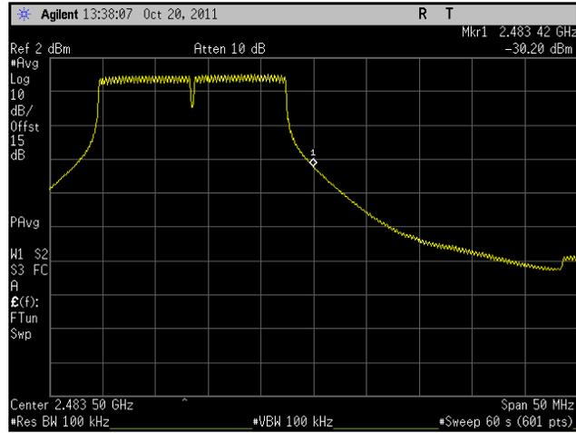
Plot 51. Frequency Range, 802.11n 20 MHz, High Channel, Low Temperature, High Voltage
