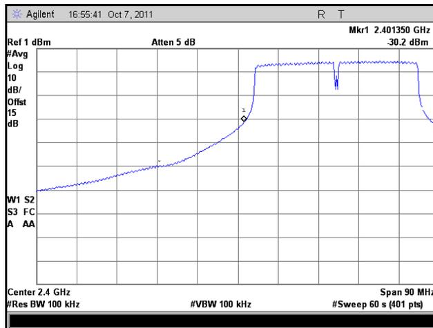
Plot 56. Frequency Range, 802.11n 40 MHz, Low Channel, Low Temperature, High Voltage
