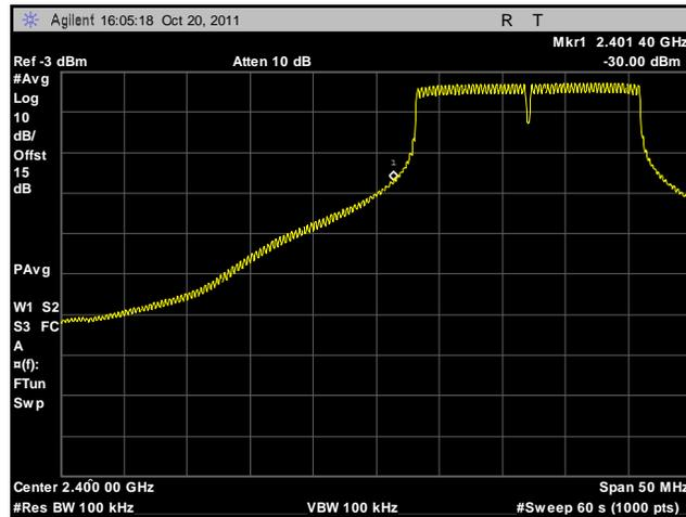
Plot 48. Frequency Range, 802.11n 20 MHz, Low Channel, High Temperature, Low Voltage
