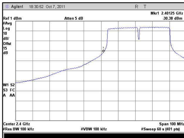
Plot 57. Frequency Range, 802.11n 40 MHz, Low Channel, Room Temperature, Nominal Voltage
