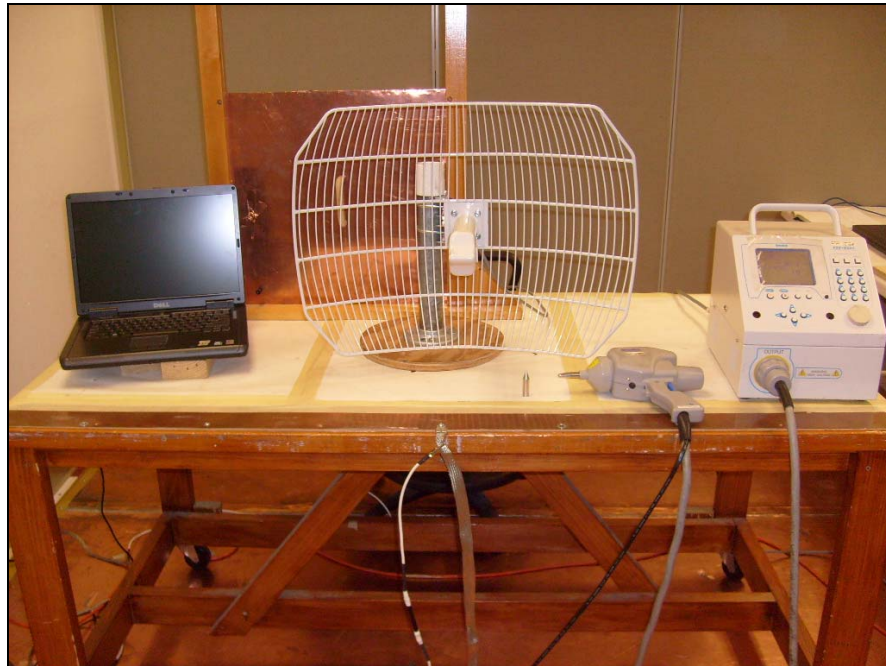
Photograph 16. Electrostatic Discharge, Test Setup, Grid Antenna
