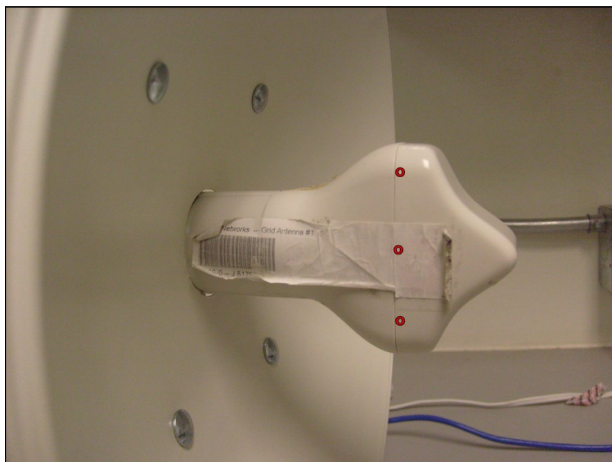
Photograph 15. Electrostatic Discharge, Dish Antenna, Right View
