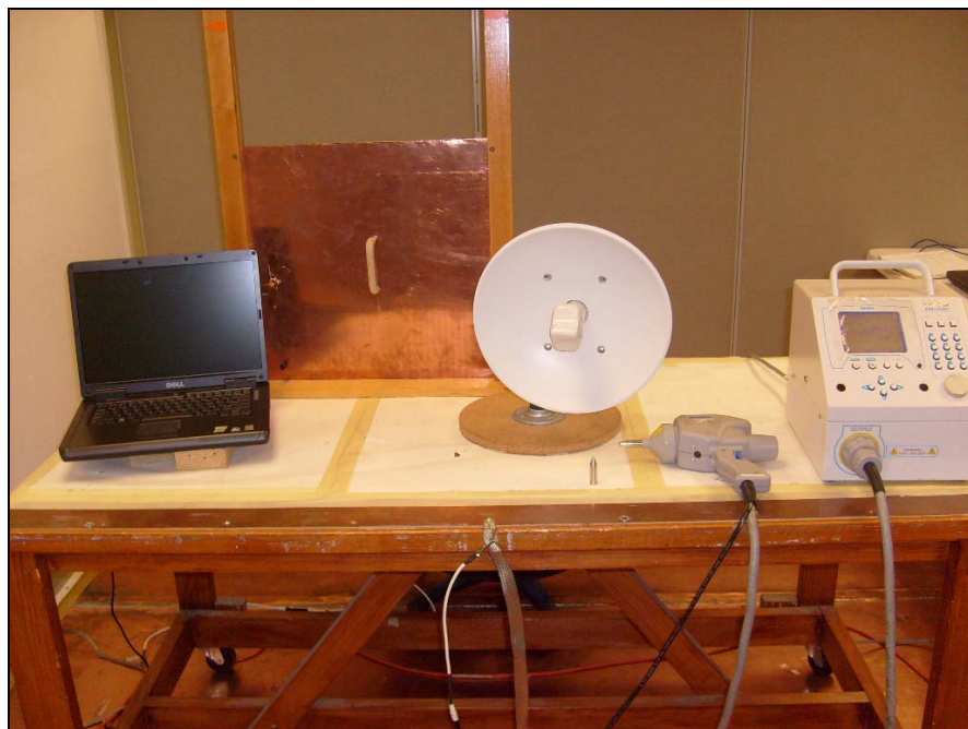
Photograph 17. Electrostatic Discharge, Test Setup, Dish Antenna
